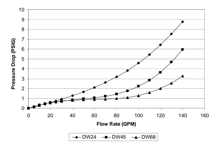
Pressure drops for intermediate flowrates can be calculated using the following formula:
