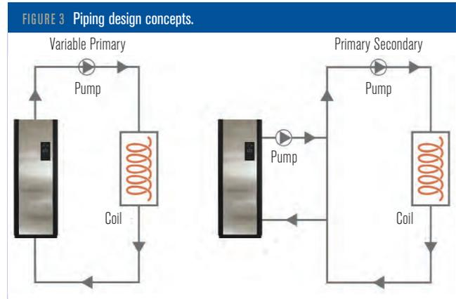
should require half the flow. That in turn, based on the affinity laws, equates to reducing the pump energy use.
