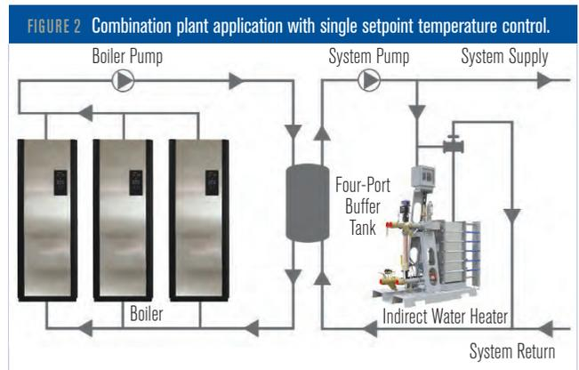
This design adds a layer of security, as well. For example, if the DHW boiler cannot meet its load, the controller will direct the swing valves to divert its designated boilers from space heating to DHW. As per ASHRAE, it is assumed that both space heating and DHW peak loads may not happen concurrently.<sup>3</sup> This offers a major benefit in reducing the number of boilers required to meet plant peak load, shrinking the footprint.
