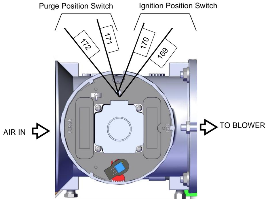
**Figure 5-11a: Air/Fuel Purge and Ignition Locations – BMK750/1000**
