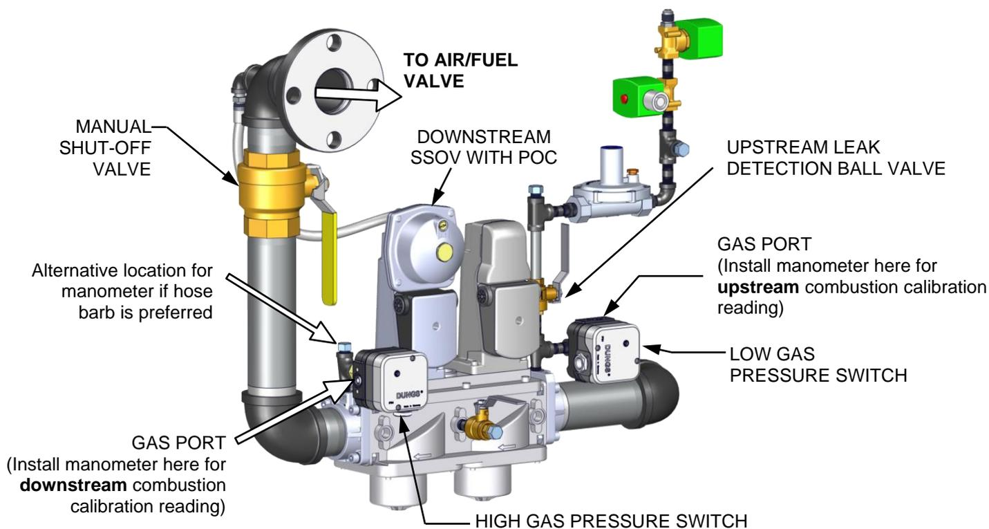
**Figure 4-1f: Port Location for Combustion Calibration – BMK5000-6000**
