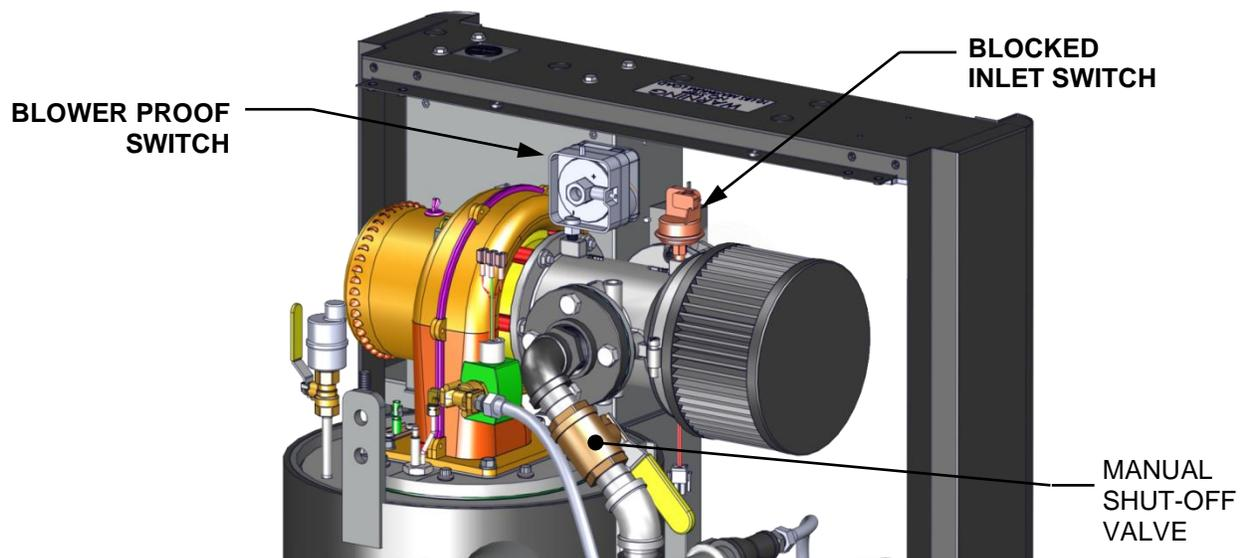
**Figure 5-6b: Blower Proof & Blocked Inlet Switch Locations – BMK750 & 1000**
