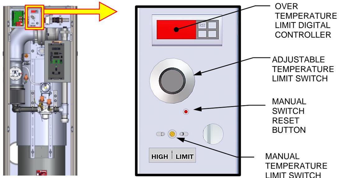
**Figure 5-5b: Temperature Limit Switch Location – BMK1500-3000 Shown**
