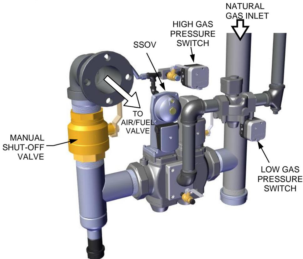
**Figure 3-1d: BMK4000: SSOV Location (P/N 22373-3 shown)**
