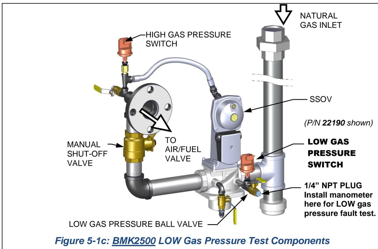
Figure 5-1c: **BMK2500** LOW Gas Pressure Test Components
