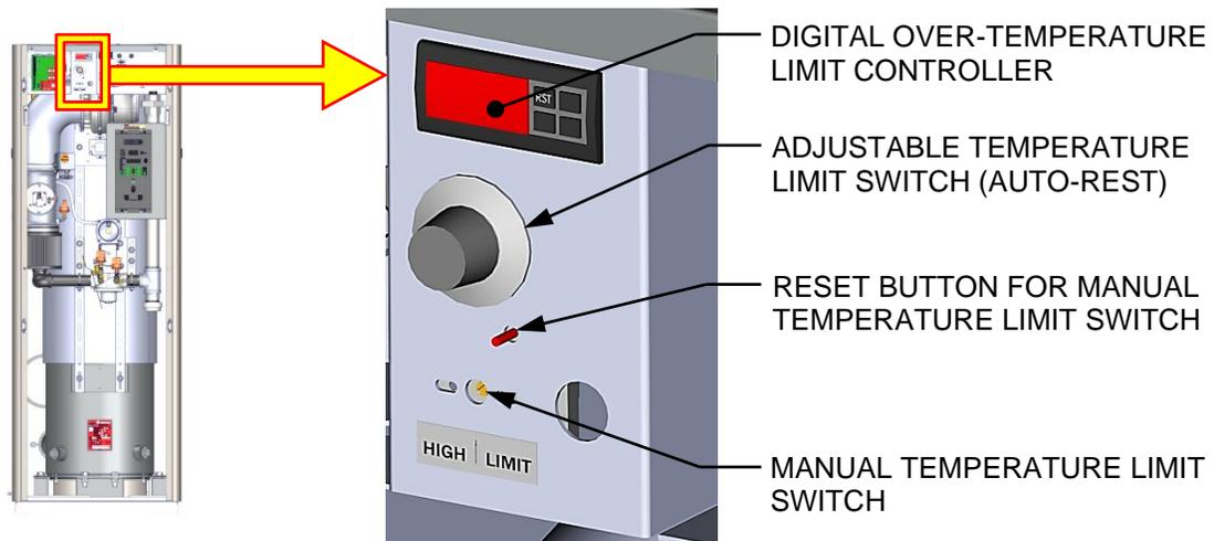
**Figure 4-11b: BMK1500 – 5000N Over-Temperature Limit Switch Location**
