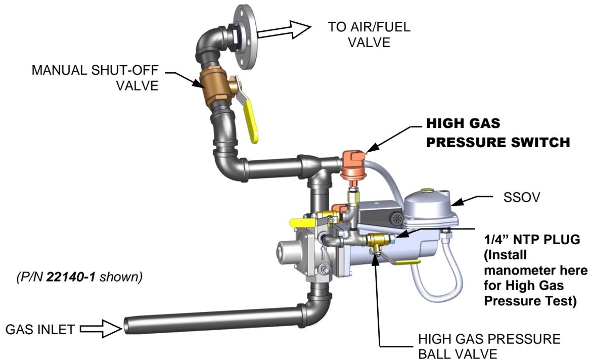
**Figure 5-3a: BMK750/1000 HIGH Gas Pressure Test Components**
