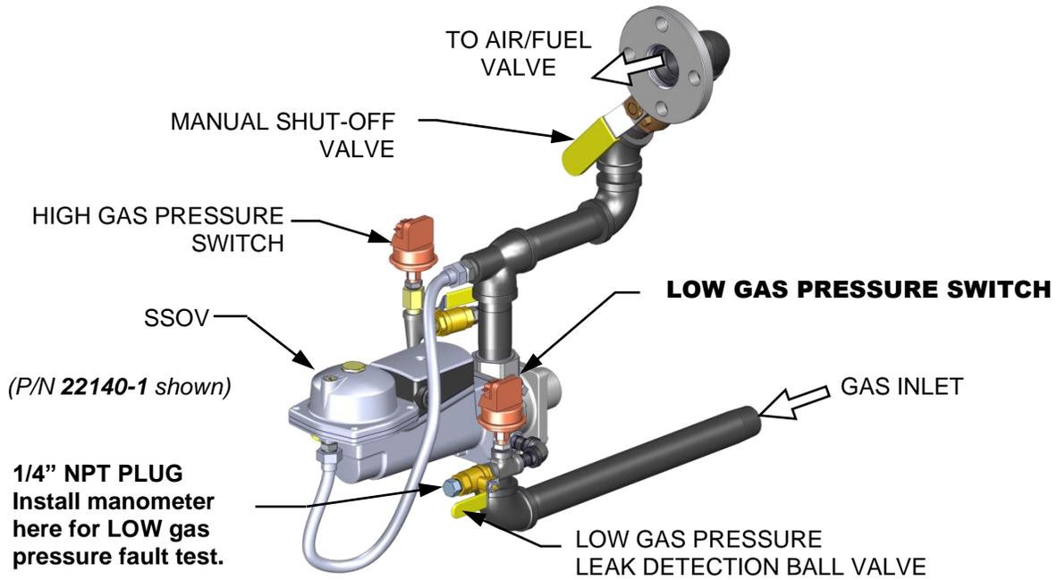
**Figure 5-1a: BMK750/1000 LOW Gas Pressure Test Components**
