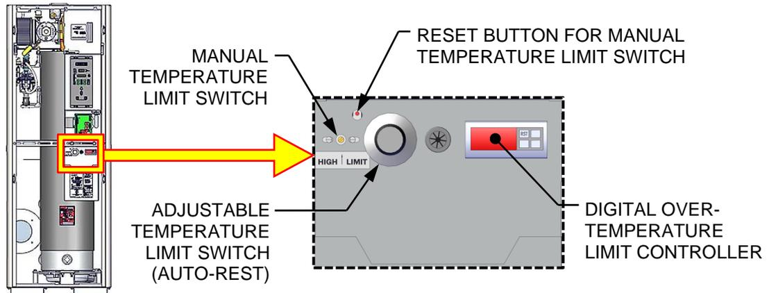
**Figure 4-11a: BMK750 & 1000 Over-Temperature Limit Switch Location**
