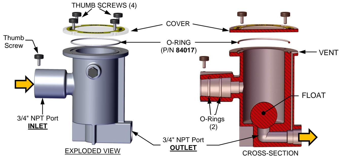
**Figure 8-6: External Condensate Trap – Cross-Section & Exploded View**
