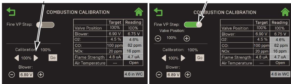
**Figure 4-9: Manual Combustion Calibration Screens**
