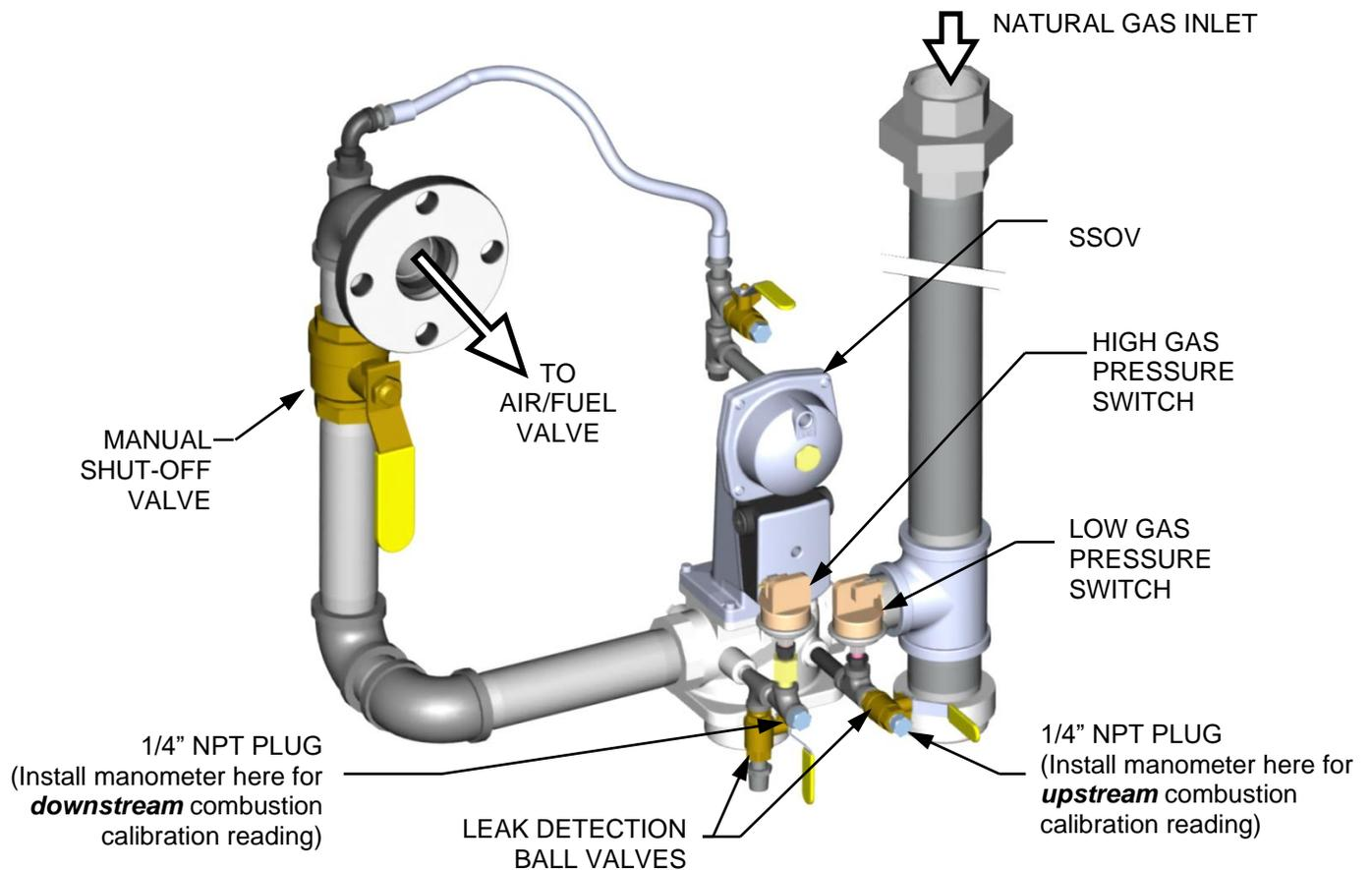
**Figure 4-1b: 1/4 Inch Gas Plug Location – BMK1500 & 2000 (P/N 22314 shown)**
