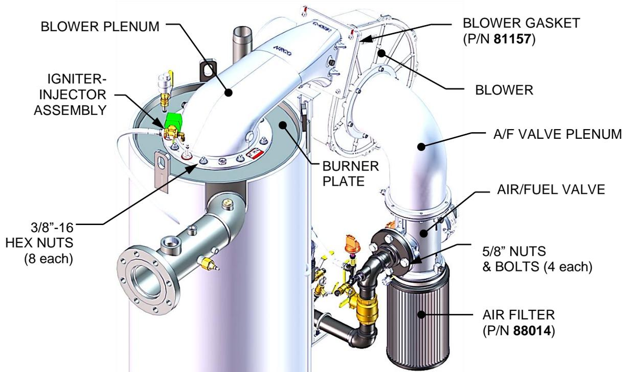
**Figure 8-5c: Burner Assembly Mounting Details – BMK2500 – 5000N**
