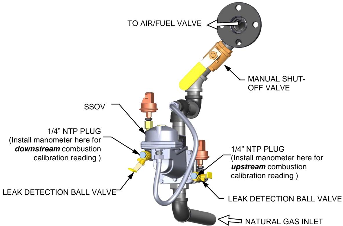
**Figure 4-1a: 1/4 Inch Gas Plug Location – BMK750 & 1000 (P/N 22322 shown)**
