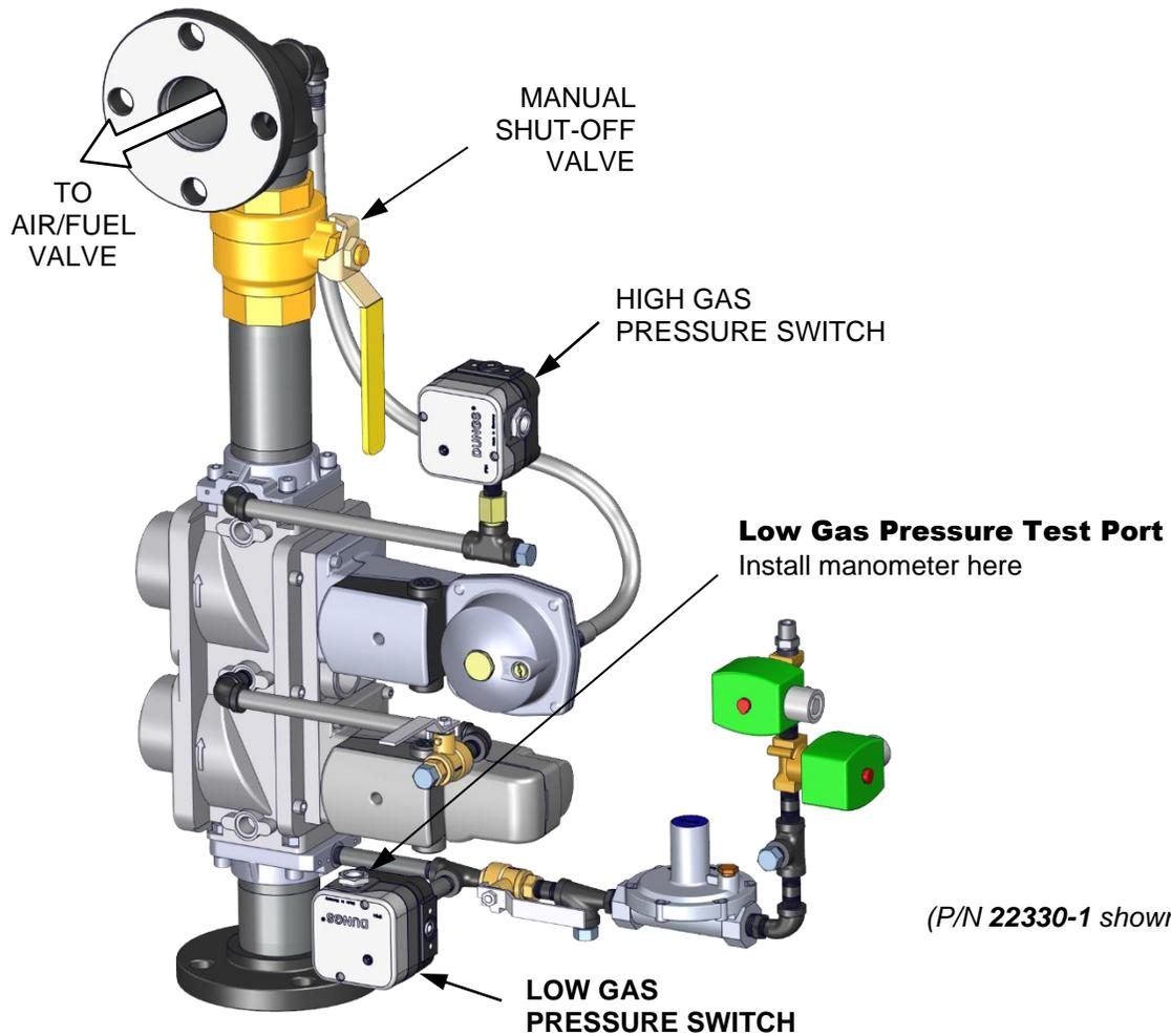
**Figure 5-2c: BMK6000 LOW and HIGH Gas Pressure Test Components**
