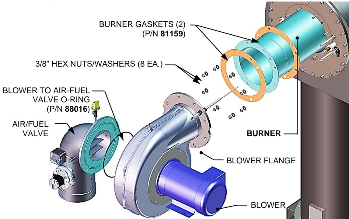
**Figure 8-5d: Burner Assembly Exploded View – BMK5000 & 6000**
