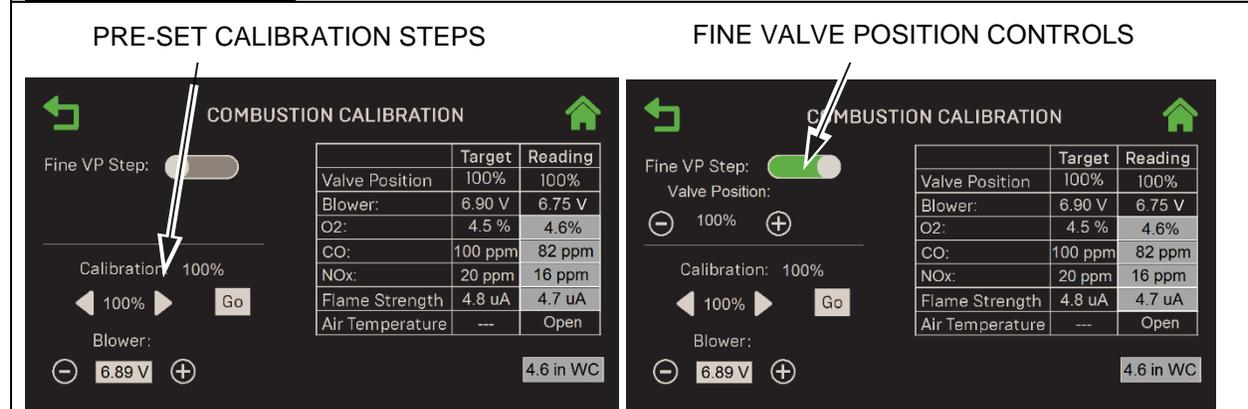
**Figure 4-6: Manual Combustion Calibration Screens**
