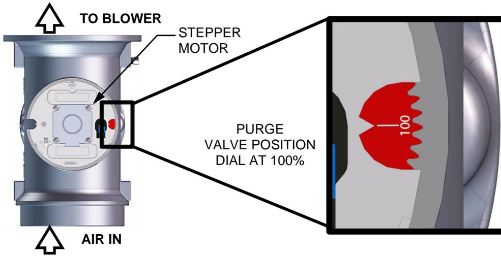
**Figure 3-2b: BMK1500 – 6000 Air/Fuel Valve In Purge Position**
