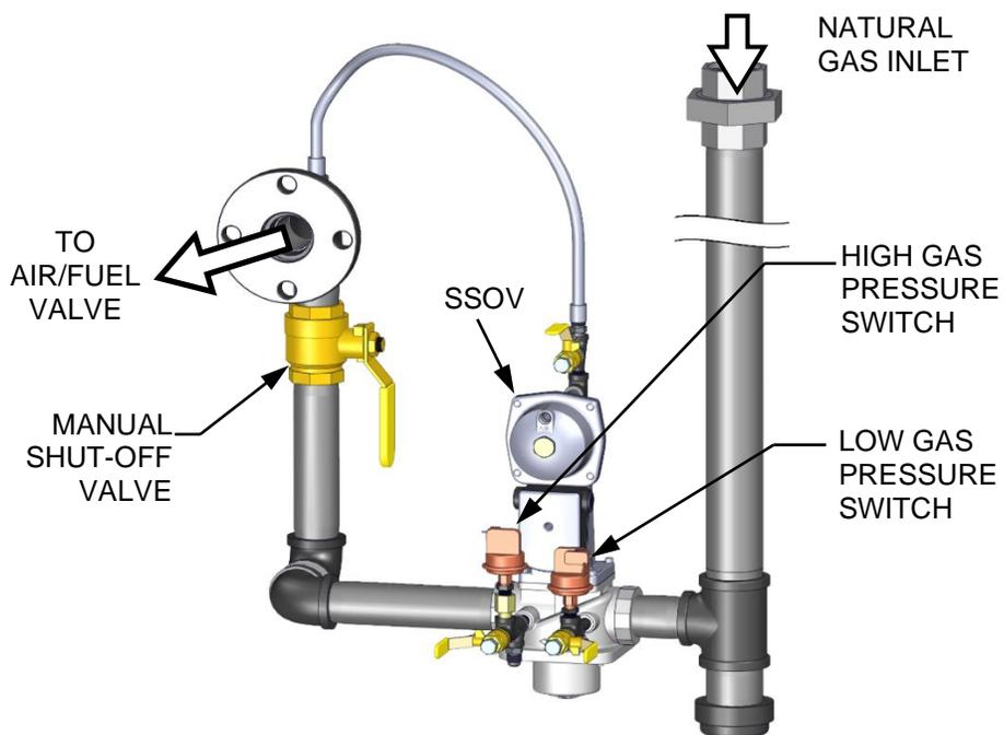
**Figure 3-1b: BMK1500 & 2000 SSOV Location (P/N 22188 shown)**
