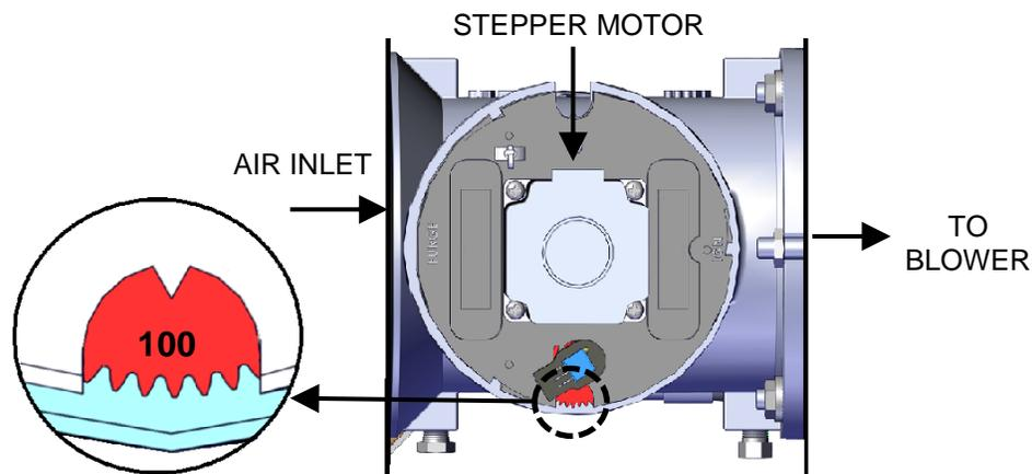
**Figure 3-2a: BMK750 & 1000 Air/Fuel Valve in Purge Position**
