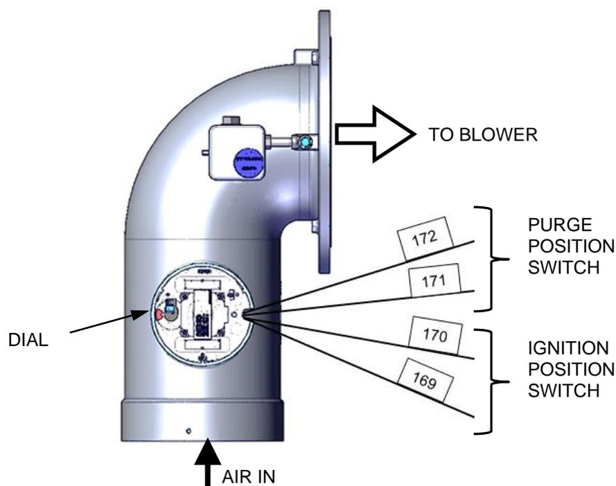
*Figure 5-11c: Air/Fuel Purge and Ignition Locations – BMK5000 & 6000*
