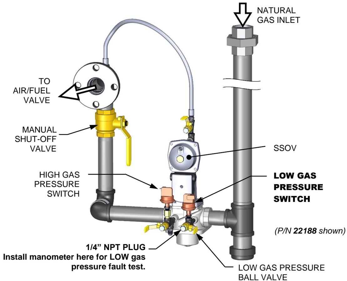
**Figure 5-1b: BMK1500/2000 LOW Gas Pressure Test Components**
