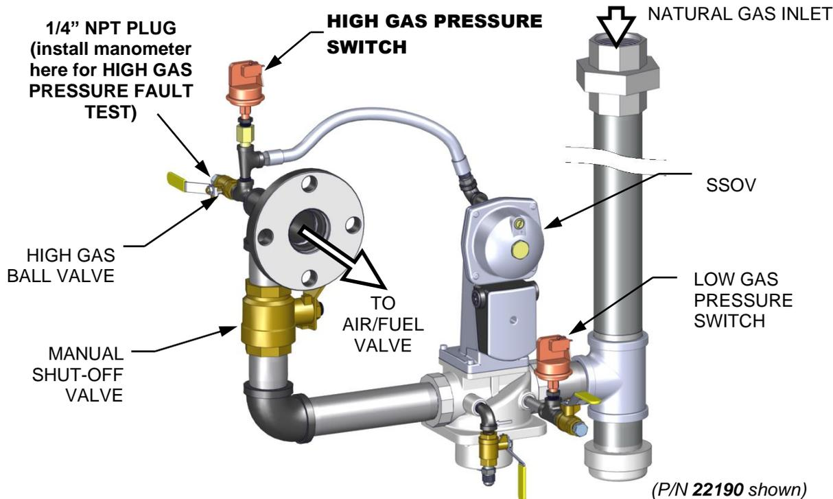
**Figure 5-3c: BMK2500 HIGH Gas Pressure Fault Test**
