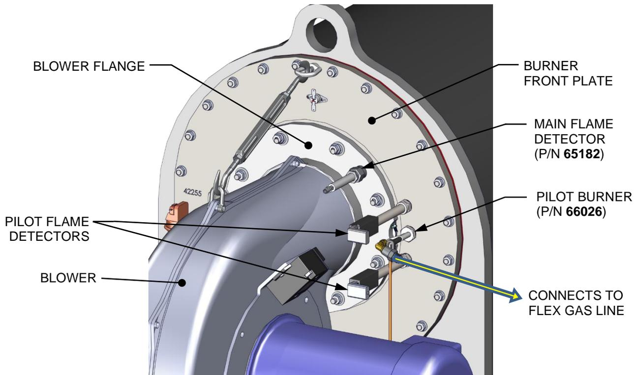
**Figure 8-2: Pilot Burner and Pilot Flame Detectors (BMK5000/6000)**
