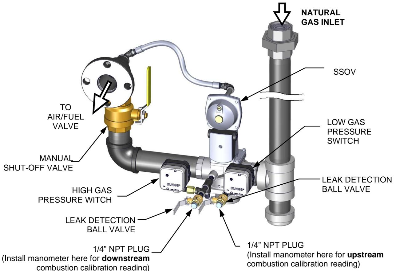
**Figure 4-1d: 1/4 Inch Gas Plug Location – BMK3000 (P/N 22310 shown)**
