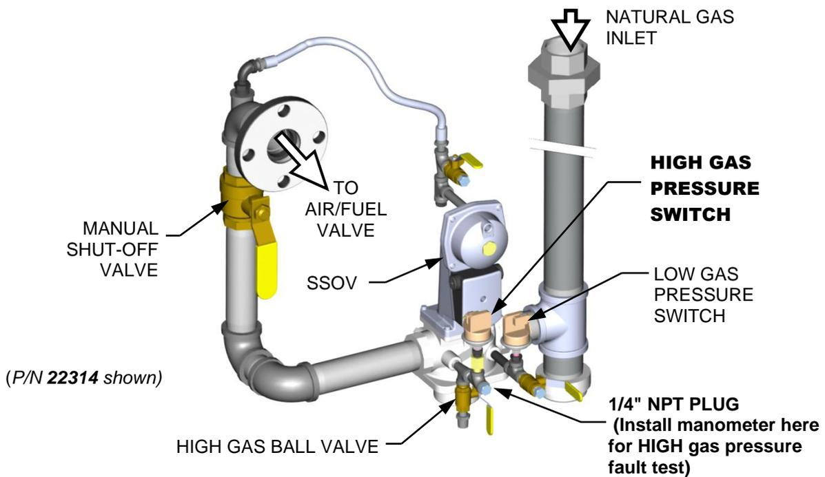
**Figure 5-3b: BMK1500/2000 HIGH Gas Pressure Fault Test**
