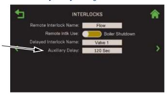
Figure 2-22: Intelocks Screen – Auxiliary Delay Parameter
