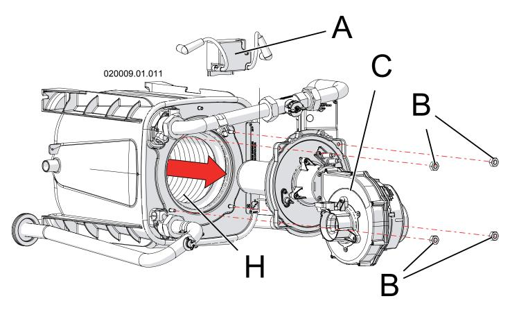
Figure 17-7 Remove the fan burner assembly
