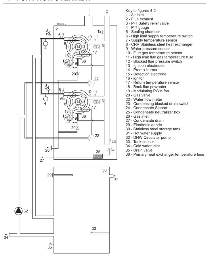
Figure 4-2 - Hydronic functional schematic for models 399 and 500
