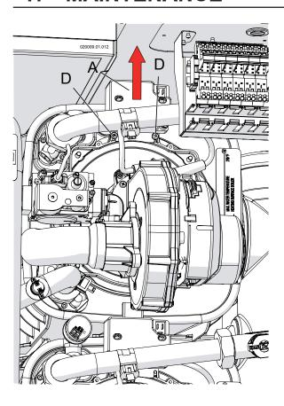
Figure 17-3 Remove the spark generator
