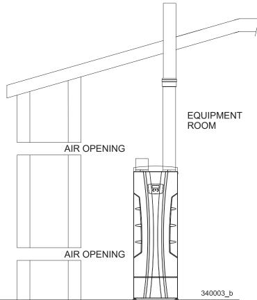
**Figure 5-2 Combustion Air through Ducts**
