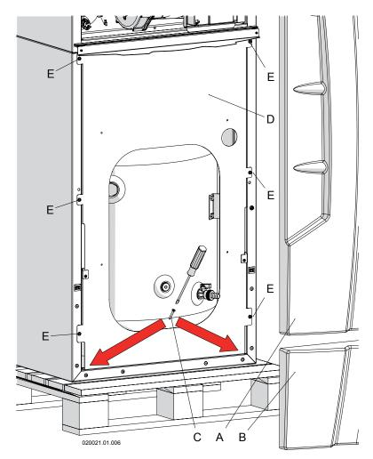
Figure 6-1 Remove heater from wood pallet (front)
