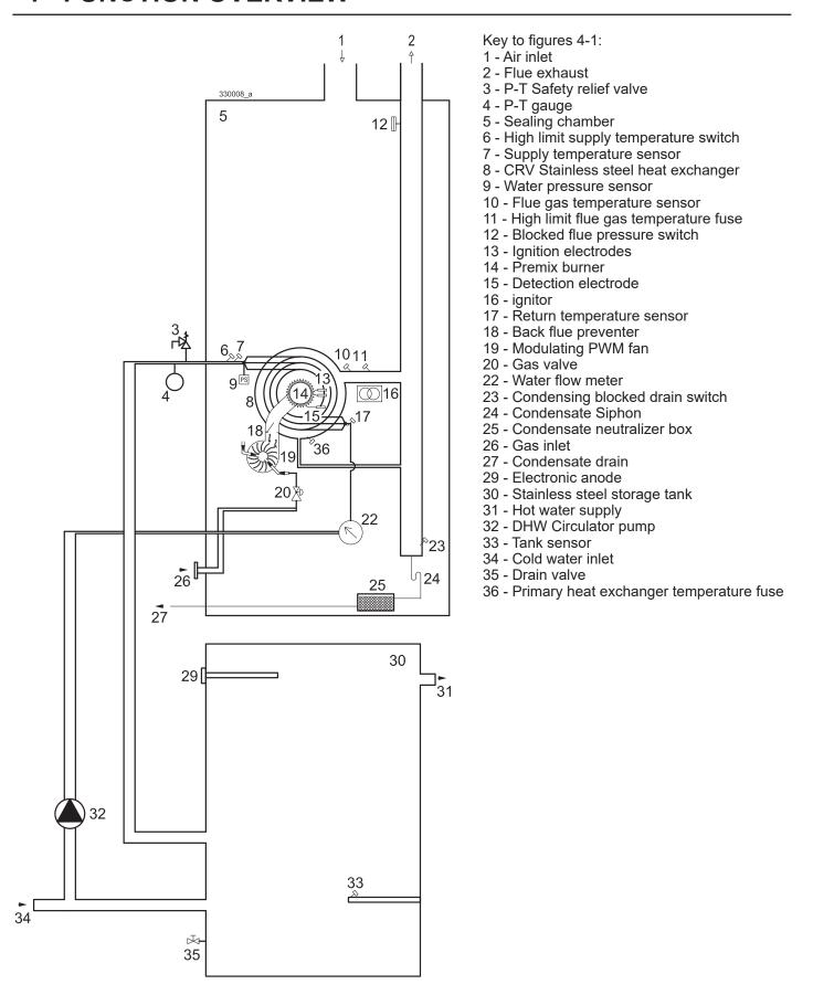
Figure 4-1 - Hydronic functional schematic for models 199 and 250
