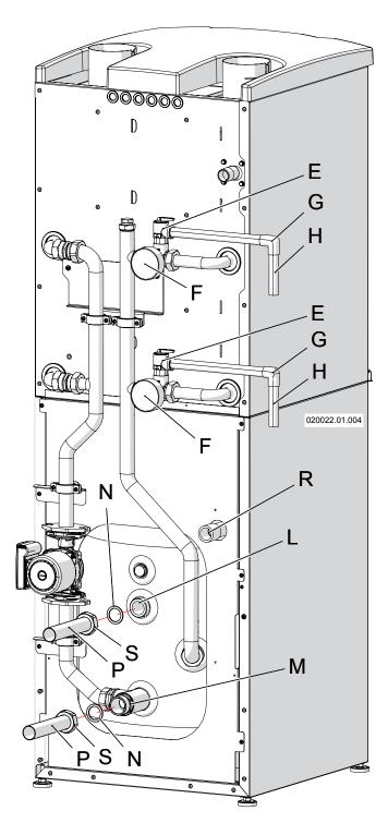
Figure 8-1 Piping of the P-T relief valve discharge and piping the water connections
