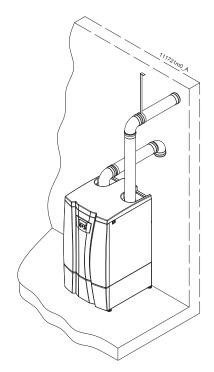
Figure 12-1 Side wall two pipes (Direct venting).
