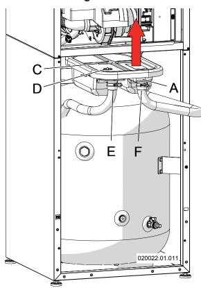
Figure 17-11 Condensate trap and neutralizing box removing
