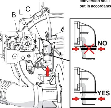
Figure 14-4 Lift the gas valve
