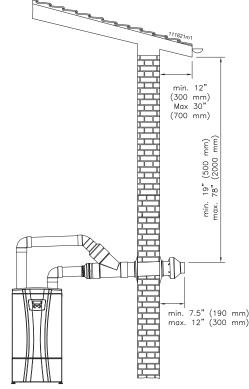
Figure 12-19 Concentric sidewall termination clearances
