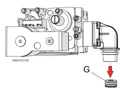
Figure 14-5 Gas orifice
