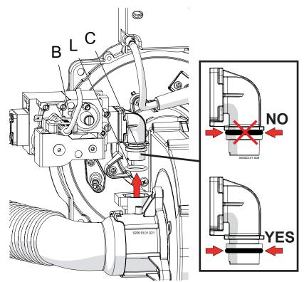
Figure 17-6 Remove the gas valve
