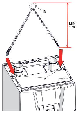
Figure 6-4 Correct way to lift the appliance
