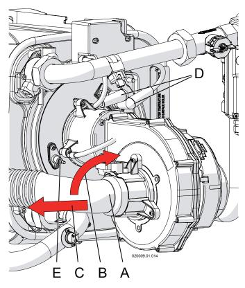
Figure 17-4 Remove the air inlet silencer
