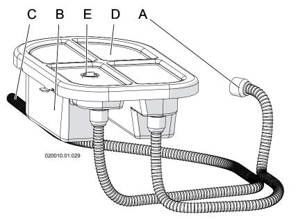
A = Pipe connected to the heaters' flue exhaust system
