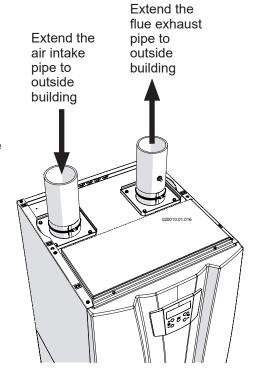
Figure 12-11 Stainless steel air intake/vent connection correctly in place
