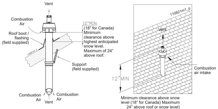
Figure 12-24 Concentric vertical terminations
