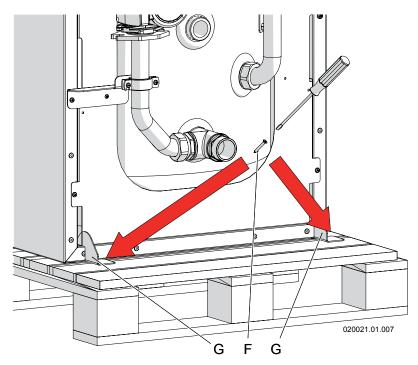
Figure 6-2 Remove heater from wood pallet (back)
