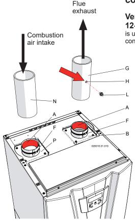
Figure 12-8 PVC/CPVC air intake/ vent connection
