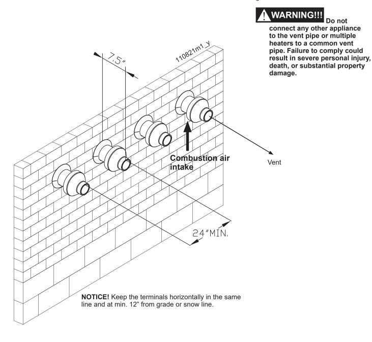
Figure 12-20 Concentric sidewall multiple heaters terminations
