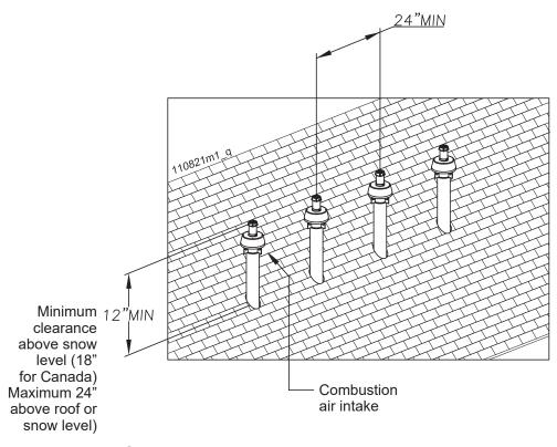
Figure 12-26 Concentric multiple heaters vertical terminations
