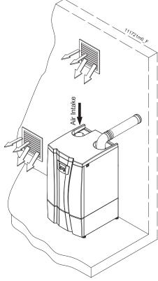
Figure 12-5 Side wall (or vertical in a roof) one pipe venting, combustion air from room (not Direct venting).
