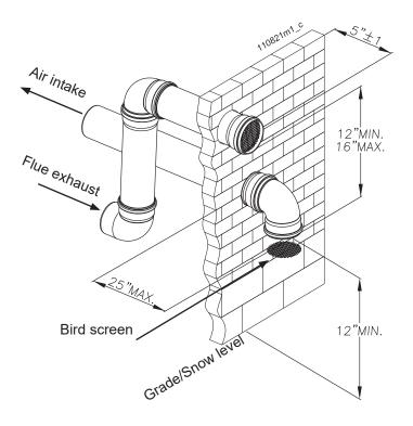
Figure 12-15 Two pipes sidewall termination of air and vent (if space permits)
