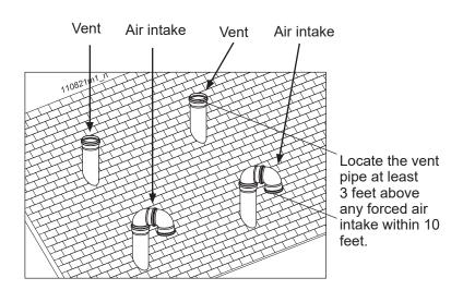
**NOTICE!** Keep the terminals at min. 12" from grade or snow line. Provide vent and air intake with bird screen.
