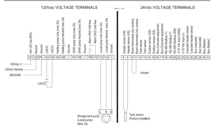
Figure 10-2 Electrical customer connection
