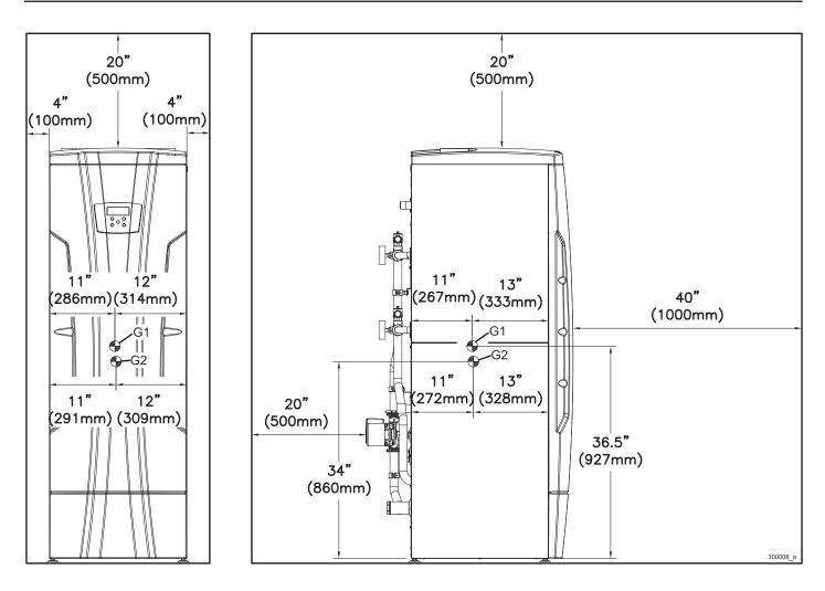
Figure 5-6 Recommended minimum clearance distances for proper installation and servicing for models 199 to 500 (G1 = Center of gravity for 199 and 250 model G2 = Center of gravity for 399 and 500 model)
