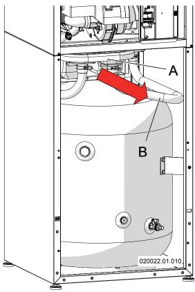
Figure 17-10 Condensate trap "B" and neutralizing box "A"
