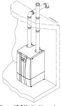
Figure 12-2 Vertical two pipes (Direct Venting).
