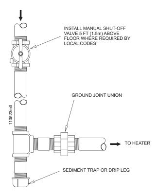
Figure 14-1 Gas supply piping
