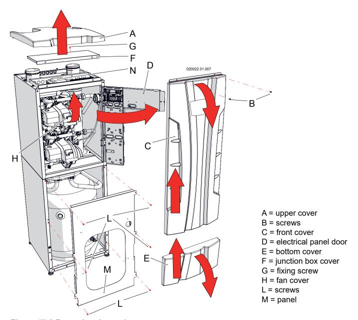
Figure 17-2 Removing the casing
