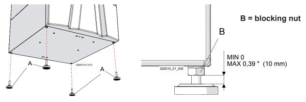
Figure 6-5 Install leveling feet
