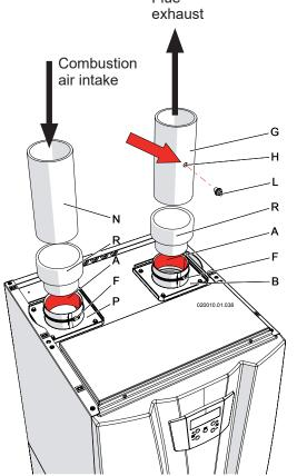
Figure 12-10 Stainless steel air intake/vent connection
