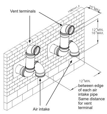
**NOTICE!** Keep the air intake at min. 12" from grade or snow line. Provide vent and air intake with bird screen
