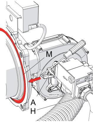
Figure 17-5 Nut and spring that fixes the gas valve
