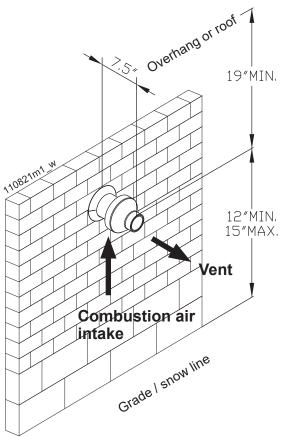
Figure 12-18 Concentric sidewall termination clearances
