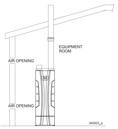
Figure 5-1 Combustion Air direct from outside
