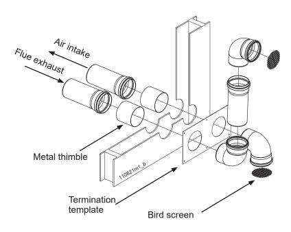
Figure 12-16 Two pipes sidewall termination assembly
