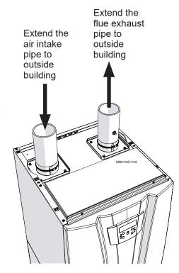
Figure 12-9 PVC/CPVC air intake/Vent connection correctly in place
