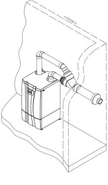
Figure 12-4 Side wall concentric (Direct venting).
