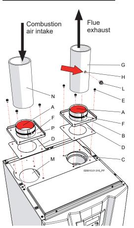
Figure 12-12 Polypropylene air intake/vent connection
