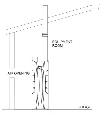
Figure 5-3 Combustion Air from outside - single opening
