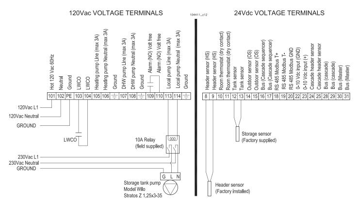
Figure 10-3 Electrical customer connection for pump brand Wilo model Stratos Z1,25X3-35
