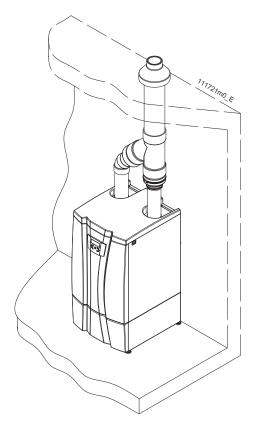
Figure 12-3 Vertical concentric (Direct venting).
