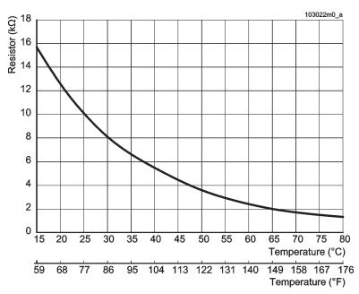
Figure 17-14 Water and flue temperature sensors' curve
