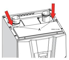
Figure 6-3 Install eyebolt to lift the appliance
