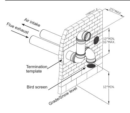
Figure 12-14 Two pipes sidewall termination of air and vent
