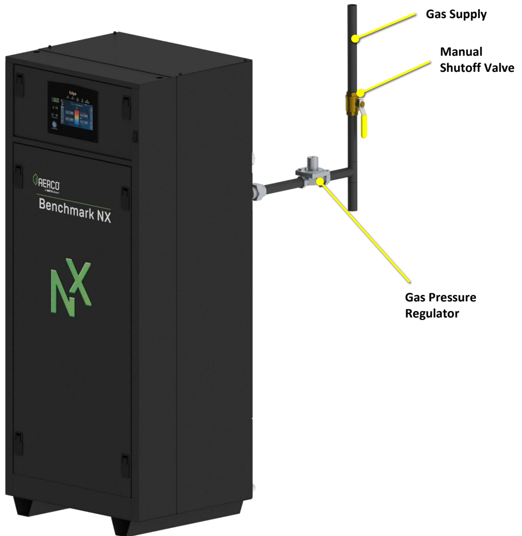
Figure 2: Multiple Boiler Gas Pipe Connections Guidelines
