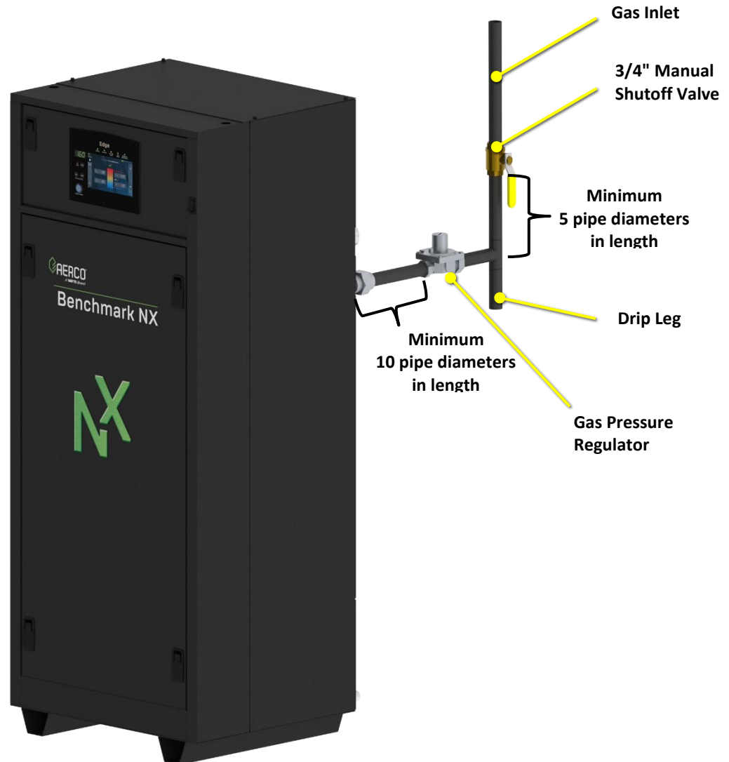
Figure 1: BNX 399/500 Gas Regulator and Manual Shut-Off Valve
