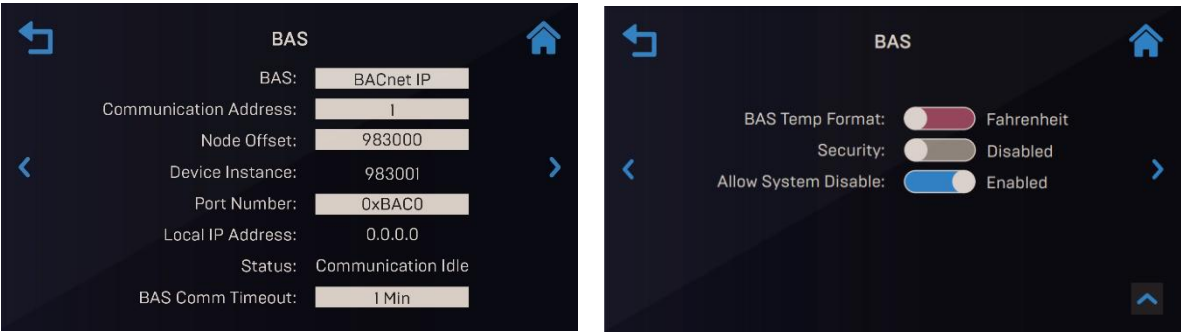
Figure 6-26: Comm & Failsafe : BAS Screen, BAS = BACnet IP
