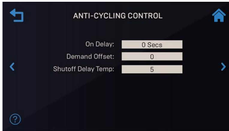
Figure 6-45: Fire Control : Standalone Anti-Cycling Controls
