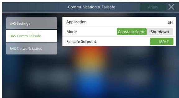
**Figure 6-22: Failsafe Mode - Constant Setpt**
