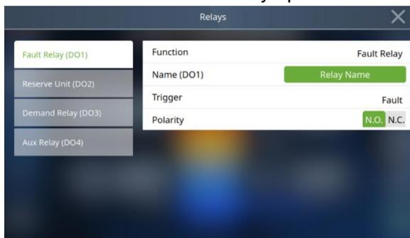
Figure 6-30: Relays > Fault Relay (DO1)
