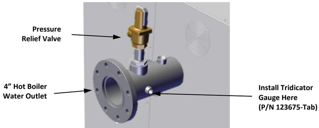
**Figure 2-5: BMK E 216 – 684 P&T Relief Valve Location**
