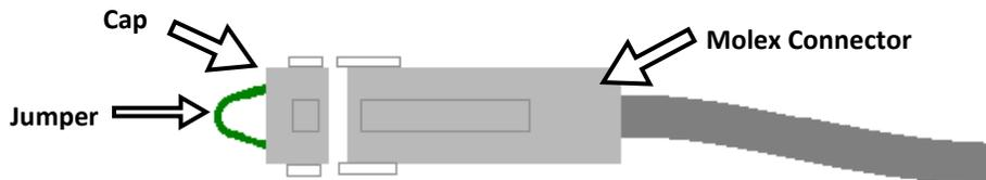
**Figure 2-11: Sequencing Isolation Valve Molex Connector and Jumper Wire**
