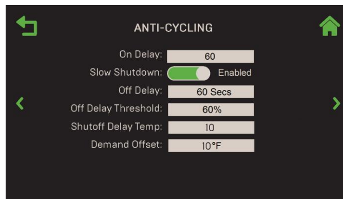
Figure 6-41: Operating Controls : Anti-Cycling Control Screen
