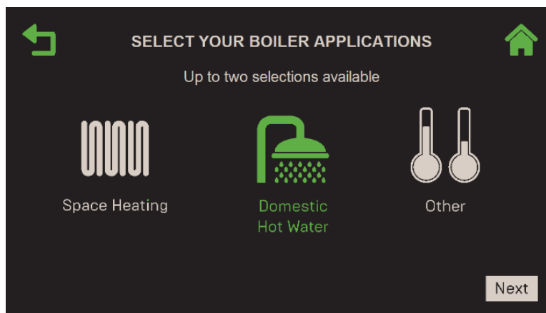
Figure 2-49: BST Manager – DHW: Select Your Boiler Application
