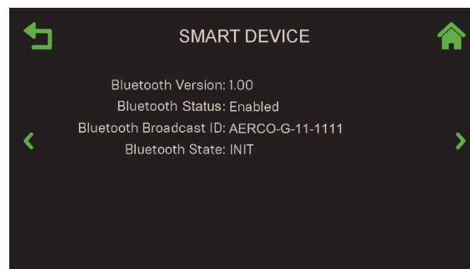
Figure 4-24: Communication & Failsafe: Smart Device Screen
