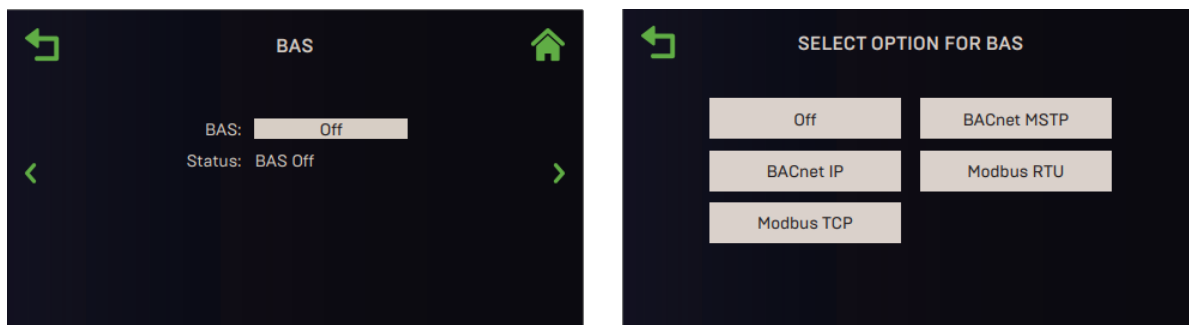
Figure 6-56: Communication & Failsafe : BAS Screens
