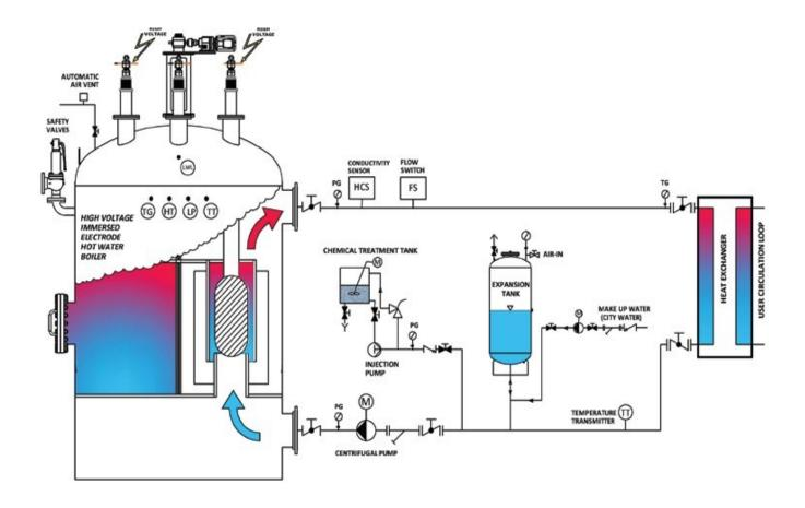
Simplex or duplex **circulation pumps** move the water in the loop. The flow of each pump is determined by the cooling requirements of the electrodes to minimize wear and tear for extended lifespan. Air-cooled pump skids include TEFC motors, usually at building voltage controlled from the System Control Panel. Pressure loss in the loop determines the head of the pump at the required flow.
