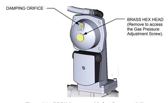
Figure 8-2: SSOV Actuator with Gas Pressure Adjustment
