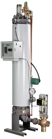
The unit's semi-instantaneous design (steam in tubes and water in shell) is compatible with low or high steam pressures. And installation is easy because of it small footprint (0.37 m<sup>2</sup>) and doorway size. Tight temperature control, low maintenance, longevity and overall reliability make the AERCO DW+ the most logical choice for any commercial or institutional water heating installation.
