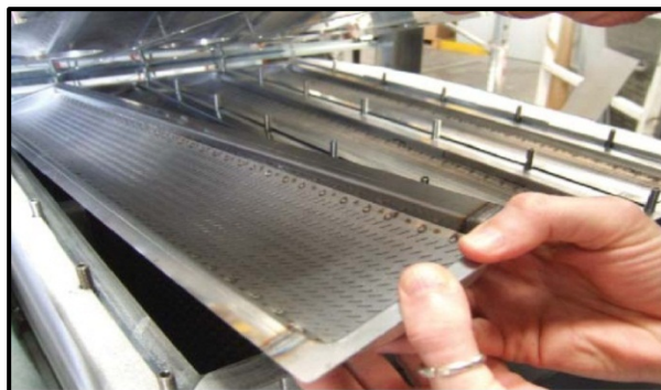
Figure 12: Exposing Burner Modules (Left) and Removing (Right)
