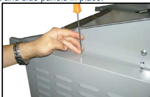
Figure 1: Removing Front & Side Panels
