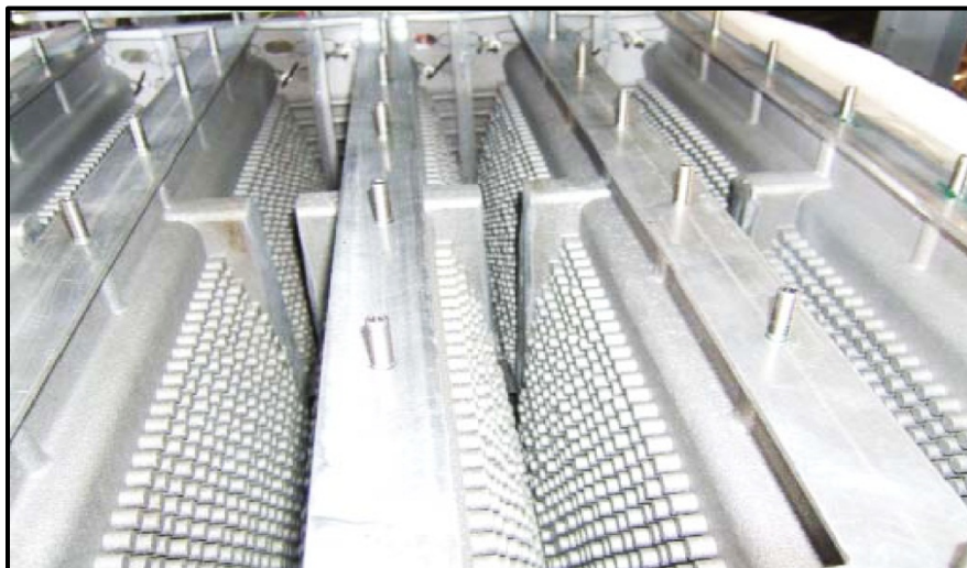
Figure 13: Exposed Combustion Chambers under Burner Modules
