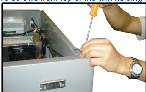
Figure 1: Removing Front & Side Panels
