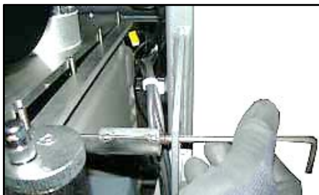
Figure 9: Unscrewing Lift Screw into Tab Hole
