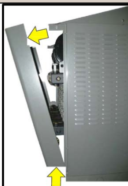
Figure 2: Removing Front & Side Panels
