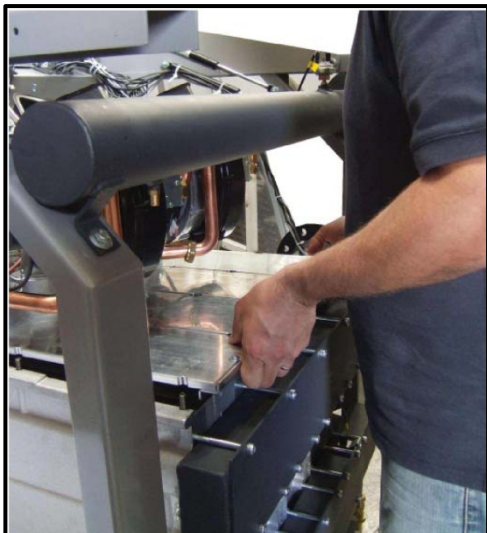
Figure 11: Lifting Burner Plates (Left) to Expose Burner Modules (Right)
