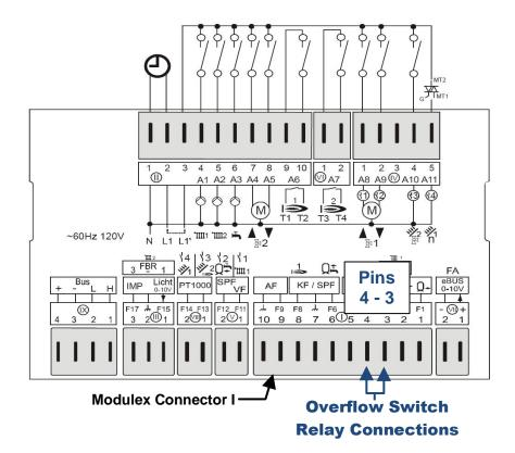
Figure 9: Modulex E8 Controller Wiring for Overflow Switch Relay Connection (Pins 3 & 4 of Connector I)
