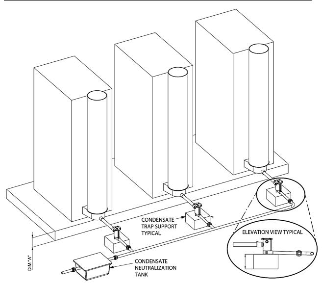
Figure 3: Elevated Multiple Boiler Units with Tank (P/N 89030)
