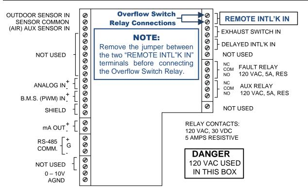
Figure 8: BMK, KC, and INN I/O Box Wiring for Overflow Switch Relay Connection (REMOTE INTL'K IN)
