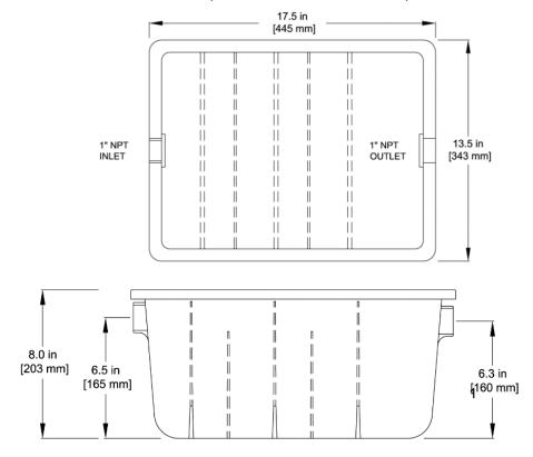
Figure 1: Condensate Neutralization Tank (P/N 89030) Dimensions
