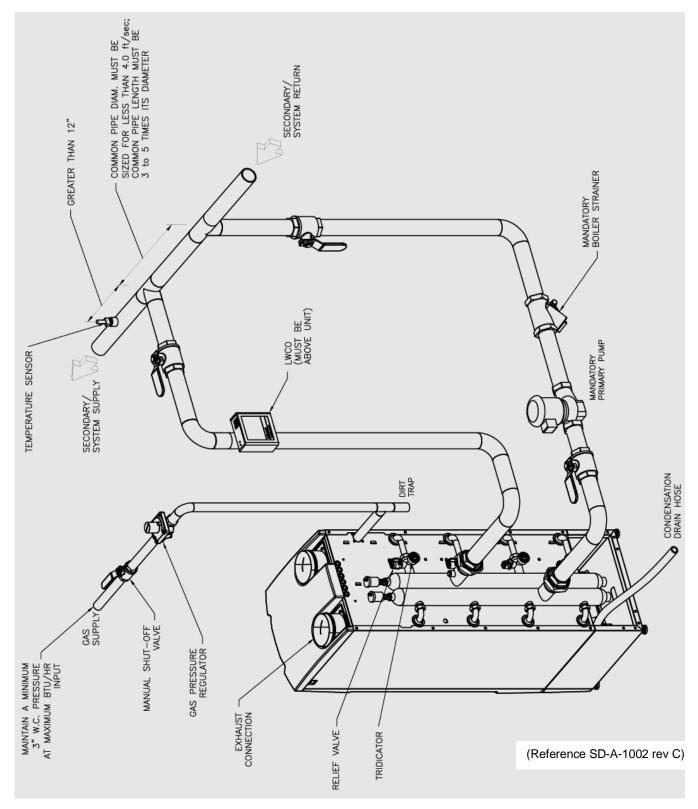
Figure 14: AM 750/1000 Single Unit Installation
