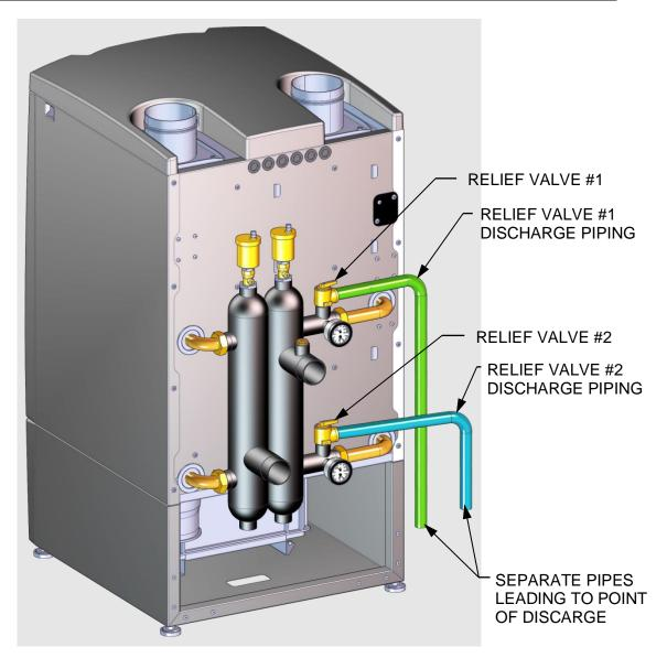
Figure 1: AM 399/500 Relief Valve Point of Discharge Example
