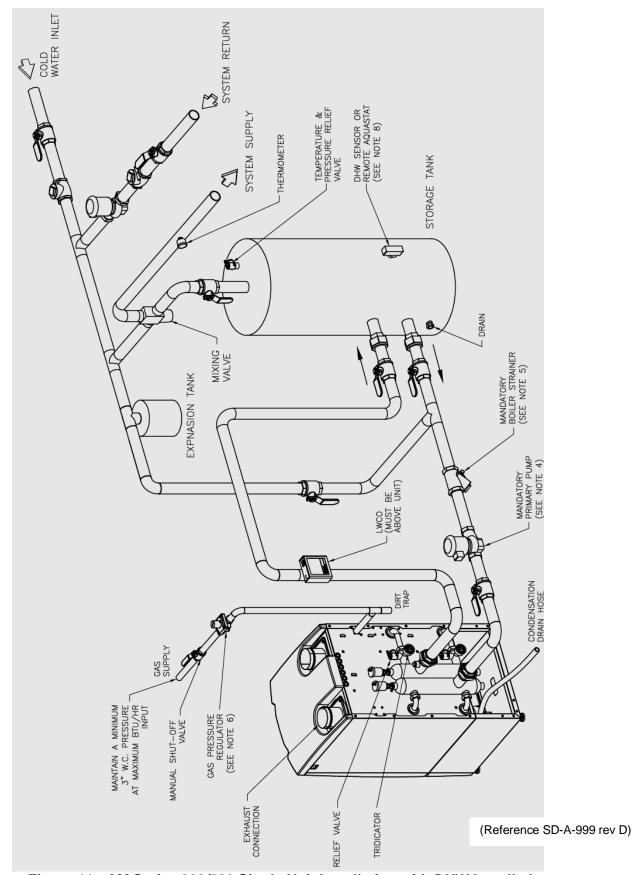
Figure 11: AM Series 399/500 Single Unit Installation with DHW Installed
