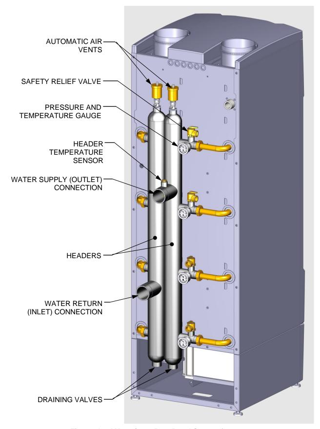
Figure 6b: AM 750/1000 Rear Panel Connections
