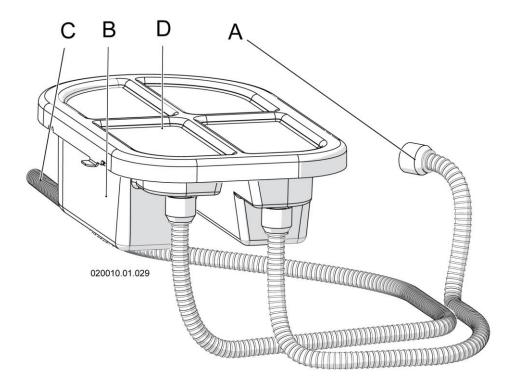
Figure 9: Condensate Drain Assembly Components
