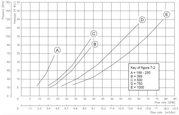
Figure 2: Water Side Pressure Loss Chart
