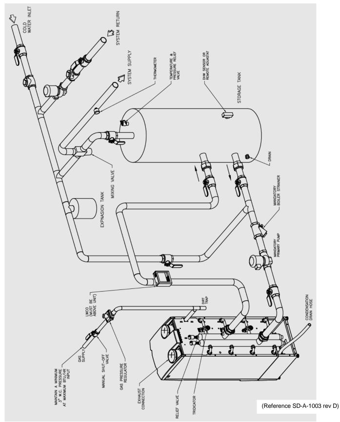
Figure 15: AM Series 750/1000 Single Unit Installation with DHW Installed
