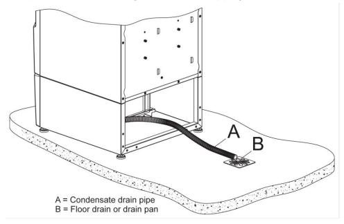
Figure 8: Typical Condensate Drain Installation
