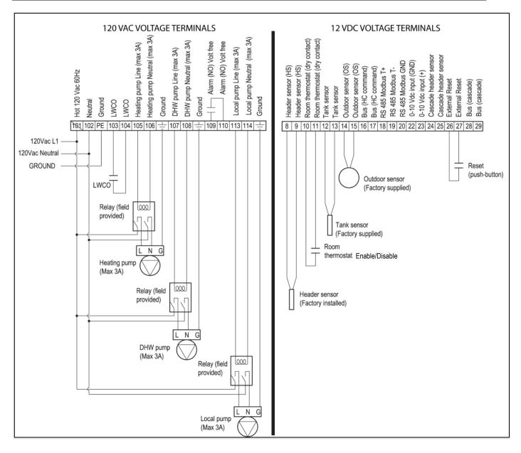
Figure 4: AM BOILER: Electrical Connections
