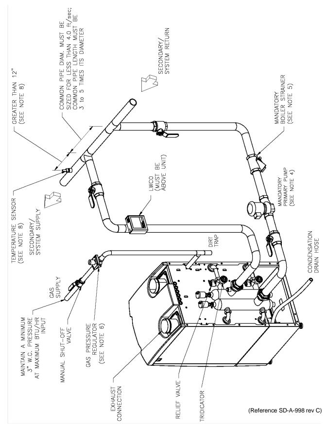
Figure 10: AM 399/500 Single Unit Installation
