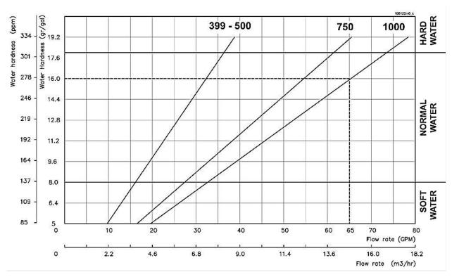
Figure 3: Minimum/Maximum Water Flow in Relation to Water Hardness
