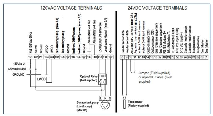
Figure 5: Water Heater Electrical Box Connections
