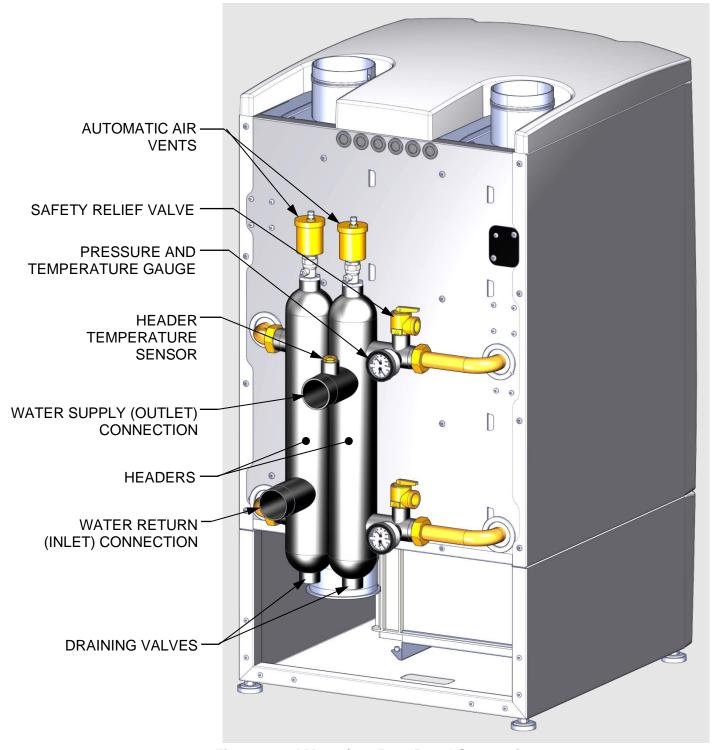
Figure 6a: AM 399/500 Rear Panel Connections
