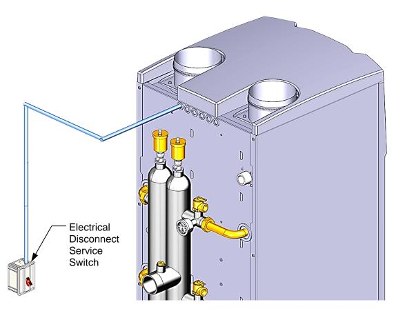
Figure 1: Electrical Disconnect Service Switch Typical Location
