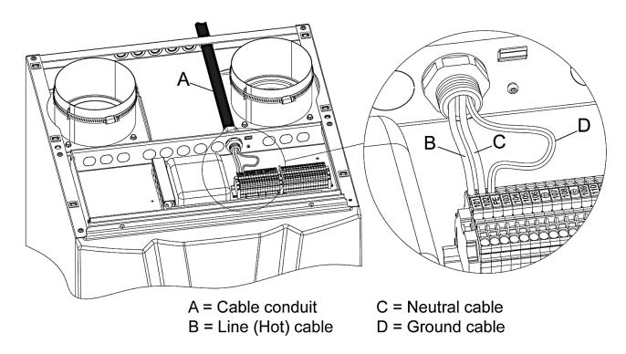
Figure 2: AM Series Boiler and Water Heater Power Wiring
