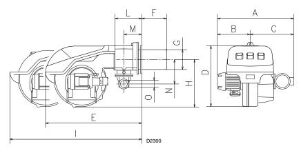
В С D Ε G Н 0 Model М Ν 8 19/32" 5 <sup>5</sup>/<sub>8"</sub> **RLS 68/E** 30 <sup>5</sup>/<sub>32"</sub> 12 <sup>25</sup>/<sub>32"</sub> 17 <sup>13</sup>/<sub>32"</sub> 23 <sup>15</sup>/<sub>64"</sub> 40 <sup>61</sup>/<sub>64"</sub> 9 59/64" 16 <sup>15</sup>/<sub>16"</sub> 8 3/4" 2"  $63^{1}/_{2}$  $30^{5}/_{32}$   $12^{25}/_{32}$   $17^{13}/_{32}$   $23^{15}/_{64}$   $40^{61}/_{64}$ 9 59/64" 8 19/32" 2" **RLS 120/E**  $5^{5}/_{8"}$ 8 3/4"
