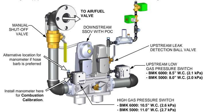
Figure 4-1: Port Location for Combustion Calibration
