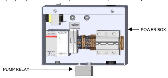
Figure 2-16: Pump Relay Location
