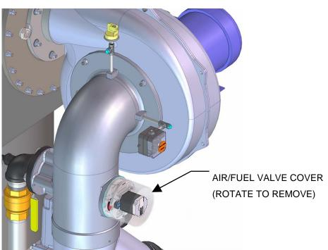
Figure 5-8: Air/Fuel Valve Cover Location
