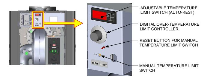
Figure 4-5: Over-Temperature Limit Switch Location
