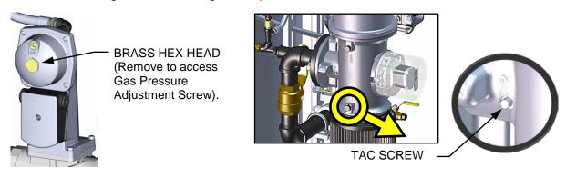
Figure 4-3: Gas Pressure Adjustment Screw and TAC Screw Location
