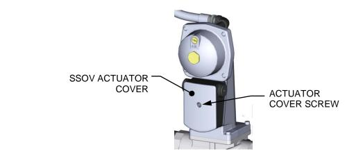
Figure 5-7: SSOV Actuator Cover Location
