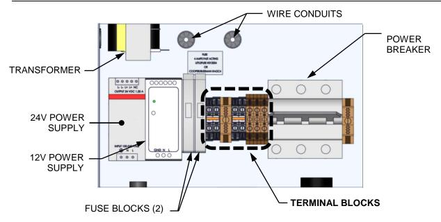
Figure 2-12: Power Box Internal Components (Cover Removed)
