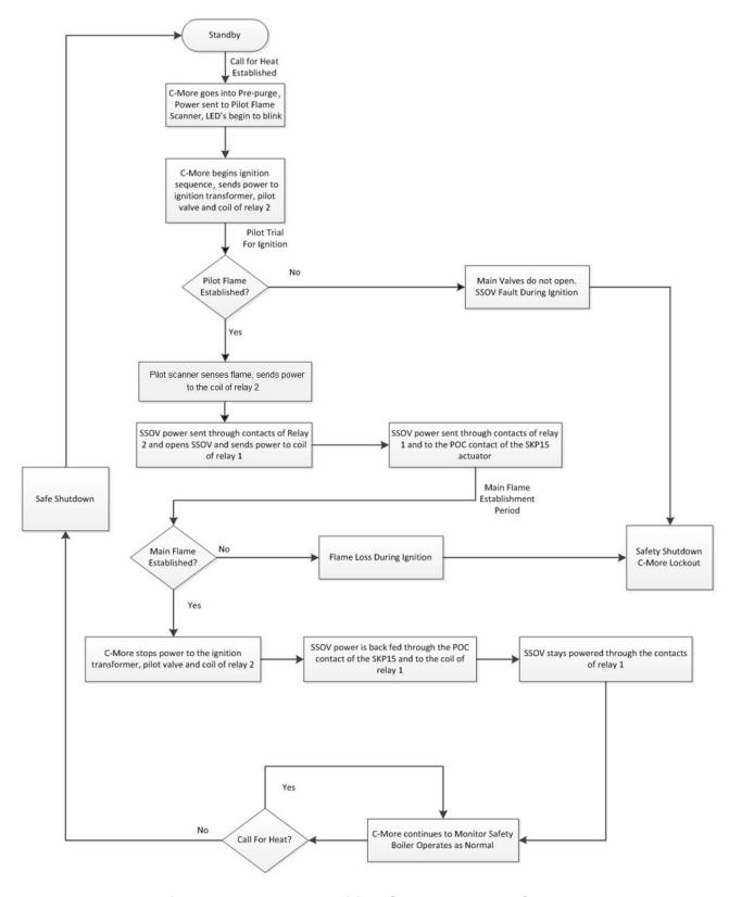
Figure 3-7: Burner Ignition Sequence Flow Chart
