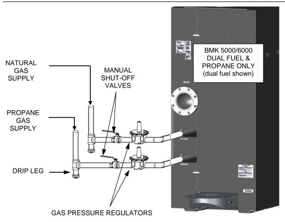
Figure 2-10: Manual Gas Shut-Off Valve Location
