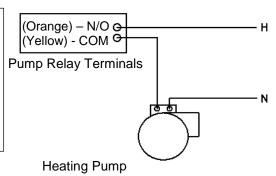
Figure 2-17: Schematic - System Pump Start using Boiler Pump Relay
