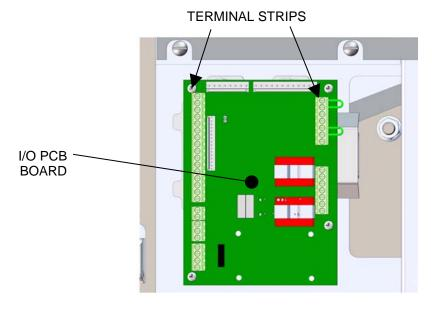
Figure 2-14b: Input/Output (I/O) Box - Cover Removed
