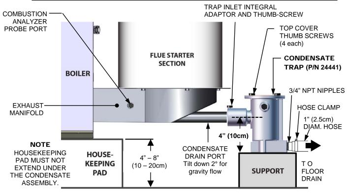
Figure 2-9: Sample Condensate Trap Installation
