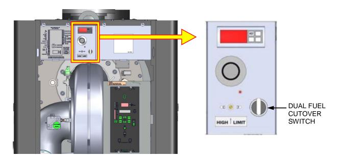
Figure 4-4: Dual Fuel Switch Location
