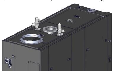
Figure 2-6. Pressure Relief Valve Installation Locations
