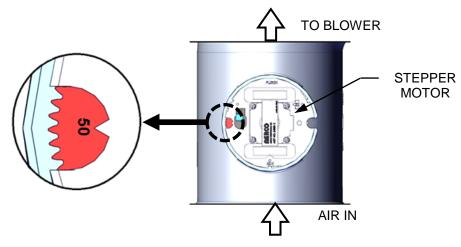
Figure 3-4: Air/Fuel Valve in Ignition Position
