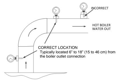
Figure 2-7: Pressure/Temperature Gauge Installation Location
