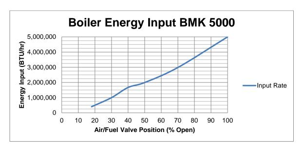
Figure 3-5: Relationship Between BMK 5000 Air/Fuel Valve Position and Energy Input
