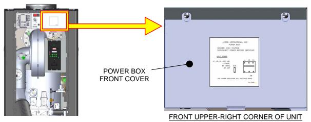
Figure 2-11: Power Box with Closed Cover
