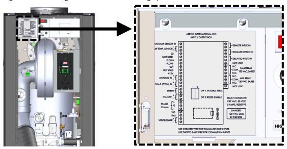
Figure 2-14a: Input/Output (I/O) Box Location
