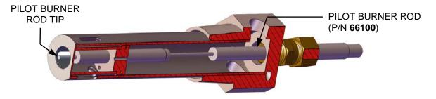
Figure 4-1b: Pilot Burner & Pilot Ignition Rod – Cross-Section
