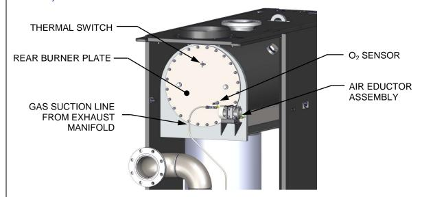
Figure 4-8: Partial Rear View Showing Rear Burner Plate
