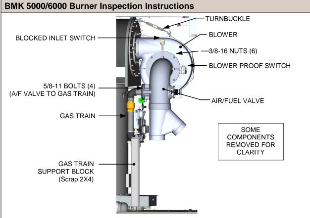
Figure 4-5b: Burner Assembly Mounting Details – Left Side View
