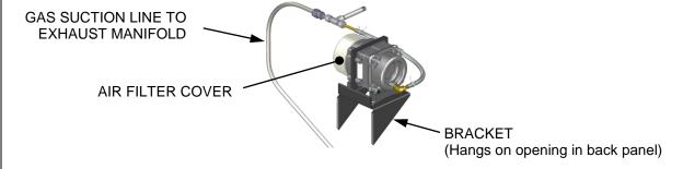
Figure 4-3: Air Eductor Assembly – Shown Removed from Unit
