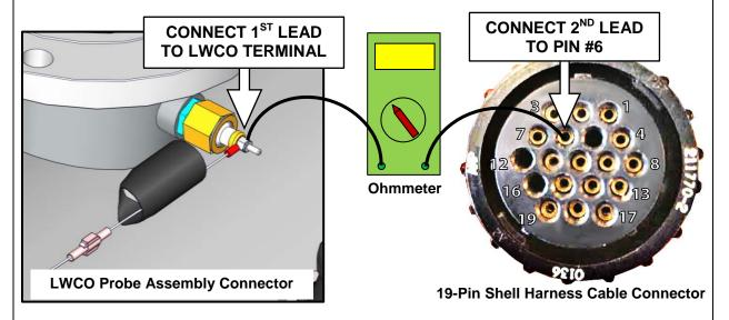
Figure 4-14: Connecting Ohmmeter between LWCO Probe & Shell Harness Cable
