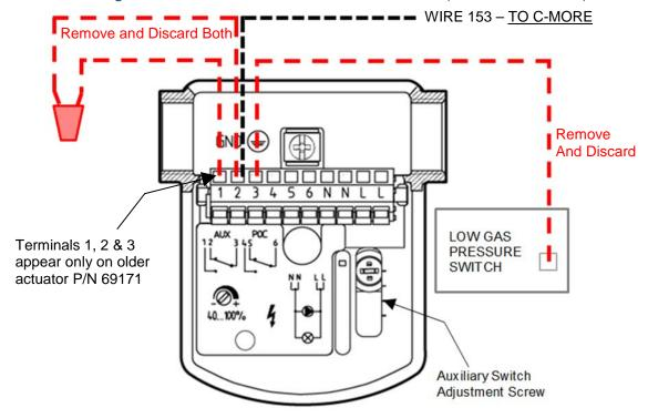
Figure 4-15: Wiring Compartment on Older Actuator (P/N 69171)
