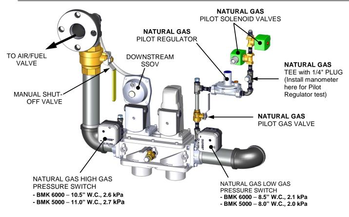
Figure 5-1: Gas Train Component and Pilot Gas Valve Location
