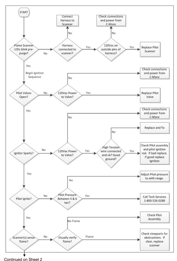
Figure 5-4a: Pilot Assembly Troubleshooting Flow Chart (Sheet 1 of 2)
