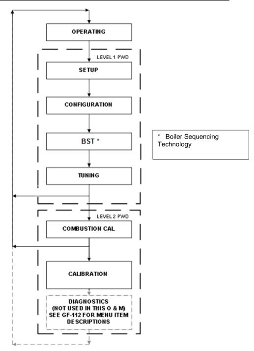
\* Boiler Sequencing Technology (BST) appears only if enabled. See Section 6 in the Benchmark 5000 – 6000 Installation and Startup Guide-INTERNATIONAL OMM-0129 (GF-207-I) for instructions.
