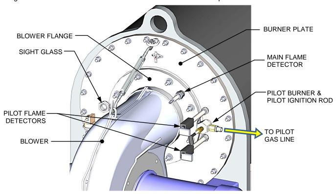
Figure 4-1a: Pilot Burner, Main & Pilot Flame Detector Mounting Locations
