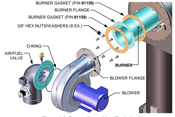
Figure 4-6: Burner Assembly – Exploded View
