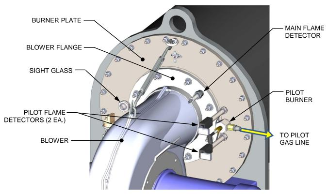
Figure 5-2: Pilot Burner & Flame Detector Locations
