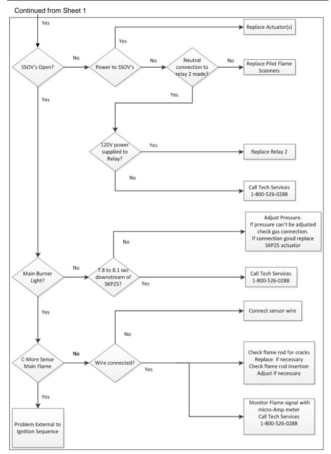
Figure 5-4b: Pilot Assembly Troubleshooting Flow Chart (Sheet 2 of 2)
