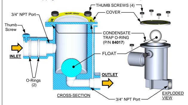
Figure 4-10: External Condensate Trap – Cross-Section & Exploded View
