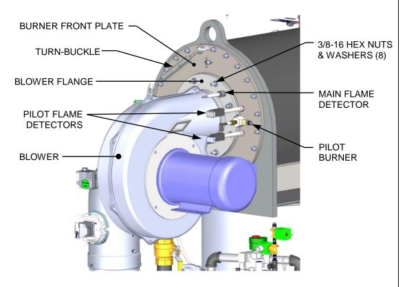
Figure 4-5a: Burner Assembly Mounting Details – Right-Front View
