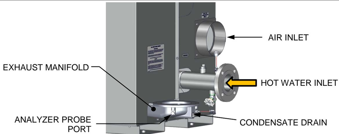
**Figure 4-2a: BMK 750 & 1000 Analyzer Probe Port Location**
