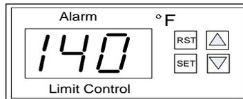
Figure 4-7: Digital Over-Temperature Alarm Switch Front Panel
