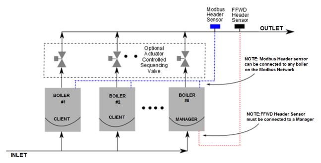
Figure 6-1: Simplified BST Block Diagram
