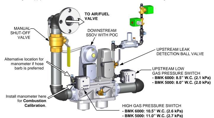
Figure 4-1: Port Location for Combustion Calibration
