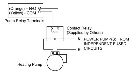
Figure 2-18: Schematic – System Pump Start using a Separate Contact Relay
