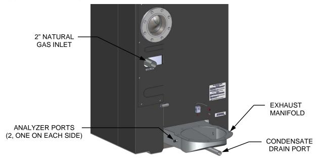
Figure 2-8: Condensate Drain Connection Location
