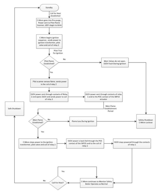
Figure 3-7: Burner Ignition Sequence Flow Chart
