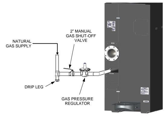
Figure 2-10: Manual Gas Shut-Off Valve Location
