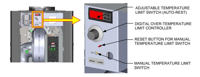
Figure 4-4: Over-Temperature Limit Switch Location
