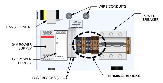
Figure 2-12: Power Box Internal Components (Cover Removed)
