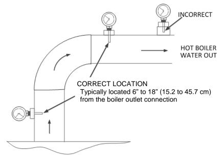
Figure 2-7: Pressure/Temperature Gauge Installation Location
