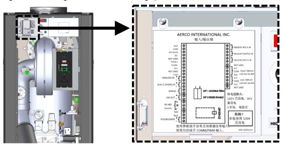
Figure 2-14a: Input/Output (I/O) Box Location
