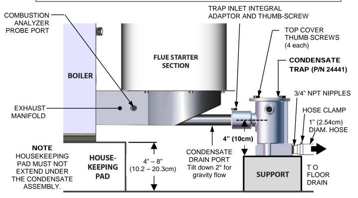
Figure 2-9: Sample Condensate Trap Installation
