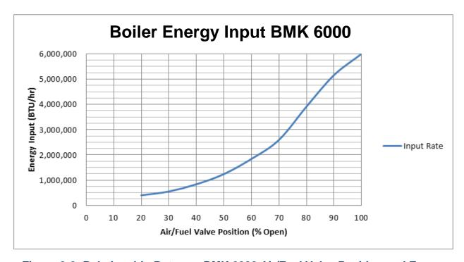
Figure 3-6: Relationship Between BMK 6000 Air/Fuel Valve Position and Energy Input
