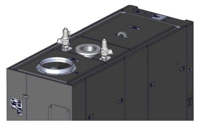
Figure 2-6. Pressure Relief Valve Installation Locations
