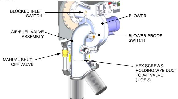
Figure 5-5: Blower Proof & Blocked Inlet Switch Locations
