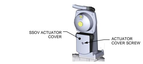
Figure 5-7: SSOV Actuator Cover Location
