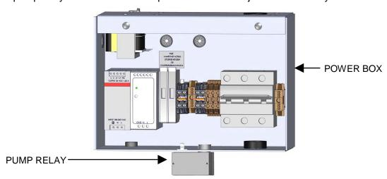
Figure 2-16: Pump Relay Location
