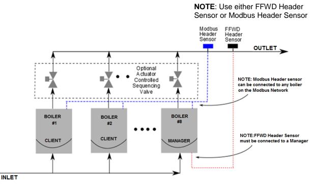
Figure 6-1: Simplified BST Block Diagram
