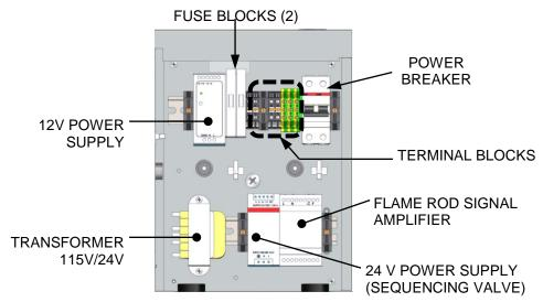
Figure 2-9a: BMK 750/1000 Power Box Internal Components
