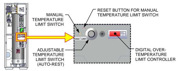
Figure 4-6a: BMK 750 & 1000 Over-Temperature Limit Switch Location
