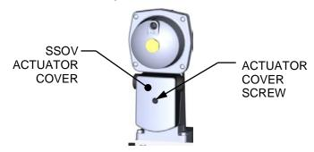
Figure 5-9: SSOV Actuator Cover Location
