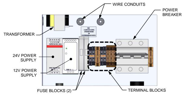
Figure 2-9c: BMK 2500/3000 Power Box Internal Components
