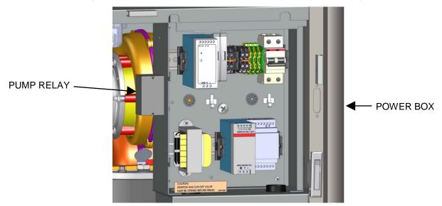
Figure 2-12a: BMK 750/1000 Pump Relay Location
