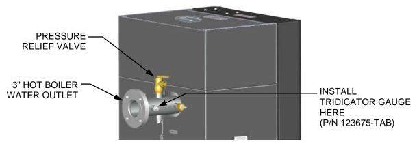
Figure 2-5a: BMK 750/1000 P&T Relief Valve Location
