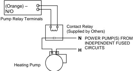
Figure 2-14: Schematic – System Pump Start using a Separate Contact Relay
