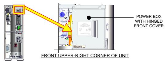
Figure 2-8a: BMK 750/1000 Power Box with Closed Cover
