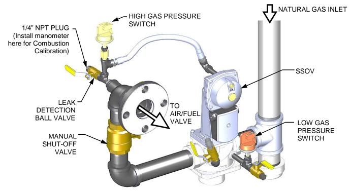
Figure 4-1c: BMK 2500 1/4 Inch Gas Plug Location
