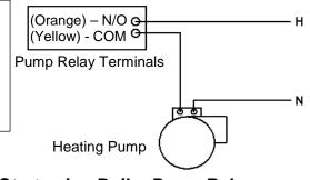
Figure 2-13: Schematic – System Pump Start using Boiler Pump Relay
