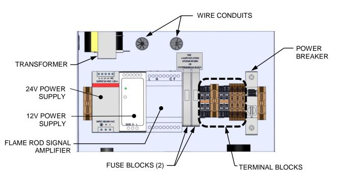
Figure 2-9b: BMK 1500/2000 Power Box Internal Components
