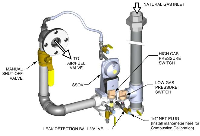
Figure 4-1b: BMK 1500 & 2000 1/4 Inch Gas Plug Location
