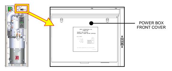
Figure 2-8b: BMK 1500/2000/2500/3000 Power Box with Closed Cover
