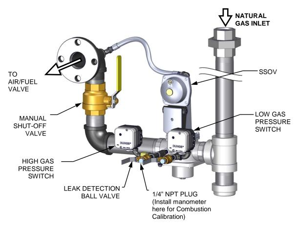
Figure 4-1d: BMK 3000 1/4 Inch Gas Plug Location
