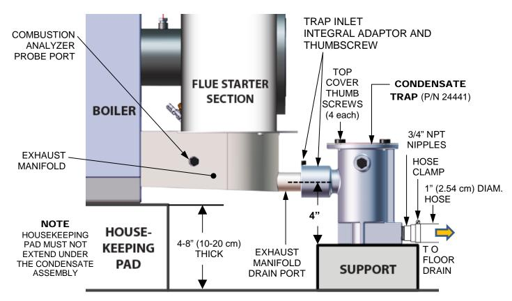
Figure 2-6b: BMK 1500/2000/2500/3000 Sample Condensate Trap Installation
