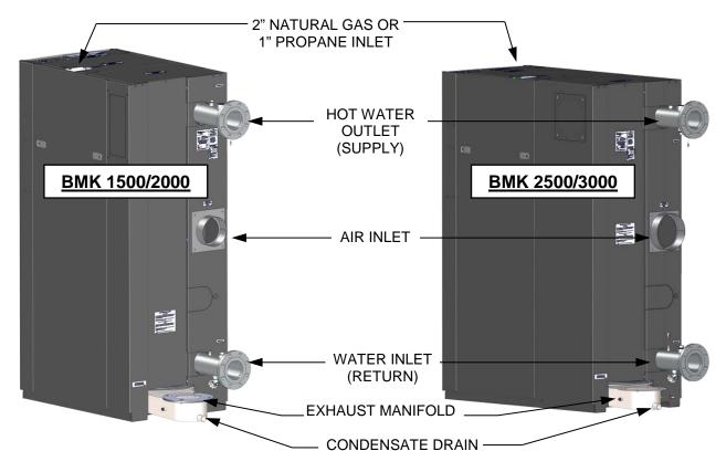
Figure 2-4b: BMK 1500/2000 and BMK 2500/3000 Supply and Return Locations
