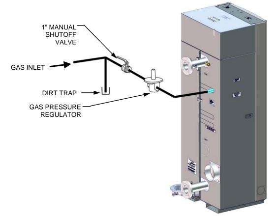
Figure 2-7a: BMK 750/1000 Manual Gas Shut-Off Valve and Gas Regulator
