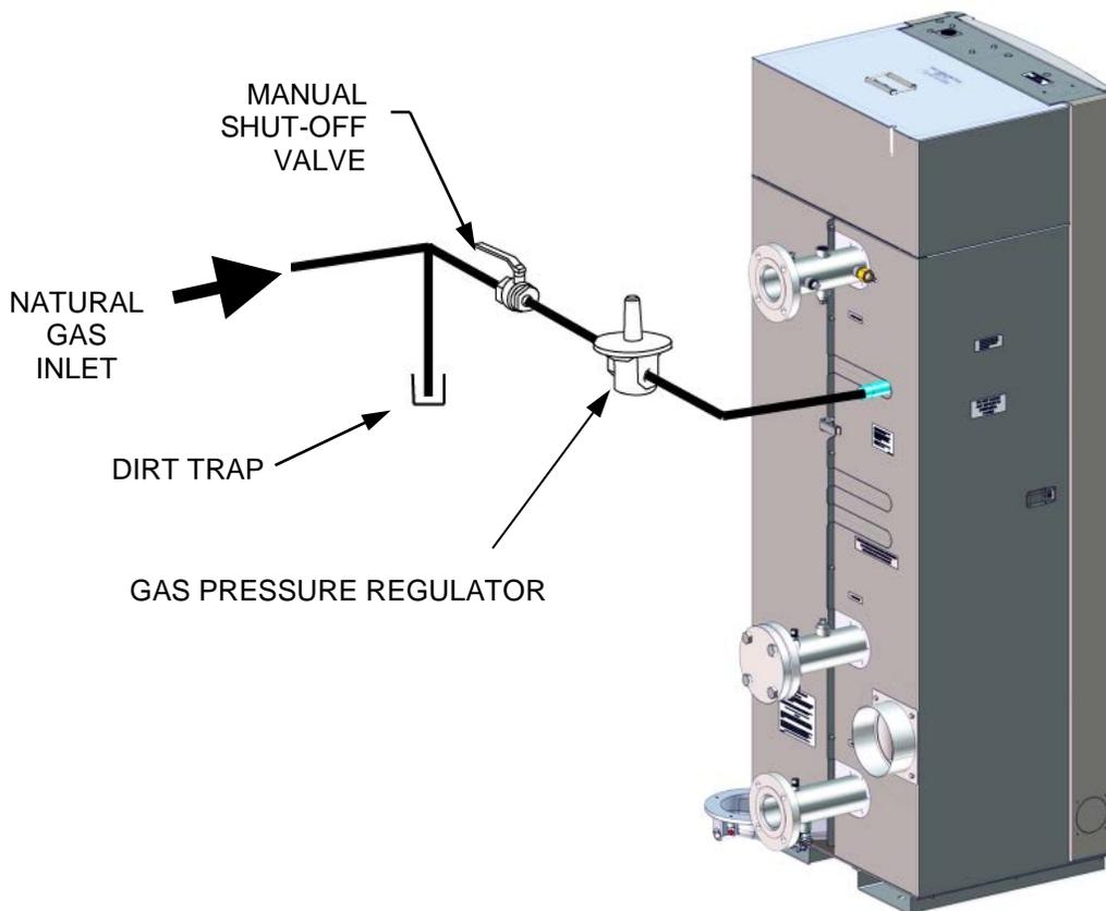
**Figure 2-7: Manual Gas Shut-Off Valve Location**
