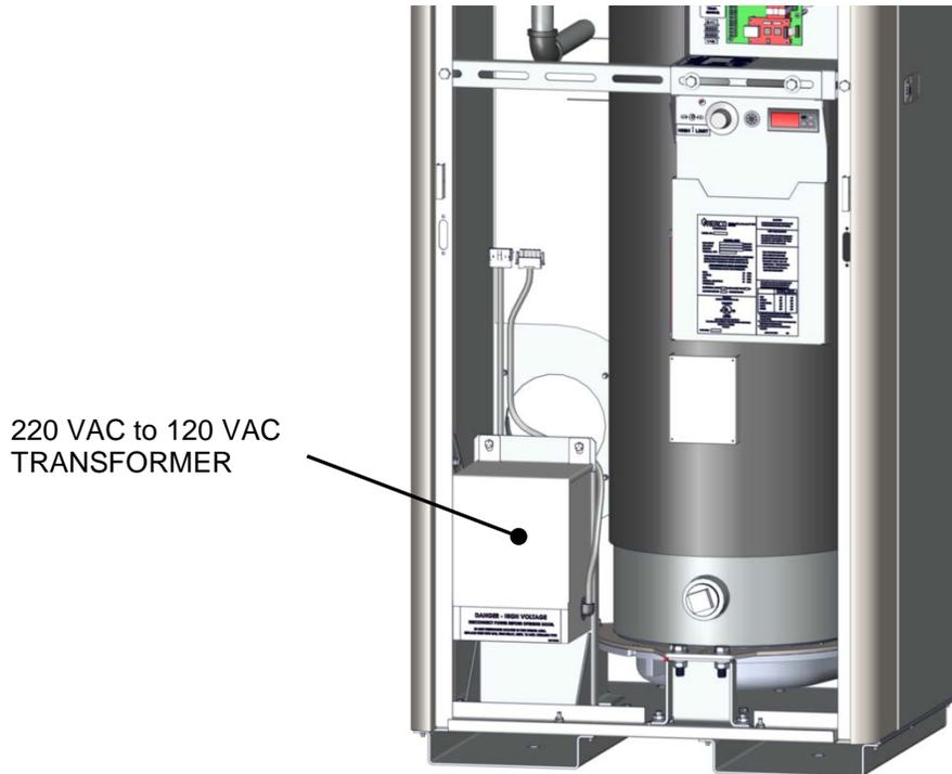
**Figure L1. 220V Transformer – Front Panel Removed**
