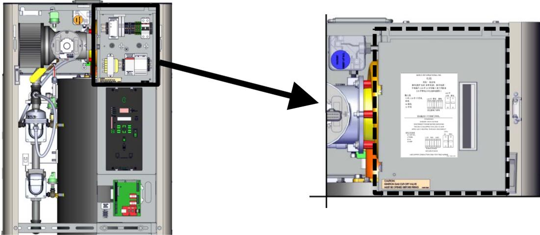
**Figure 2-8: Power Box Location with Cover Closed**
