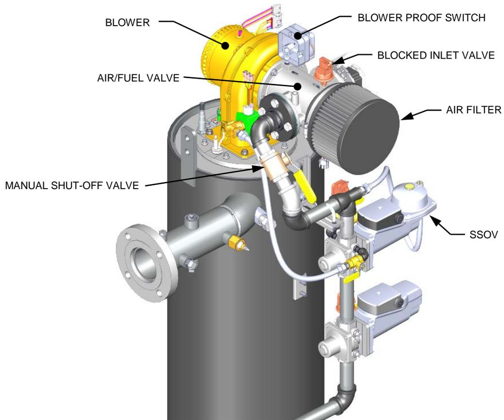
**Figure 6-3: Bare Heating Boiler – Partial View**
