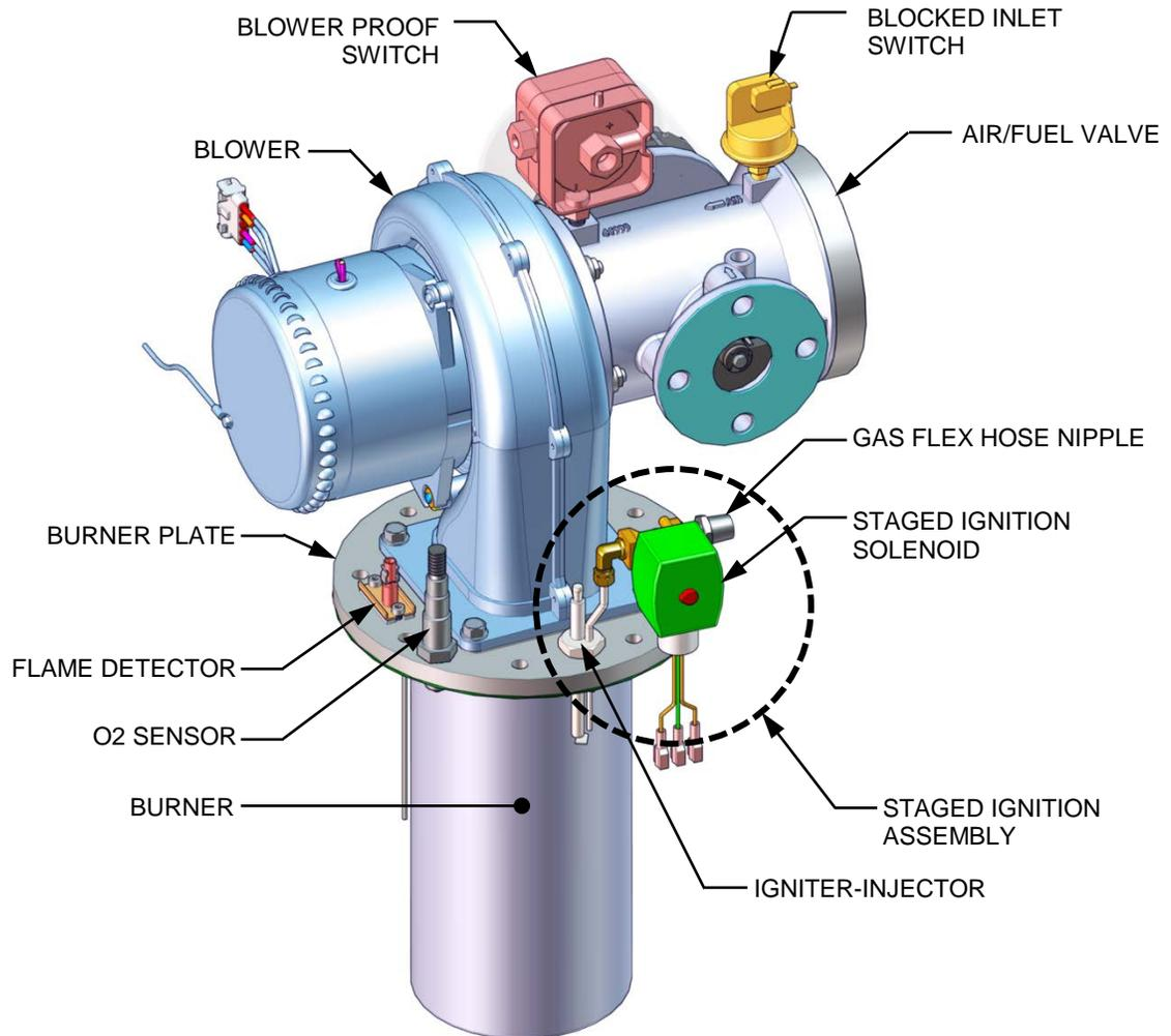
**Figure 7-1: Benchmark 750/1000 Burner Assembly (Removed from Unit)**
