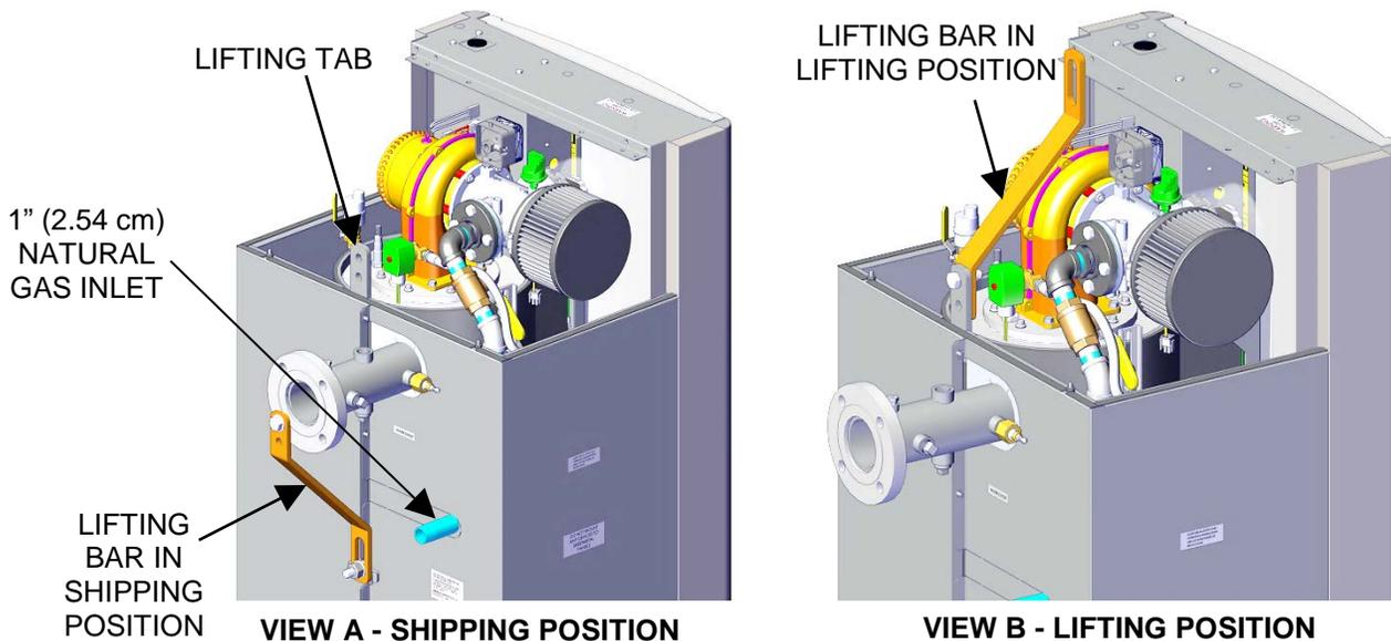
**Figure 2-2: Heating Boiler Lifting Provisions**
