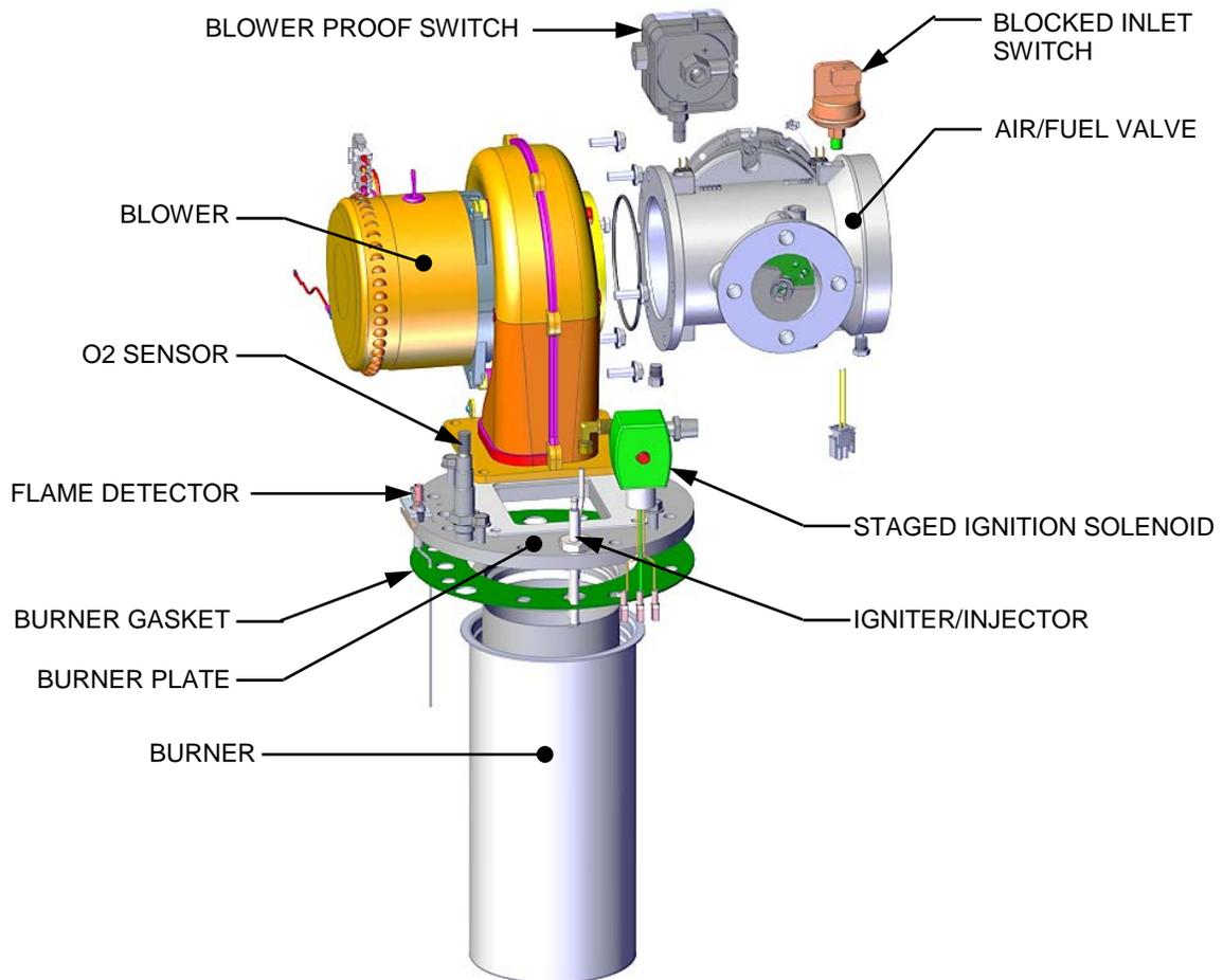
**Figure 7-5: Burner Assembly – Exploded View**
