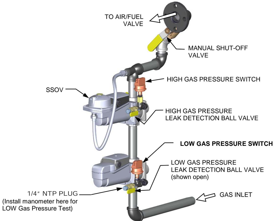
**Figure 6-1a: Low Gas Pressure Test**
