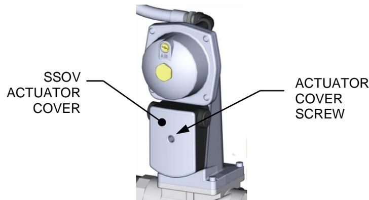
**Figure 6-6: SSOV Actuator Cover Location**
