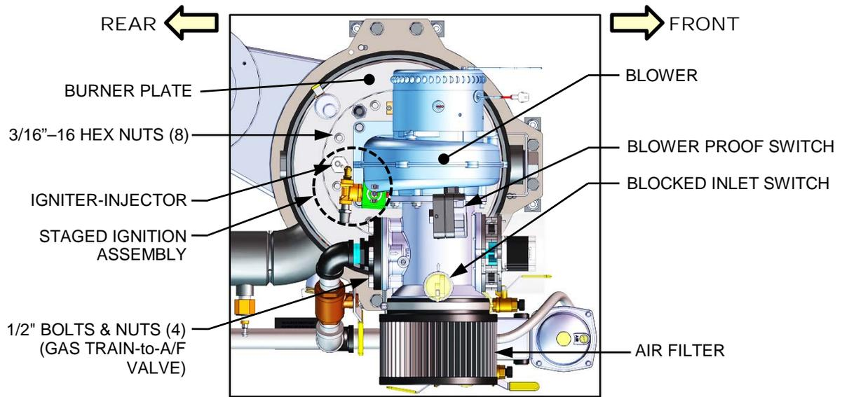
**Figure 7-4: Burner Assembly Mounting Details – Overhead View**
