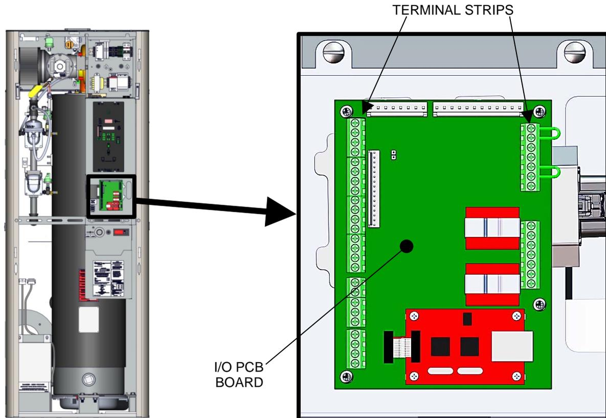
**Figure 2-11: Input/Output (I/O) Box Location**
