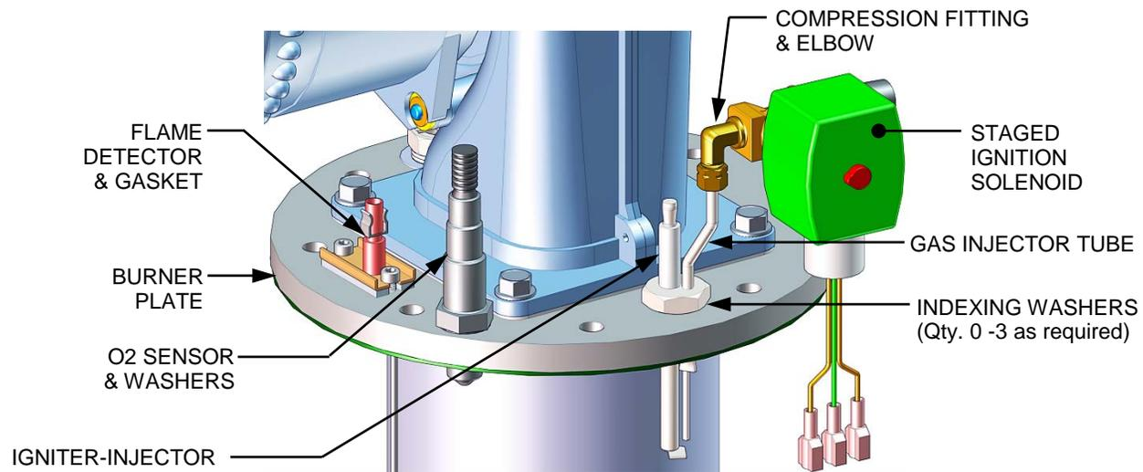
**Figure 8-2: Staged Ignition Connection to Gas Injector Tube**
