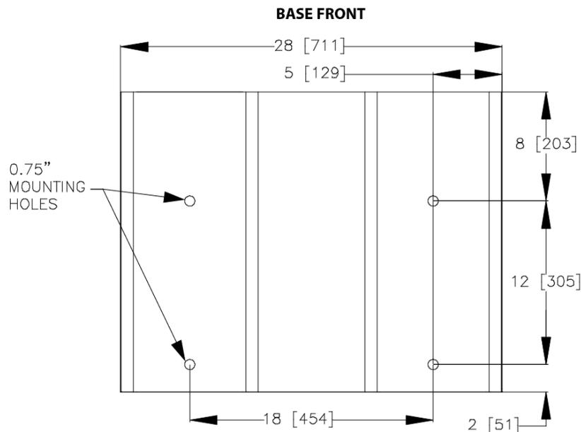
**Figure 2-1b: Benchmark 750/1000 Anchor Bolt Locations**
