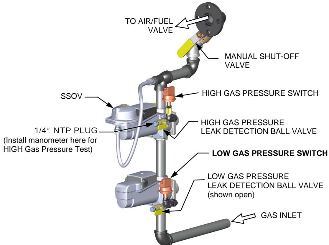
**Figure 6-1b: High Gas Pressure Fault Test**
