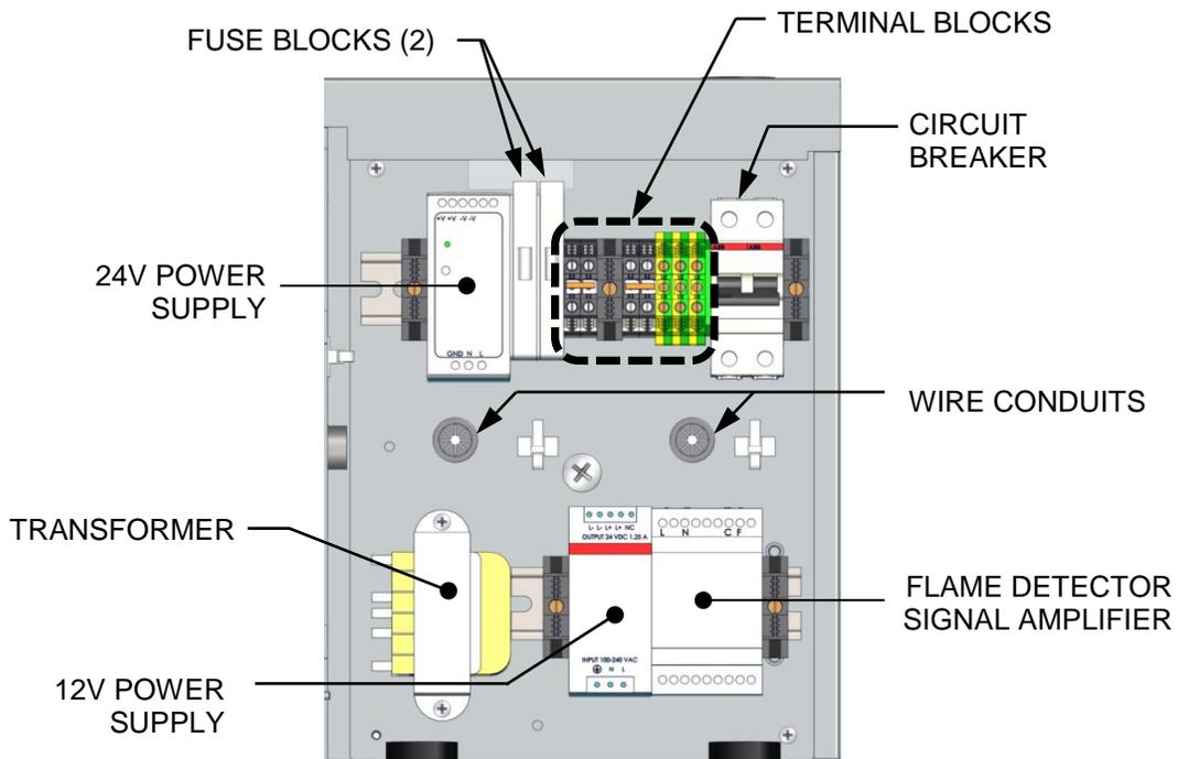
**Figure 2-9: Power Box Internal Components**
