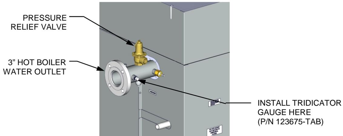
**Figure 2-4: P&T Relief Valve Location**
