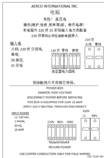
**Figure 2-10: Power Box Cover Labels – 220 VAC**
