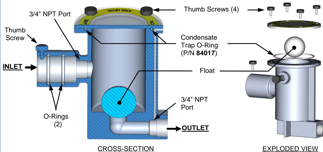
**Figure 7-6: External Condensate Trap – Cross-Section & Exploded View**
