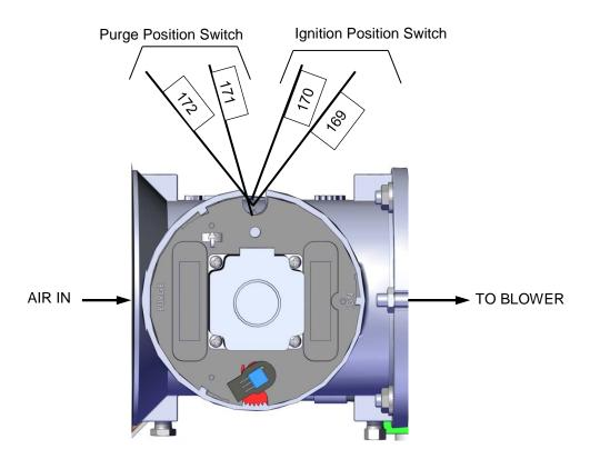
Figure 6-8: Air/Fuel Valve Purge and Ignition Switch Locations
