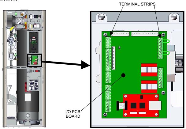
Figure 2-11: Input/Output (I/O) Box Location
