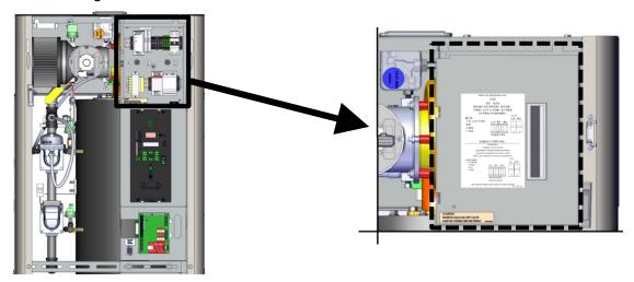
Figure 2-8: Power Box Location with Cover Closed
