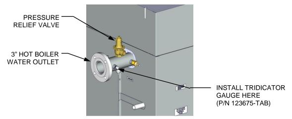
Figure 2-4: P&T Relief Valve Location
