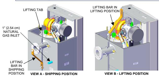
Figure 2-2: Heating Boiler Lifting Provisions
