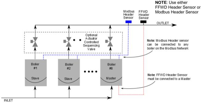
Figure 9-1. Simplified BST Block Diagram
