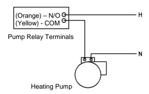
Figure 2-16: Schematic – System Pump Start using Boiler Pump Relay
