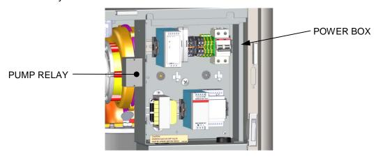
Figure 2-15: Pump Relay Location
