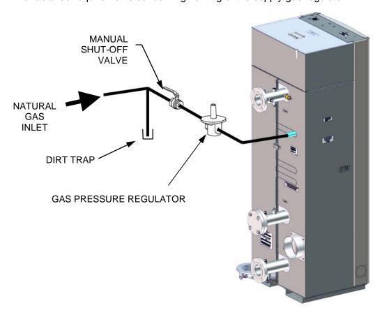
Figure 2-7: Manual Gas Shut-Off Valve Location
