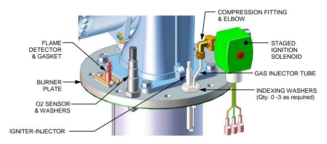
Figure 8-2: Staged Ignition Connection to Gas Injector Tube
