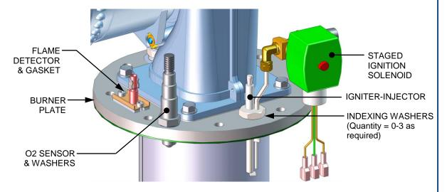
Figure 7-2: Igniter-Injector & Flame Detector Mounting Details
