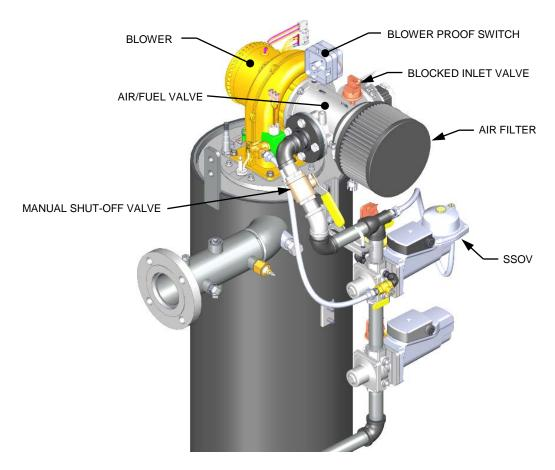
Figure 6-3: Bare Heating Boiler – Partial View
