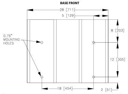
Figure 2-1b: Benchmark 750/1000 Anchor Bolt Locations
