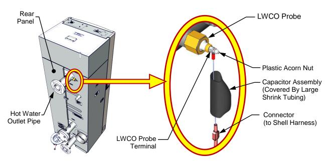
Figure 7-8: LWCO Probe Location (BMK750 Shown)
