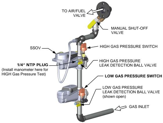
Figure 6-1b: High Gas Pressure Fault Test
