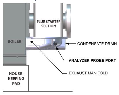
Figure 4-2: Analyzer Probe Port Location (Right Side Partial View)
