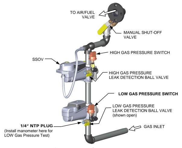
Figure 6-1a: Low Gas Pressure Test
