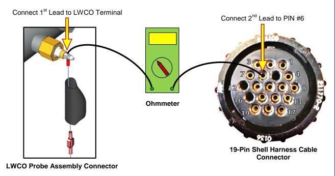
Figure 7-10: Connecting Ohmmeter between LWCO Probe & Shell Harness Cable
