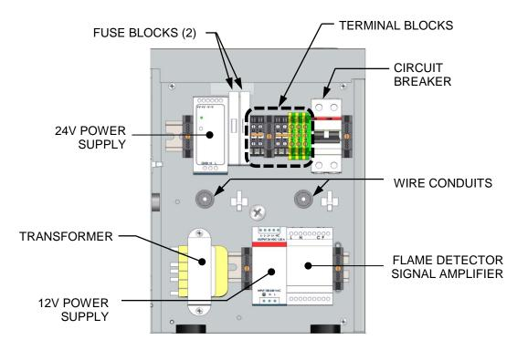
Figure 2-9: Power Box Internal Components
