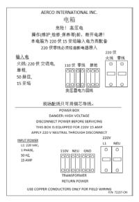
Figure 2-10: Power Box Cover Labels – 220 VAC
