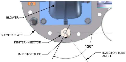
Figure 7-3: Igniter-Injector Orientation (Viewed Looking Down from Above)
