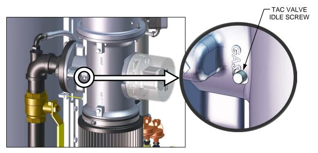
Figure 4-4: TAC Valve Adjust (Idle Screw)
