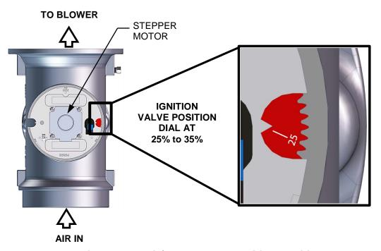
Figure 3-6: Air/Fuel Valve In Ignition Position
