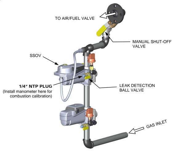
Figure 4-1: 1/4 Inch Gas Plug Location for Combustion Calibration
