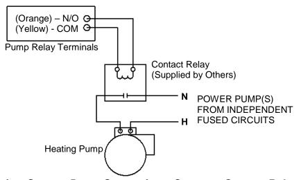
Figure 2-17: Schematic – System Pump Start using a Separate Contact Relay
