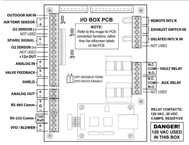
Figure 2-12: I/O Box Terminal Strips
