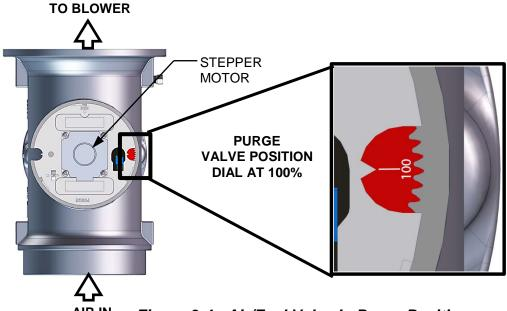
N Figure 3-4: Air/Fuel Valve In Purge Position
