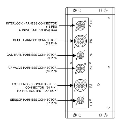
Figure J-2: Benchmark Control Panel Rear View
