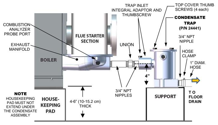
Figure 2-6a: BMK 750/1000 Sample Condensate Trap Installation
