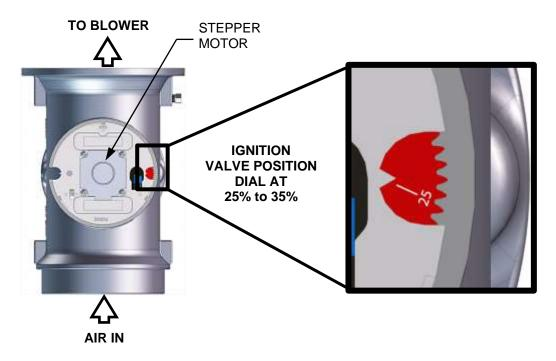
Figure 3-4: Air/Fuel Valve In Ignition Position
