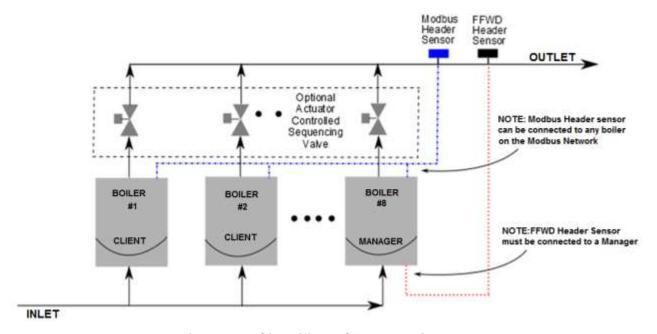
Figure 6-1: Simplified BST Block Diagram
