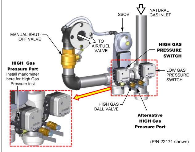
Figure 5-4: <u>BMK 3000</u> HIGH Gas Pressure Test Components
