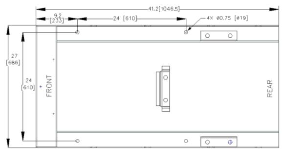
Figure 2-2a: BMK 750/1000 Anchor Bolt Locations
