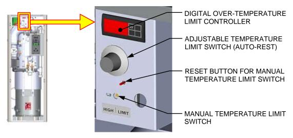
Figure 4-6b: BMK 1500 – 3000 Over-Temperature Limit Switch Location
