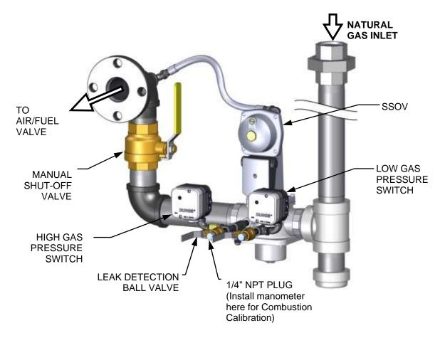
Figure 4-1d: BMK 3000 1/4 Inch Gas Plug Location (P/N 22171 shown)
