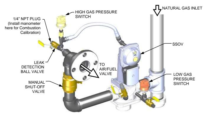
Figure 4-1c: BMK 2500 1/4 Inch Gas Plug Location (P/N 22190 shown)
