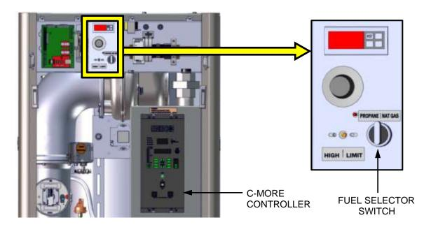
PARTIAL FRONT VIEW WITH FRONT COVER REMOVED
