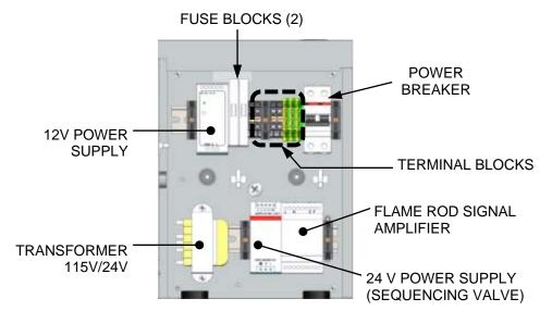
Figure 2-9a: BMK 750/1000 Power Box Internal Components
