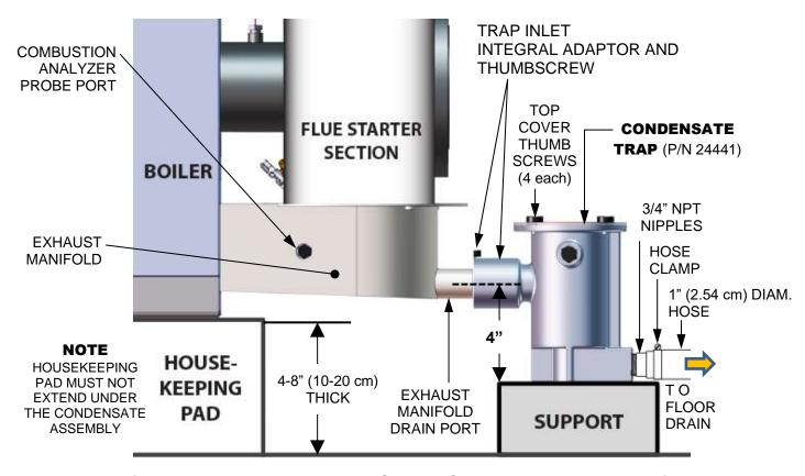
Figure 2-6b: BMK 1500 - 3000 Sample Condensate Trap Installation
