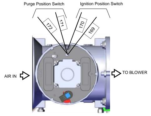
Figure 5-11b: Air/Fuel Purge and Ignition Locations— BMK 750/1000
