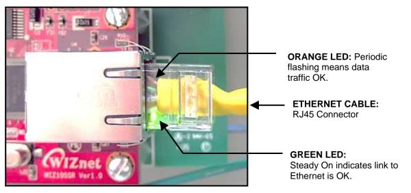
Figure 7-2: Ethernet Link and Data Traffic LEDs
