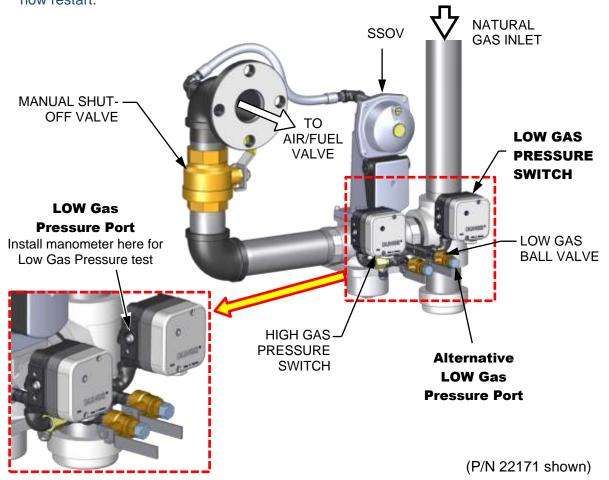
Figure 5-2: <u>BMK 3000</u> LOW and HIGH Gas Pressure Test Components
