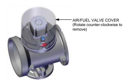
Figure 5-10b: Air/Fuel Valve Cover Location – BMK 750/1000
