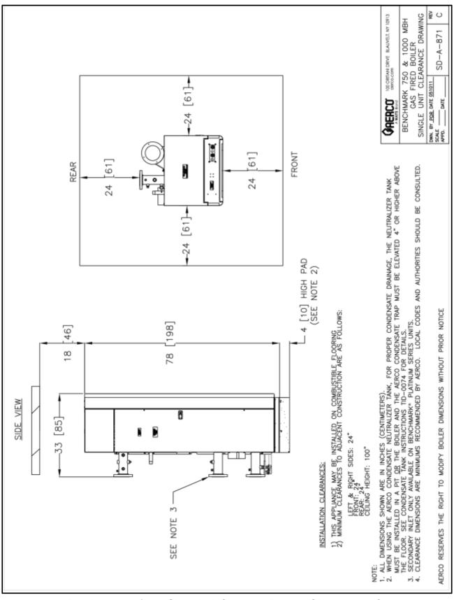
Benchmark 750/1000 Single Unit Clearance Drawing SD-A-871 rev C
