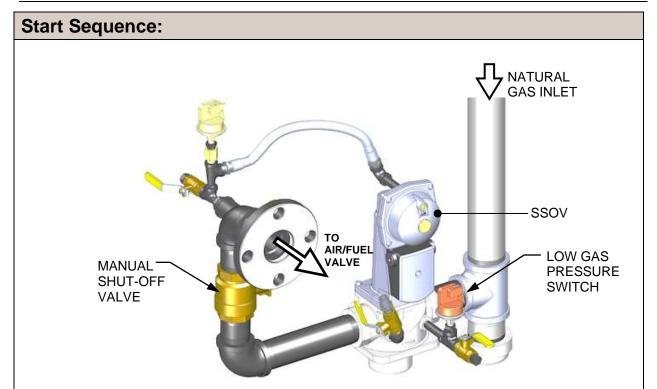
Figure 3-1c: BMK 2500: SSOV Location (P/N 22190 shown)
