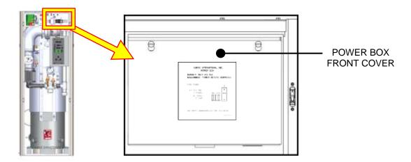
Figure 2-8b: BMK 1500/2000/2500/3000 Power Box with Closed Cover
