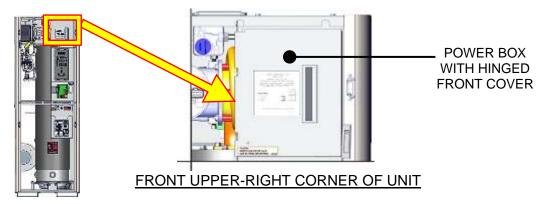
Figure 2-8a: BMK 750/1000 Power Box with Closed Cover
