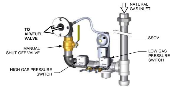
Figure 3-1d: BMK 3000: SSOV Location (P/N 22171 shown)
