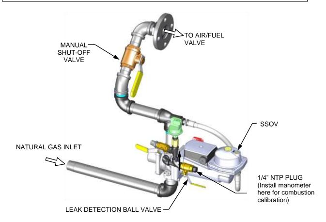
Figure 4-1a: BMK 750 & 1000 1/4 Inch Gas Plug Location (P/N 22140-1 shown)
