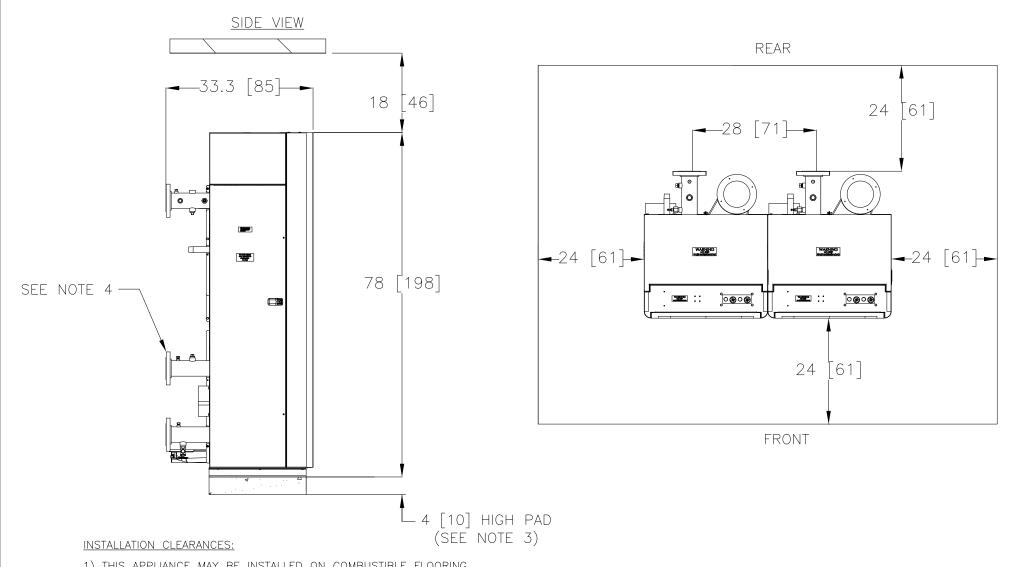
1) THIS APPLIANCE MAY BE INSTALLED ON COMBUSTIBLE FLOORING 2) MINIMUM CLEARANCES TO ADJACENT CONSTRUCTION ARE AS FOLLOWS:
