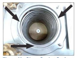
Figure M: Clean Gasket Surface
