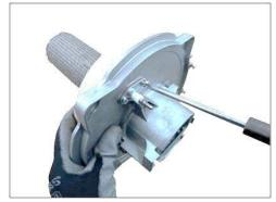
Figure L: Tighten the Electrodes
