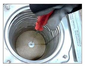
Figure D: Installing Thermal Insulation
