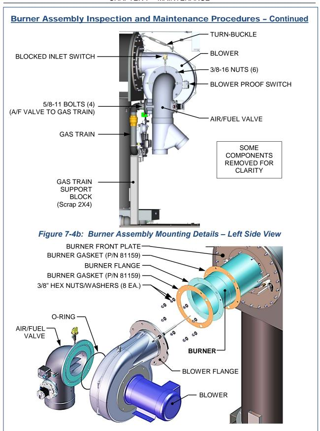
Figure 7-5: Burner Assembly – Exploded View
