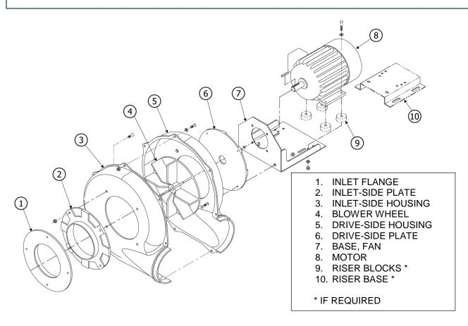
Figure L-1: Benchmark 6000 Blower Exploded View
