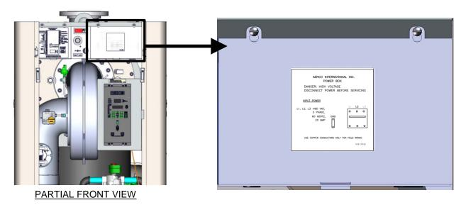
Figure 2-9. Power Box With Cover Closed (460V shown)
