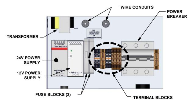
Figure 2-10. Power Box Internal Components (Cover Removed)
