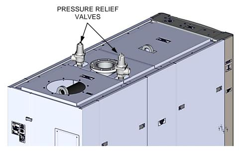
Figure 2-5A: Pressure Relief Valve Installation Locations
