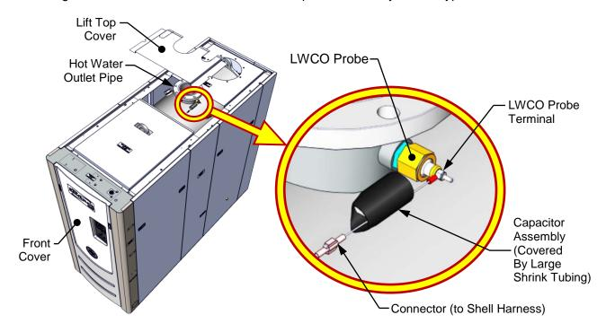
Figure 7-12: LWCO Probe Location for BMK6000
