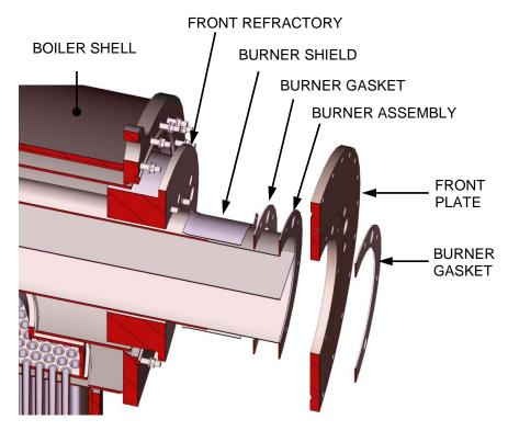
Figure 7-9b: Front Plate Assembly - Cut-Away View
