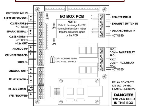
Figure 2-13. I/O Box Terminal Strips
