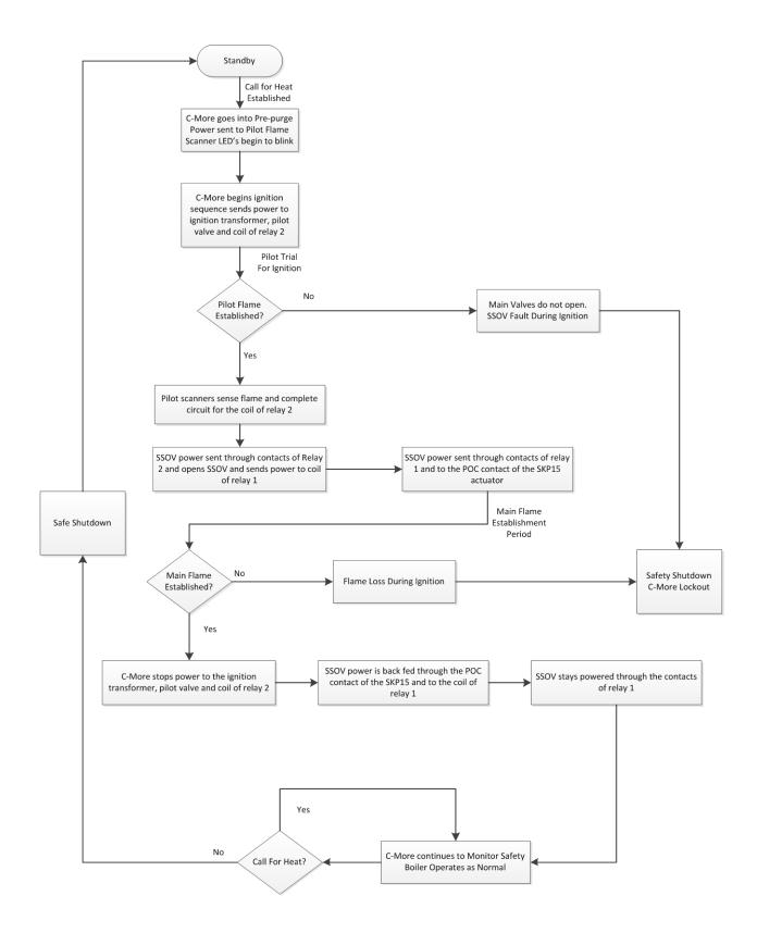
Figure 3-9: Burner Ignition Sequence Flowchart
