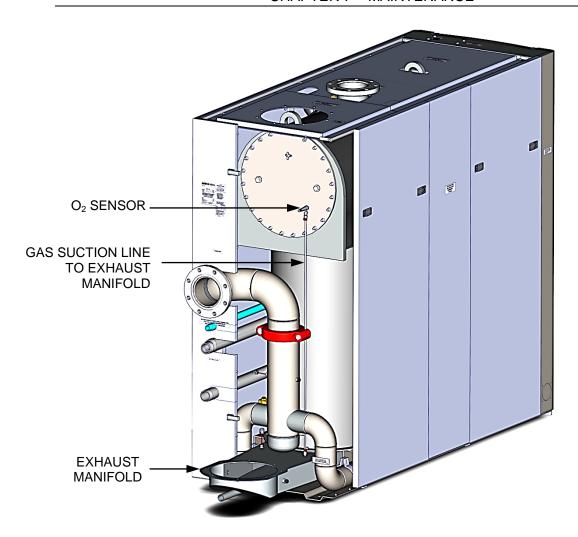
Figure 7-2. O<sub>2</sub> Sensor Mounting Location
