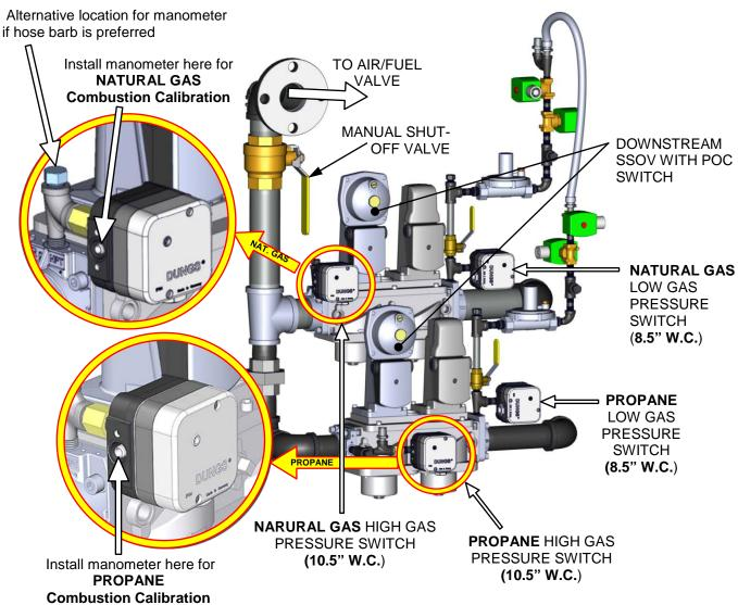
Figure 4-1: Port Locations for Combustion Calibration Measurements
