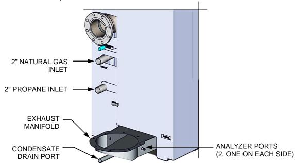
Figure 2-6. Partial Rear View - Condensate Drain Location
