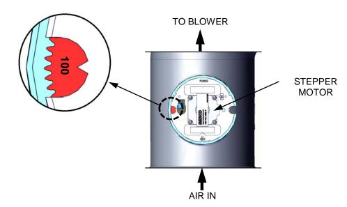
Figure 3-4: Air/Fuel Valve In Purge Position
