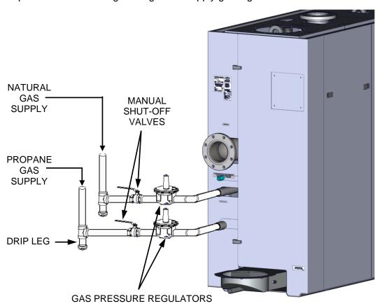
Figure 2-8. Manual Gas Shut-Off Valve Location
