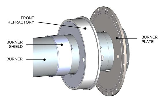
Figure 7-9a: Front Plate Assembly
