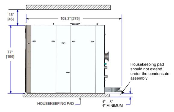
Figure 2-2a. Benchmark Boiler Model 6000 Clearances
