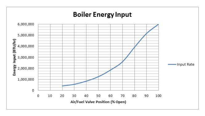
Figure 3-8: Relationship Between Air/Fuel Valve Position and Energy Input
