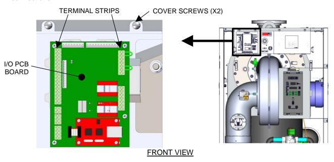
Figure 2-12. Input/Output (I/O) Box Location
