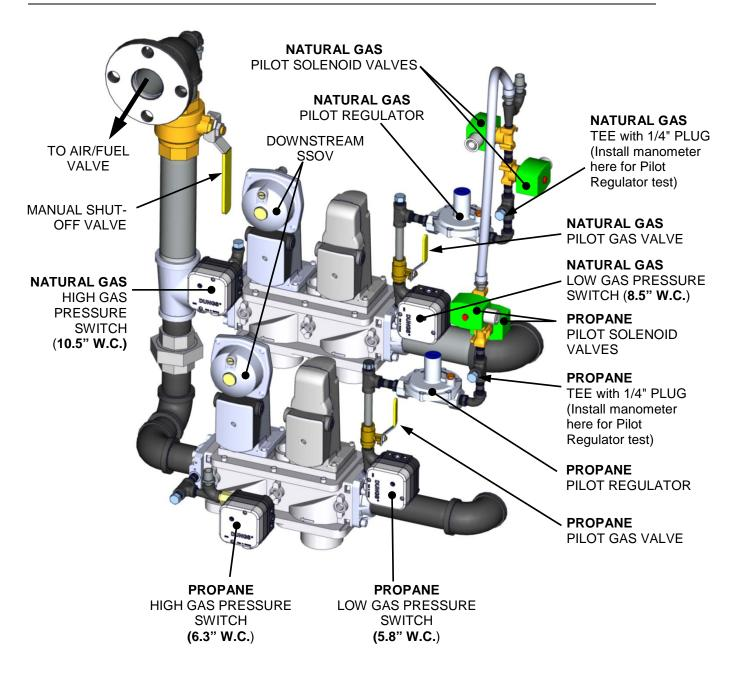
Figure 8-1: Gas Train Component and Pilot Gas Valve Location
