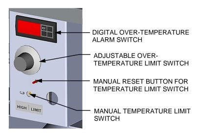
Figure 4-5: Over-Temperature Limit Switch Locations
