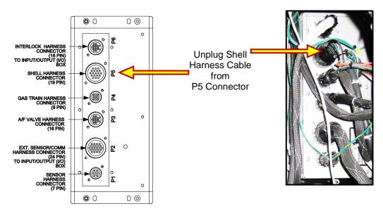
Figure 7-13: Removing Shell Harness Cable from P5 Conn. on C-More Rear Panel
