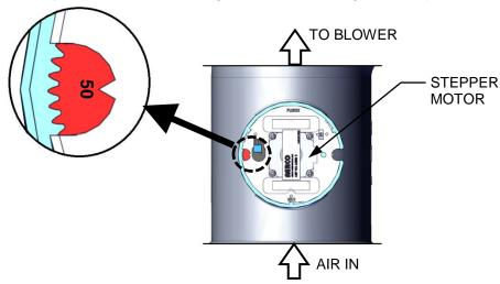
Figure 3-6: Air/Fuel Valve In Ignition Position
