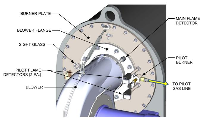
Figure 8-2: Pilot Burner & Flame Detector Locations
