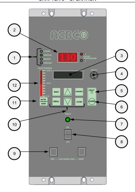
Figure 3-1: Control Panel Front View
