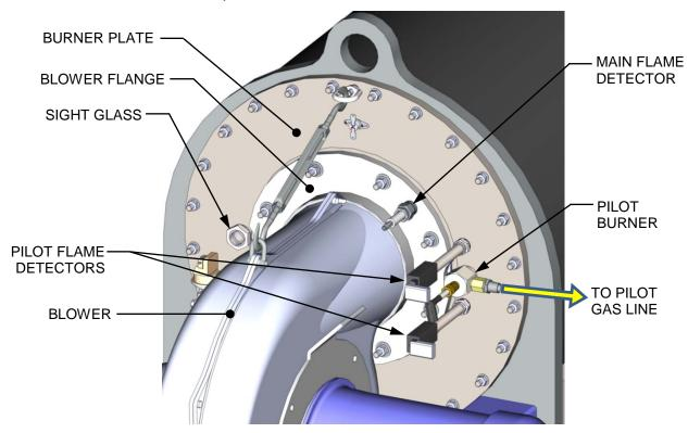
Figure 7-1: Pilot Burner, Main & Pilot Flame Detector Mounting Locations
