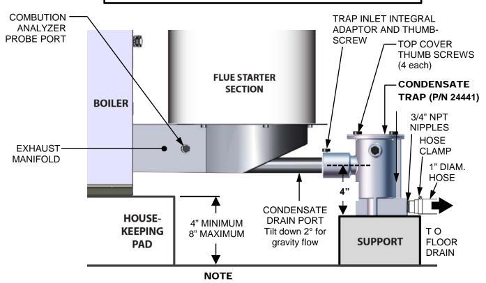
HOUSKEEPING PAD MUST NOT EXTEND UNDER THE CONDENSATE ASSEMBLY.
