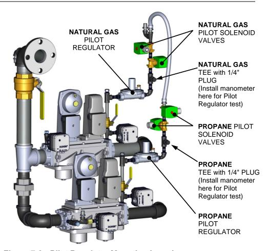
Figure 7-3: Pilot Regulator Mounting Location
