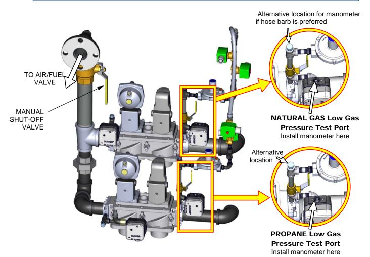
Figure 6-1A: Low Gas Pressure Switch Locations & Test Ports
