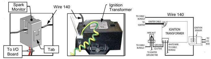
Figure 7-15: Spark Detector Sensor (AC Current Transducer) P/N 61034
