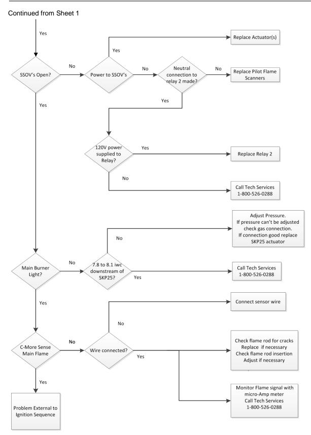
Figure 8-4: Pilot Assembly Troubleshooting Flow Chart (Sheet 2 of 2)
