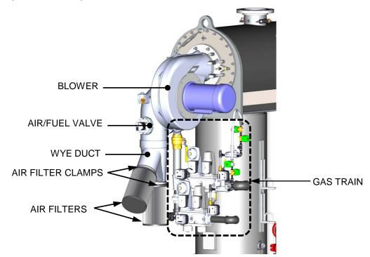
Figure 7-11: Air Filter Location and Removal
