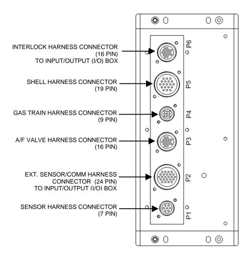
Figure J-2: Benchmark Control Panel Rear View
