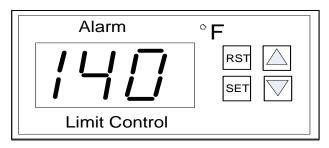
Figure 4-6: Digital Over-Temperature Alarm Switch Front Panel
