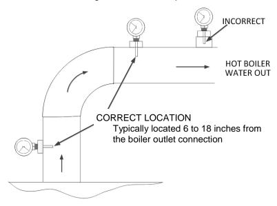
Figure 2-5B. Pressure/Temperature Gauge Installation Location
