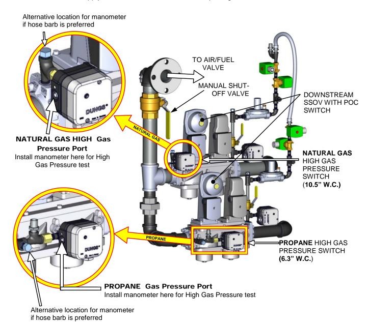
Figure 6-1B: High Gas Pressure Switch Locations & Test Ports
