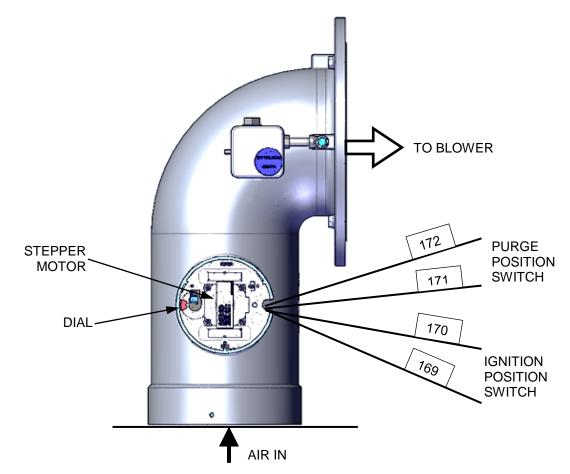
Figure 6-9: Air/Fuel Valve Purge and Ignition Switch Locations
