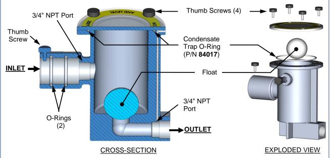
Figure 7-10: External Condensate Trap: Cross-Section & Exploded View
