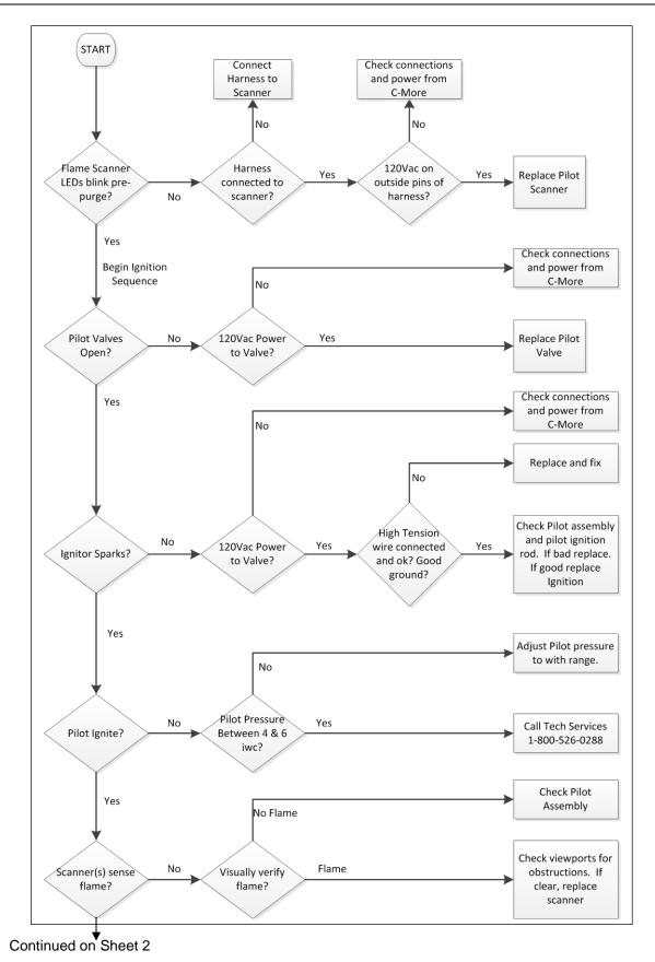
Figure 8-4: Pilot Assembly Troubleshooting Flow Chart (Sheet 1 of 2)
