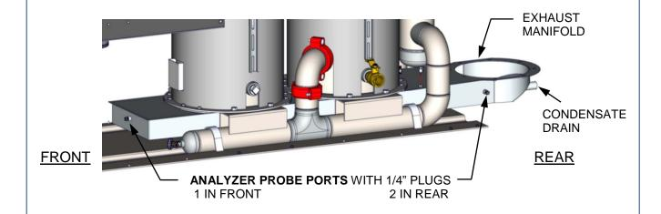
Figure 4-2: Analyzer Probe Hole Location
