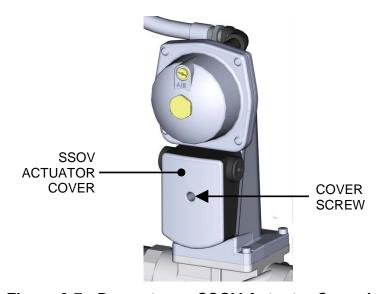
Figure 6-7: Downstream SSOV Actuator Cover Location
