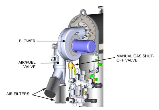
Figure 6-4: Bare Boiler – Partial View
