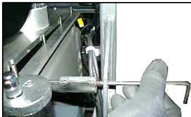
Figure 8-14: Unscrewing Lift Screw into Tab Hole (Step 10)
