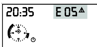
Figure 4-25: “Loss of Flame” FaultCode (E 05)
