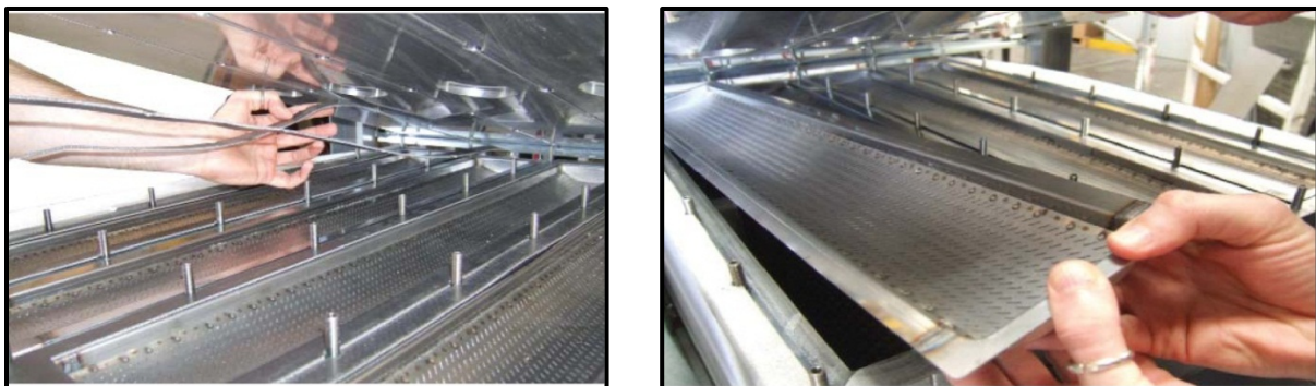
Figure 8-17: Exposing Burner Modules (Left) and Removing (Right)
