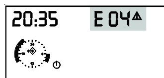
Figure 4-26: “No Flame Detected During Ignition” Fault Code (E 04)
