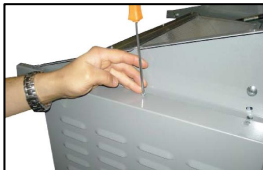
Figure 8-5: Remove Screws at Edges and Remove Side and Rear Panels (Step 3)
