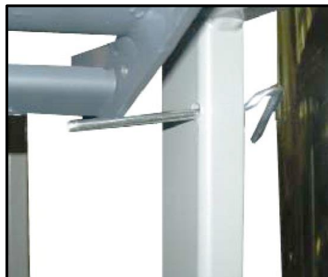
Figure 8-22: Lift Pins Inserted into Lift Holes, Left and Right Sides (Step 15)
