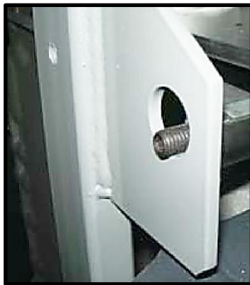
Figure 8-19: Lift Screws Extended into Tab Holes, Left and Right Sides (Step 14)
