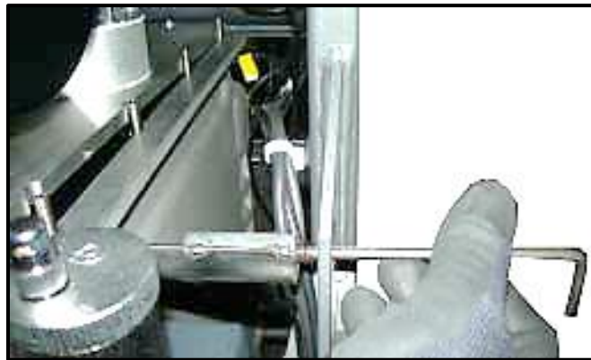
Figure 8-18: Unscrewing Lift Screw into Tab Hole (Step 14)
