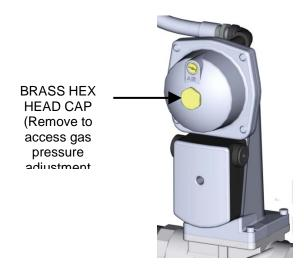
Figure 4-4. Gas Pressure Adjustment Screw Location
