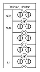
Figure 2-10. AC Terminal Block Configurations
