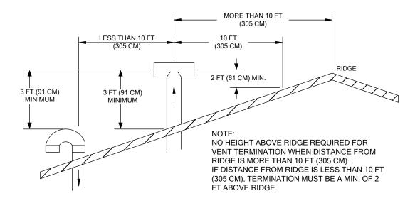
Figure 4. Roof-Mounted Combustion Air Inlet & Vent Outlet Installations
