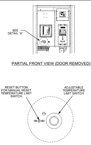
Figure 5-2. Temperature Limit Switch Setting
