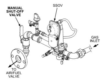
Figure 5-3. Manual Gas Shut-Off Valve Location
