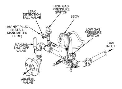
Figure 4-1. 1/8 Inch Gas Plug Location
