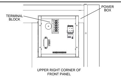
Figure 2. Terminal Block Location
