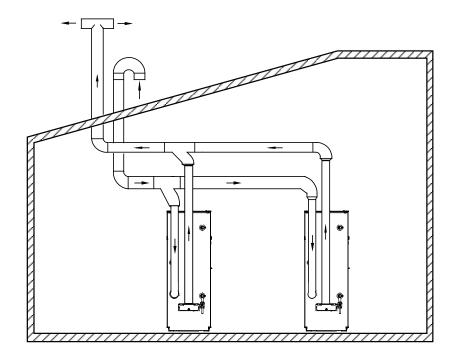
Figure 6. Roof-Mounted Combustion Air Inlet & Vent Installation
