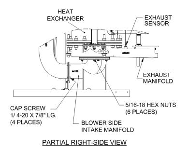
Figure 6-3. Blower-Side Intake Manifold & Exhaust Manifold Locations
