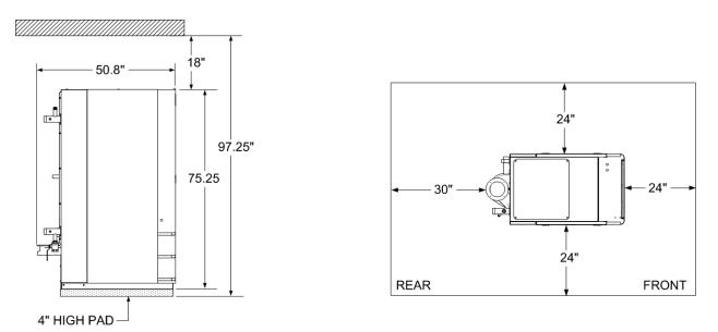
Figure 2-1 Innovation Water Heater Clearances
