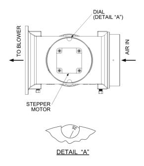
Figure 3-6. Air/Fuel Valve In Ignition Position
