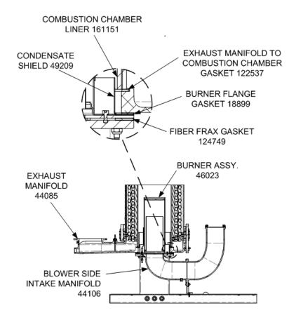
Figure 6-6. Combustion Chamber Liner & Gasket Locations
