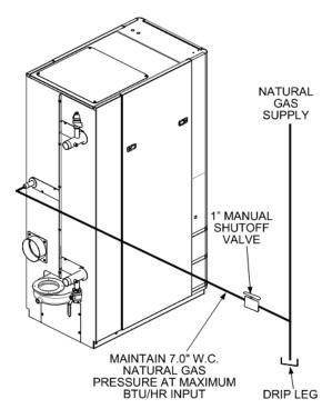
**Diagram 1. Single Heater Pipe Connections**
