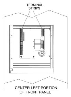
Figure 2-11. Input/Output (I/O) Box Location
