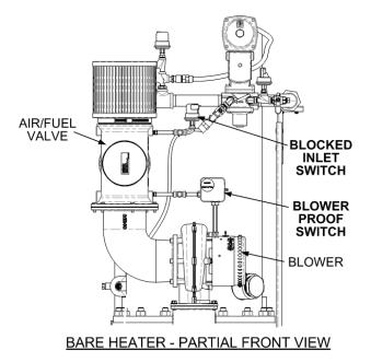
Figure 5-4. Blower Proof & Blocked Inlet Switch Locations
