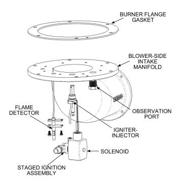
Figure 6-1. Blower-Side intake Manifold (Shown Removed from Heater)
