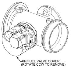
Figure 5-7. Typical Air/Fuel Valve Cover Location
