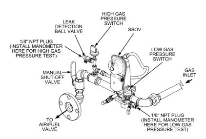
Figure 5-1. Low & High Gas Pressure Testing
