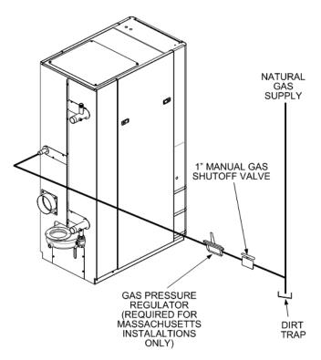
Figure 2-8. Manual Gas Shut-Off Valve Location
