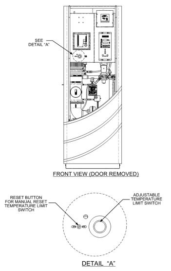
Figure 4-4. Over Temperature Limit Switch Location
