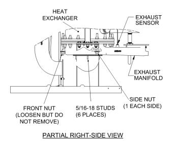
Figure 6-5. Innovation Heater – Partial Cut-Away View
