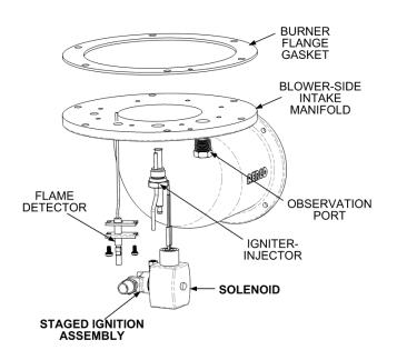
Figure 7-2. Blower-Side Intake Manifold (Shown removed from Heater)
