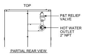
Figure 2-5. P&T Relief Valve Location
