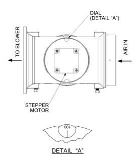
Figure 3-4. Air/Fuel Valve In Purge Position
