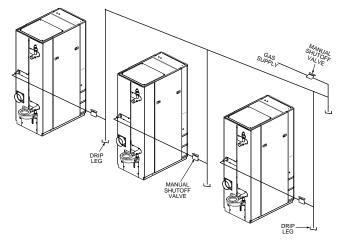
Diagram 3 Typical Multiple Heater Manifold Construction
