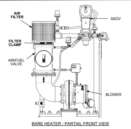
Figure 6-10. Air Filter Mounting Location
