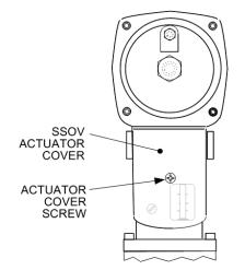
Figure 5-6. SSOV Actuator Cover Location
