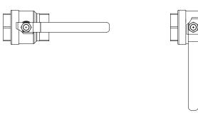
Figure 1-1. Manual Gas Shutoff Valve
