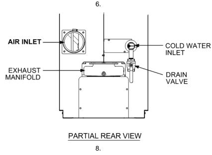
Figure 5-5. Water Heater Rear View Showing Air Inlet Location
