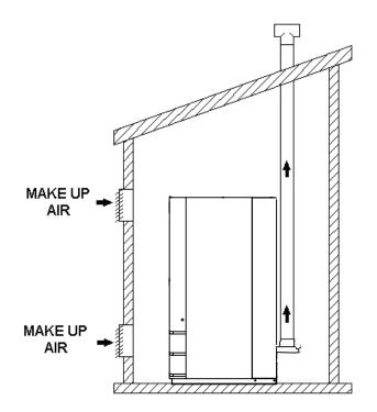
Figure 2. Combustion Air From Outside the building
