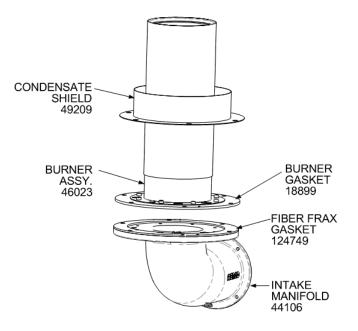
Figure 6-4. Innovation Heater – Partial Left-Side View
