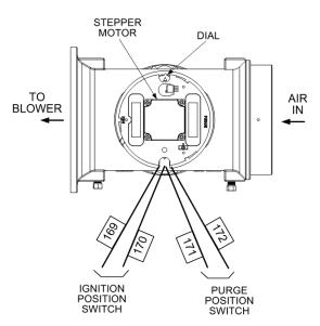
Figure 5-8. Air/Fuel Valve Purge and Ignition Switch Locations
