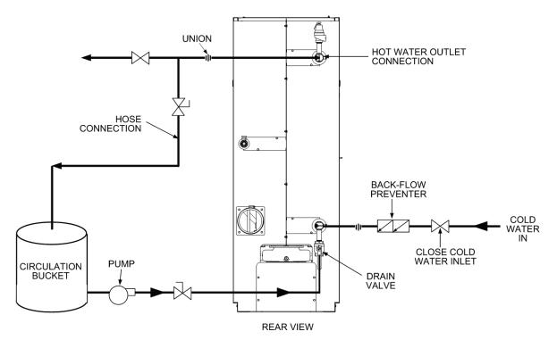
Figure 6-8. Sample Heat Exchanger Cleaning Set-Up
