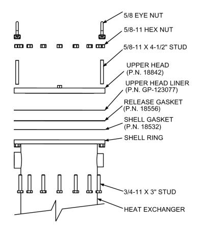
Figure 6-7. Flat Style Head Configuration
