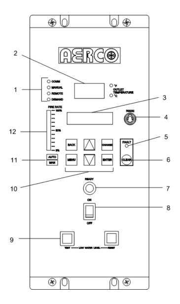
Figure 3-1. Control Panel Front View
