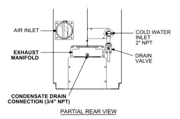
Figure 2-6. Condensate Drain Connection Location
