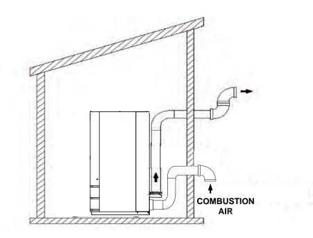
Figure 5. Wall-Mounted Combustion Air Inlet & Vent Outlet Installations
