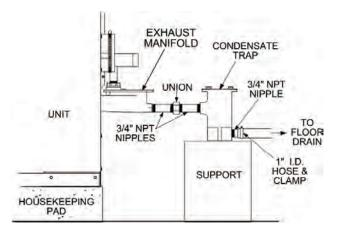
Figure 2-7. Sample Condensate Trap Installation
