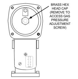
TYPICAL SSOV ACTUATOR WITH REGULATOR
