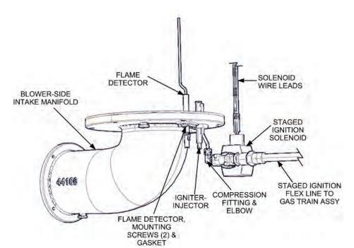
Figure 6-2. Igniter-Injector & Flame Detector Mounting Details
