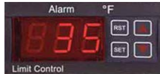
Figure 8-11a. Over-Temperature Switch & Temperature Indicator
