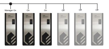
efficient firing rate. Importantly, because the BST reacts in real-time to, up to 8 boilers, changes in the number of boilers available, users can take a unit offline for maintenance at any time or bring on back-up boilers for extremely cold conditions without changes to the BST. And as individual boilers are added or deleted, the energy delivered is automatically adjusted to prevent fluctuations in the header temperature of the plant.
