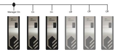
efficient firing rate. Importantly, because the BST reacts in real-time to, up to 16 boilers, changes in the number of boilers available, users can take a unit offline for maintenance at any time or bring on back-up boilers for extremely cold conditions without changes to the BST. And as individual boilers are added or deleted, the energy delivered is automatically adjusted to prevent fluctuations in the header temperature of the plant.
