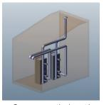
Common vertical vent/ individual sidewall air
