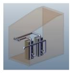
Individual sidewall vent/ common sidewall air
