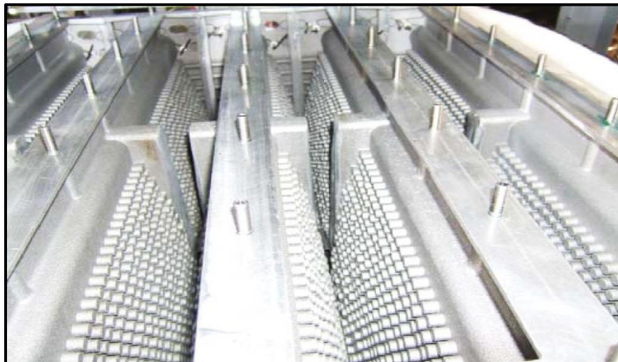
Figure 8-18: Exposed Combustion Chambers under Burner Modules
