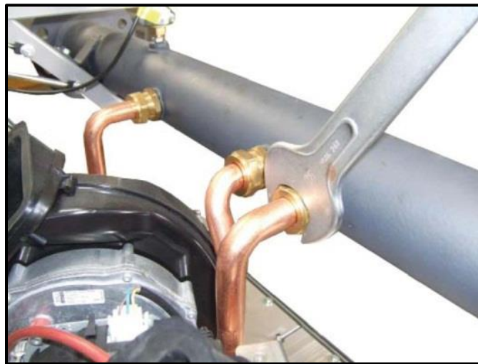
Figure 8-12: Removing the Gas Pipes from Gas Manifold (Step 8)
