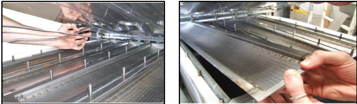
Figure 8-17: Exposing Burner Modules (Left) and Removing (Right)
