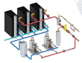
mon of older mechanical plants run by either large built-in-place cast iron or Scotch-Marine boilers, there is a significant weakness in this type of system that cannot be ignored. When a unit is brought offline, either for reactive service or preventive maintenance, the building will be completely without a heat source. For this reason, modern boiler plants typically consist of multiple smaller units.
