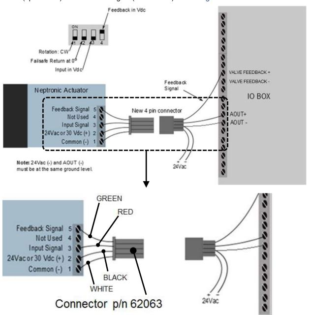
Figure 8.10.2: Sequencing Valve Wiring
