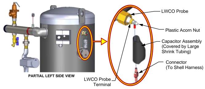
Figure 6.11: LWCO Probe Location (INN 1350 Shown)
