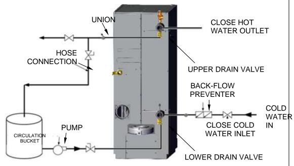
Figure 6.8.3.1: Sample Heat Exchanger Cleaning Set-Up
