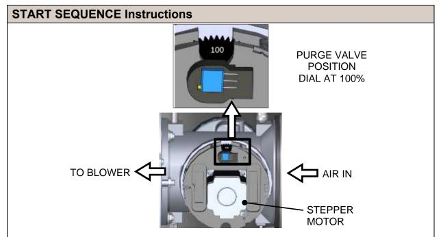
Figure 3.4-2: Air/Fuel Valve in Purge Position
