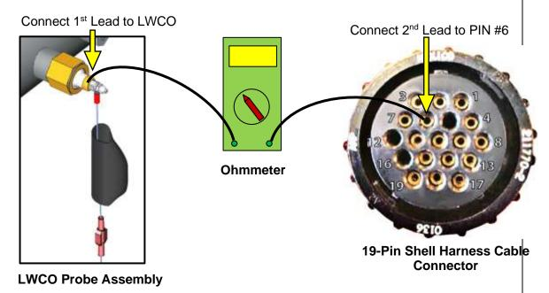
Figure 6.11.1-2: Connecting Ohmmeter – LWCO Probe & Shell Harness Cable
