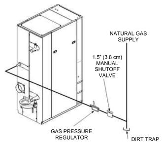
Figure 2.10.3.2: Manual Gas Shut-Off Valve Location
