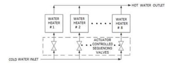
Figure 8.1: Simplified Block Diagram - Water Heater Management (WHM)
