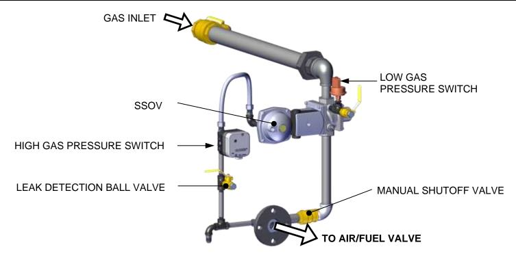
Figure 7.2-1: Innovation Gas Train Component Locations (600N & 800N P/N 22332 shown)
