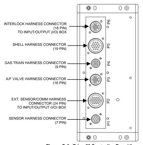
Figure G-2: Edge [i] Controller Rear View
