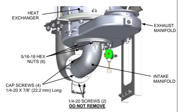
PARTIAL RIGHT-SIDE VIEW – BASE & SUPPORT BRACKET REMOVED FOR CLARITY
