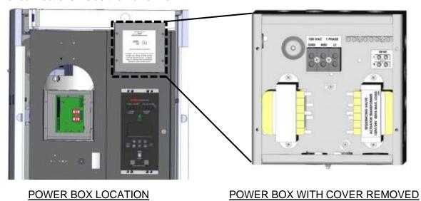
Figure 2.11-1: Power Box Location - Partial Front View, Front Panel Removed
