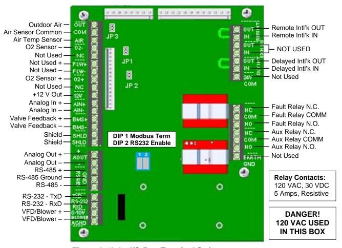
Figure 2.12-2: I/O Box Terminal Strips
