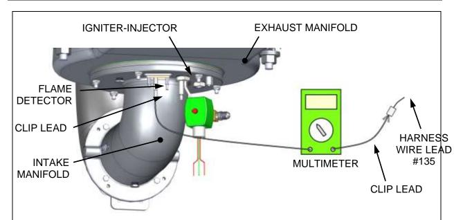
Figure 4.2.4: Flame Strength Set-Up Using Multimeter – Rear View
