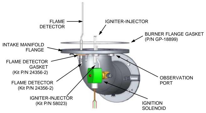
Figure 6.3-1: Intake Manifold with Igniter-Injector & Flame Detector
