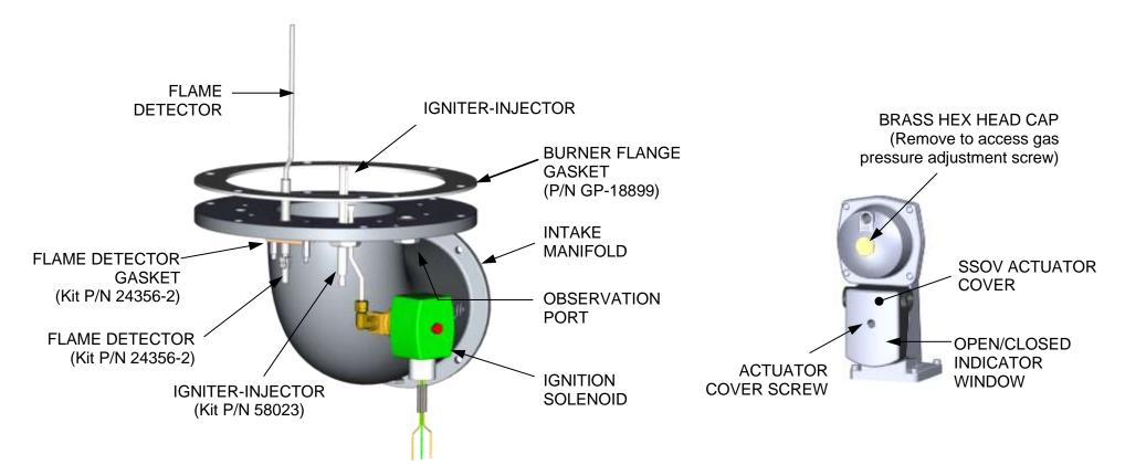
Figure 7.2-2: Intake Manifold
