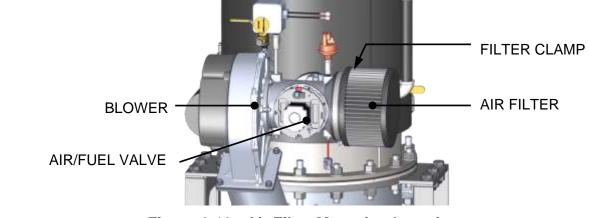
Figure 6.10: Air Filter Mounting Location
