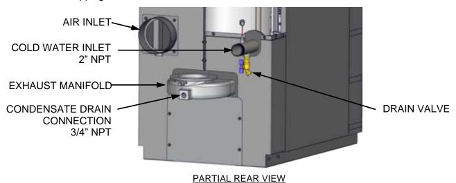
Figure 2.9-1: Condensate Drain Connection Location
