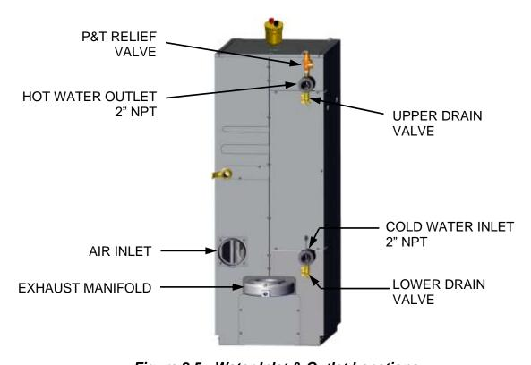
Figure 2.5: Water Inlet & Outlet Locations
