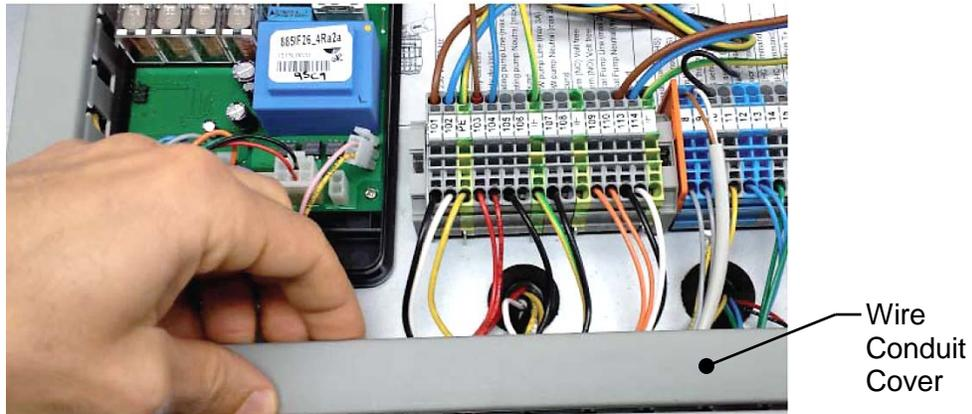
**Figure 1-9: Opening the Wire Conduit Cover**
