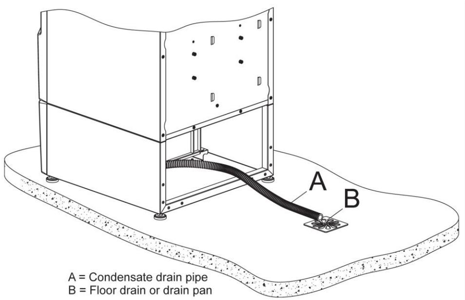
**Figure 8: Typical Condensate Drain Installation**
