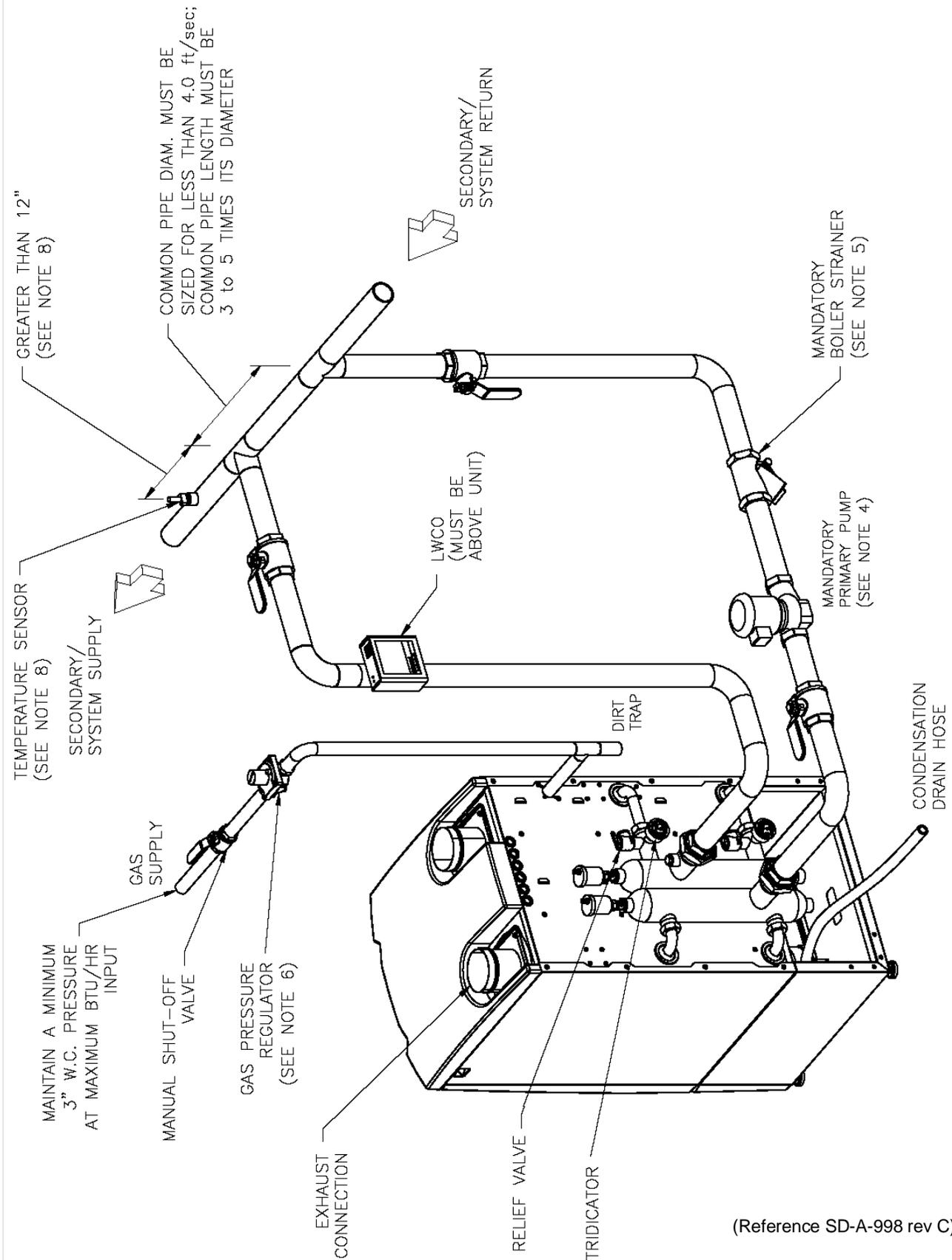
Figure 10: AM 399/500 Single Unit Installation
