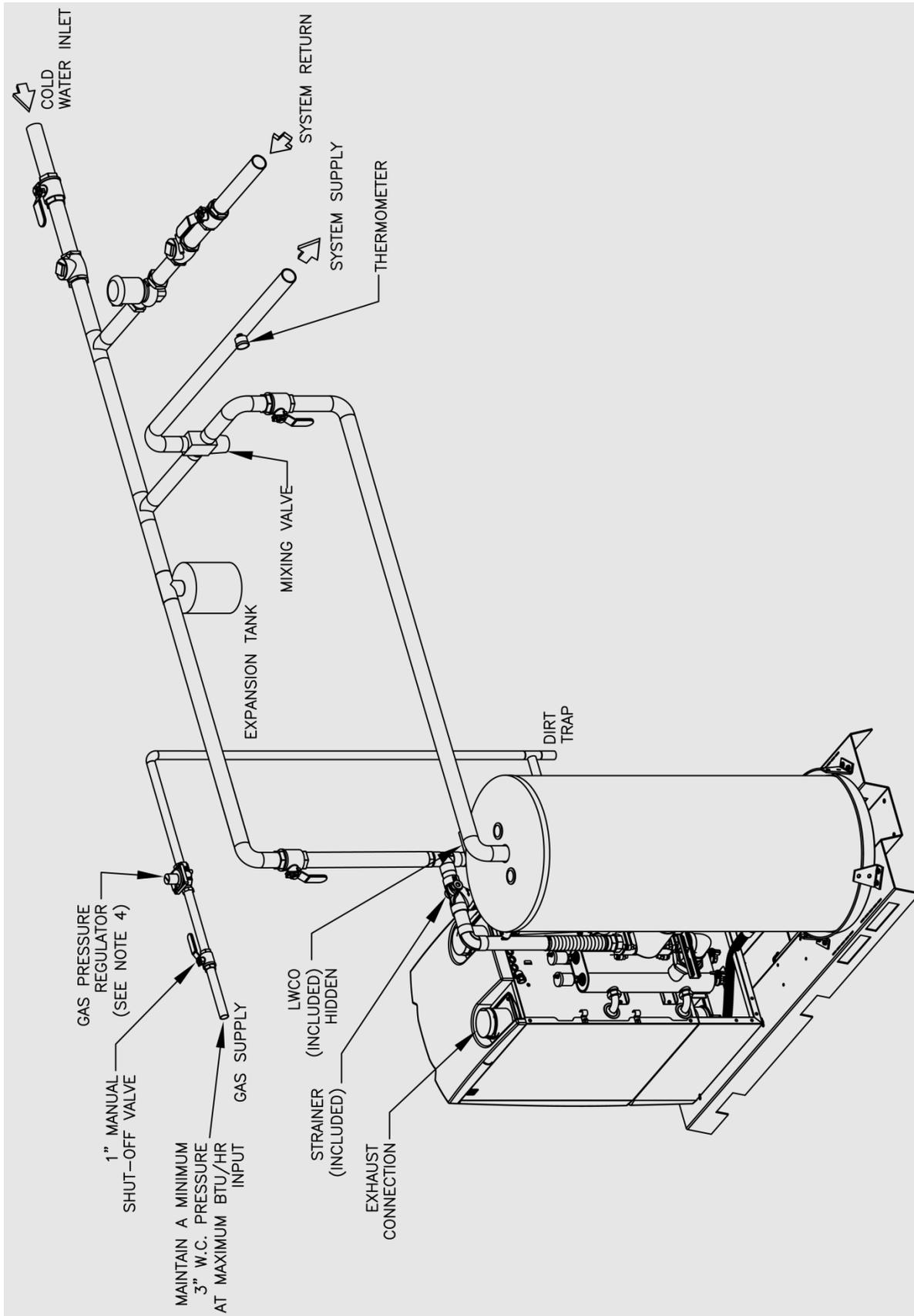
Figure 19: AM Series 399R/500R, Single Unit Installation
