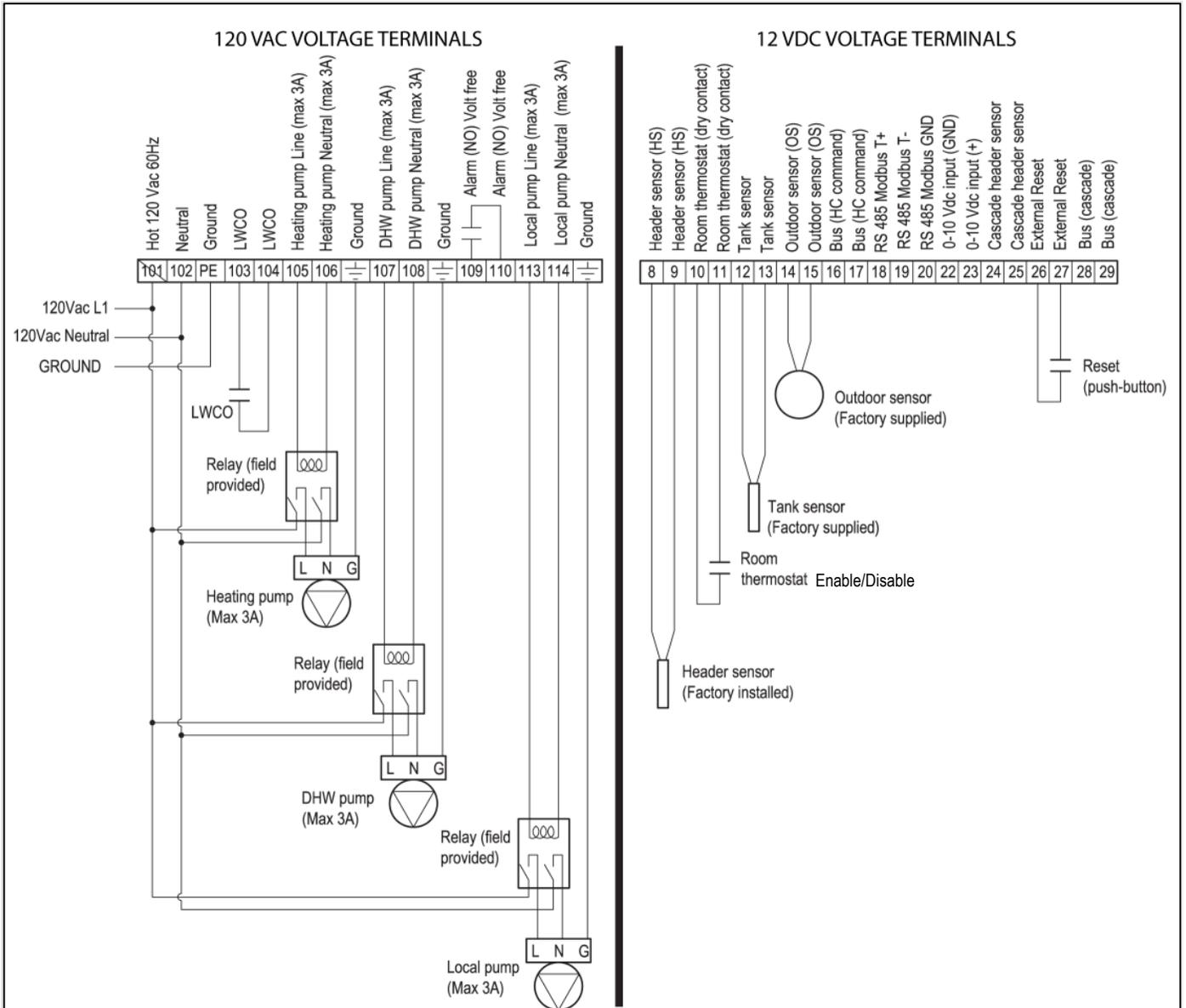
Figure 4: AM BOILER: Electrical Connections
