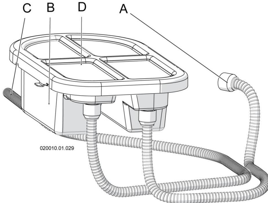
**Figure 9: Condensate Drain Assembly Components**
