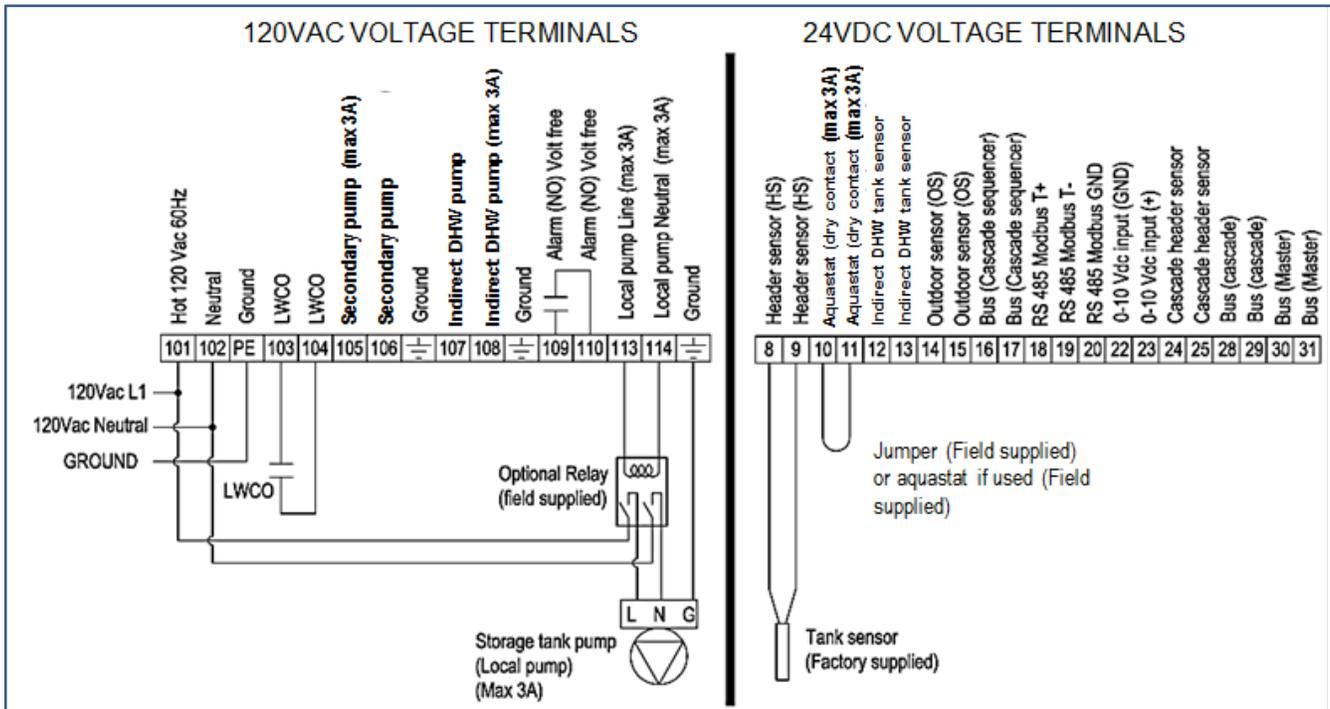
Figure 5: Water Heater Electrical Box Connections
