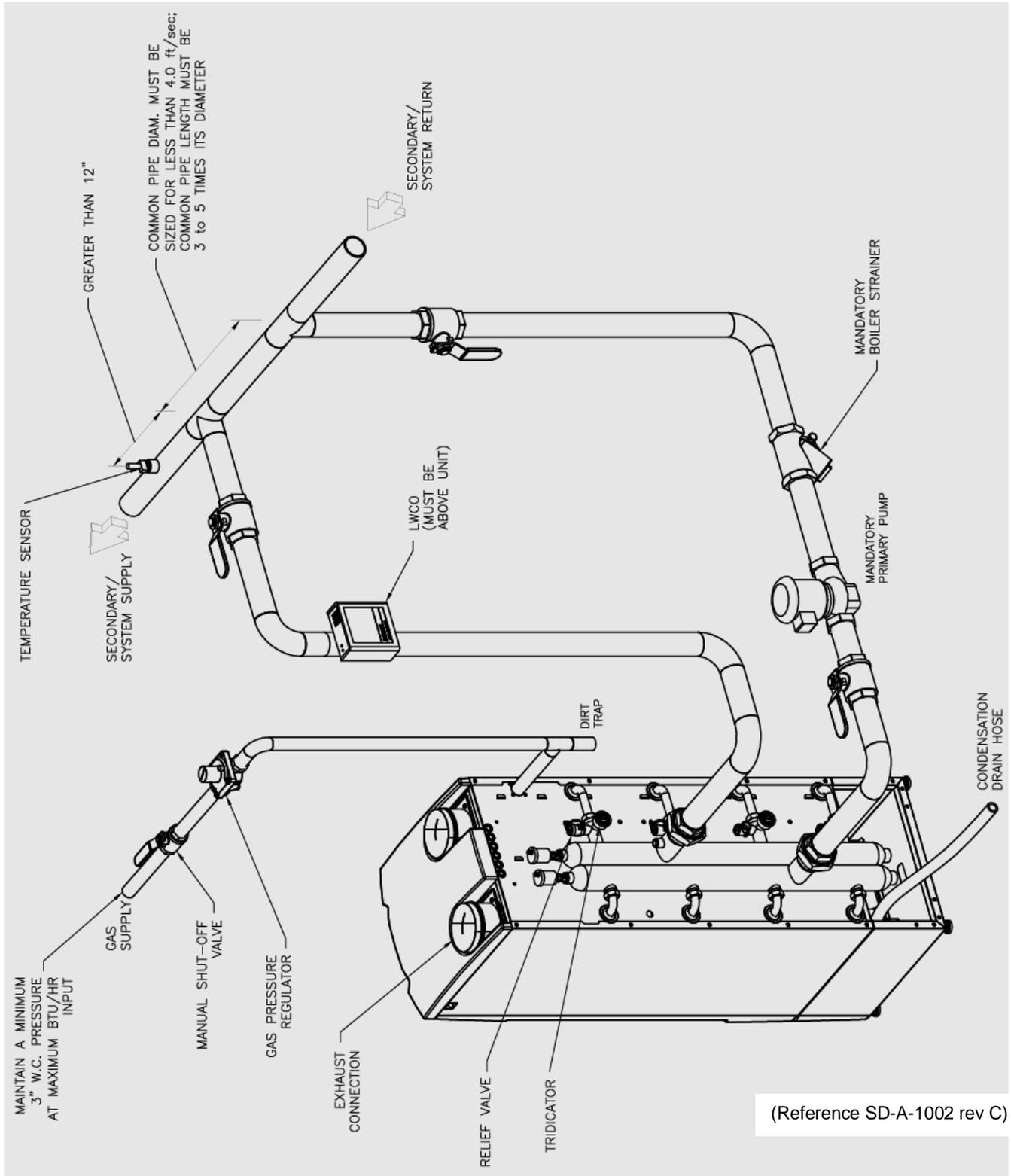
Figure 14: AM 750/1000 Single Unit Installation
