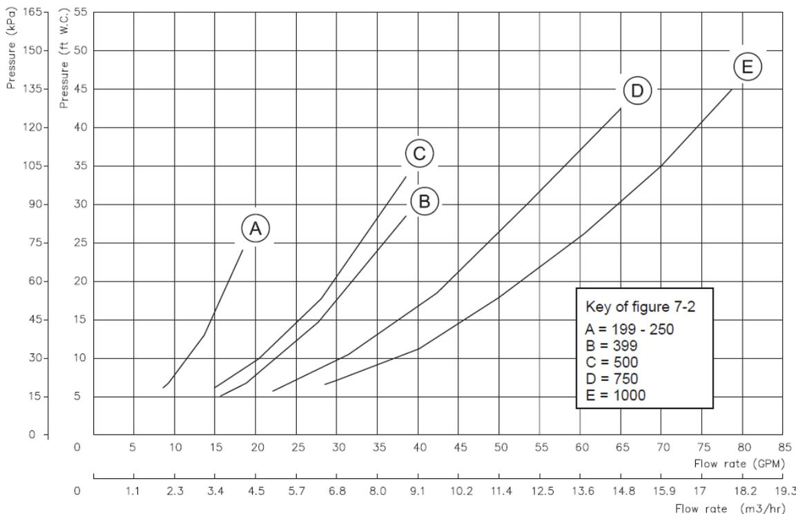
**Figure 2: Water Side Pressure Loss Chart**
