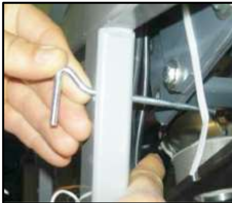
Figure 8-22: Lift Pins Inserted into Lift Holes, Left and Right Sides (Step 17)
