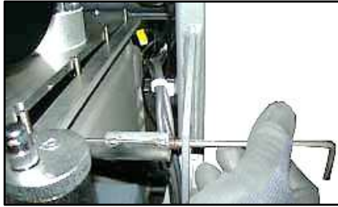
Figure 8-18: Unscrewing Lift Screw into Tab Hole (Step 14)
