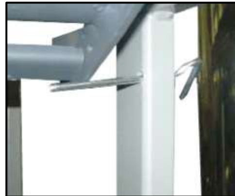
Figure 8-22: Lift Pins Inserted into Lift Holes, Left and Right Sides (Step 17)
