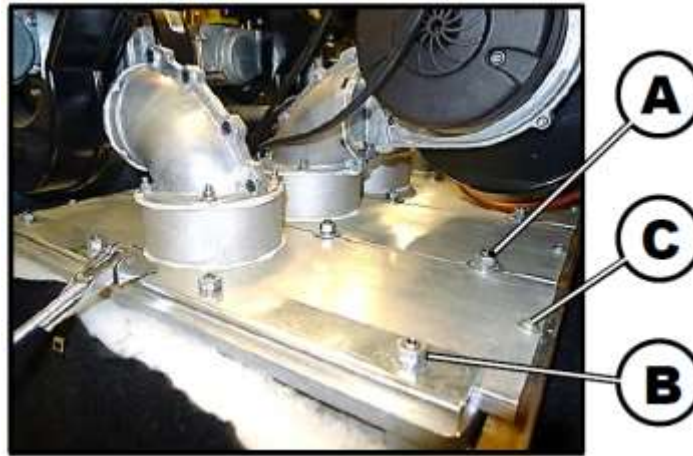
Figure 8-14: Removal of Burner Plate Hardware (Steps 9, 10, 11)
