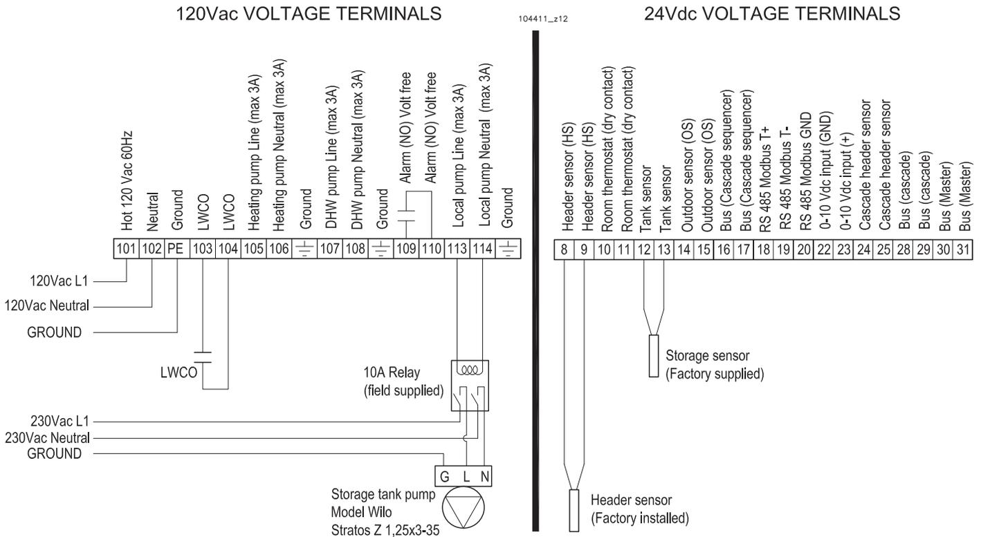
**Figure 10-3 Electrical customer connection for pump brand Wilo model Stratos Z1,25X3-35**
