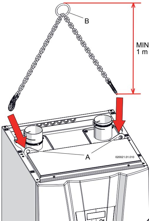
Figure 6-4 Correct way to lift the appliance
