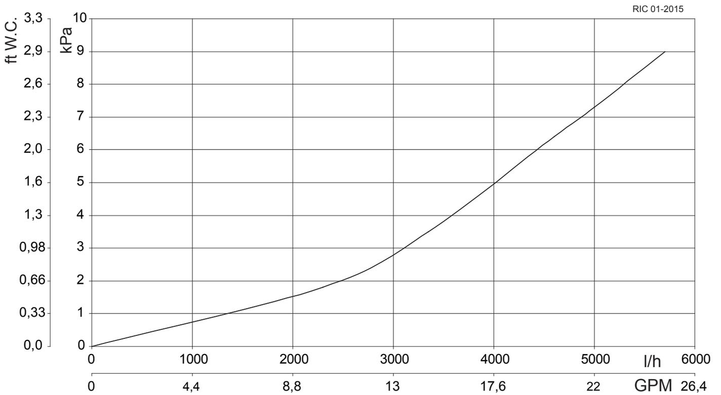
Figure 7-1 Water side head loss of the heater
