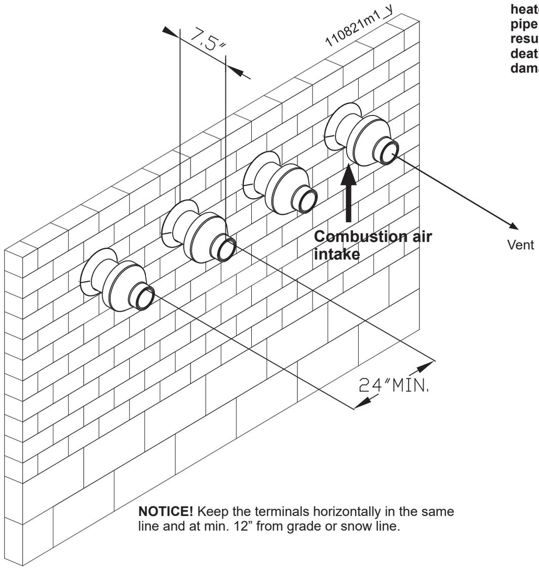
Figure 12-20 Concentric sidewall multiple heaters terminations
