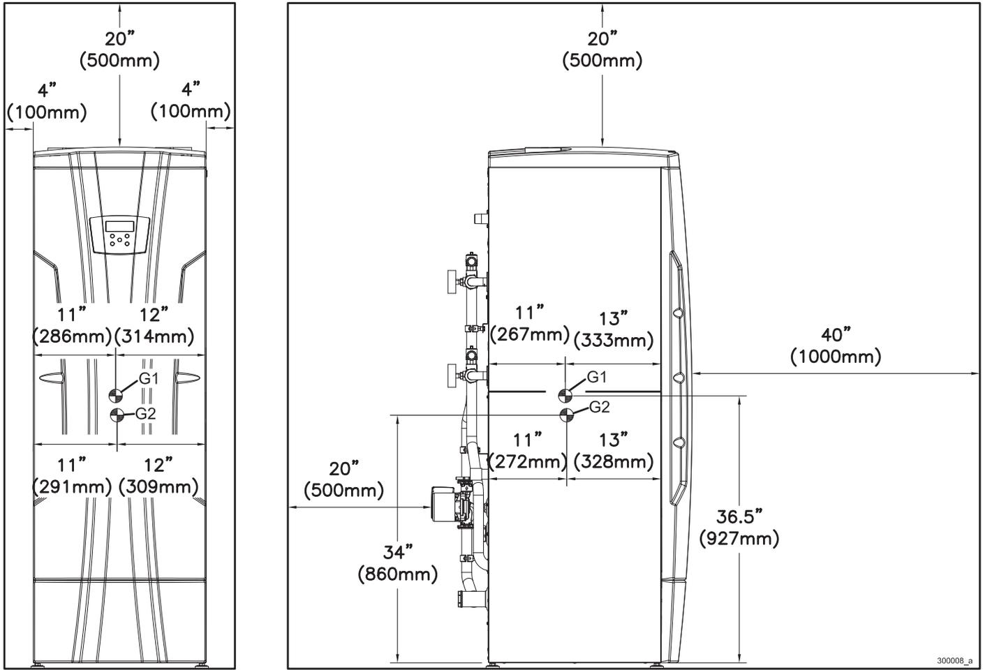
**Figure 5-6 Recommended minimum clearance distances for proper installation and servicing for models 199 to 500 (G1 = Center of gravity for 199 and 250 model G2 = Center of gravity for 399 and 500 model)**
