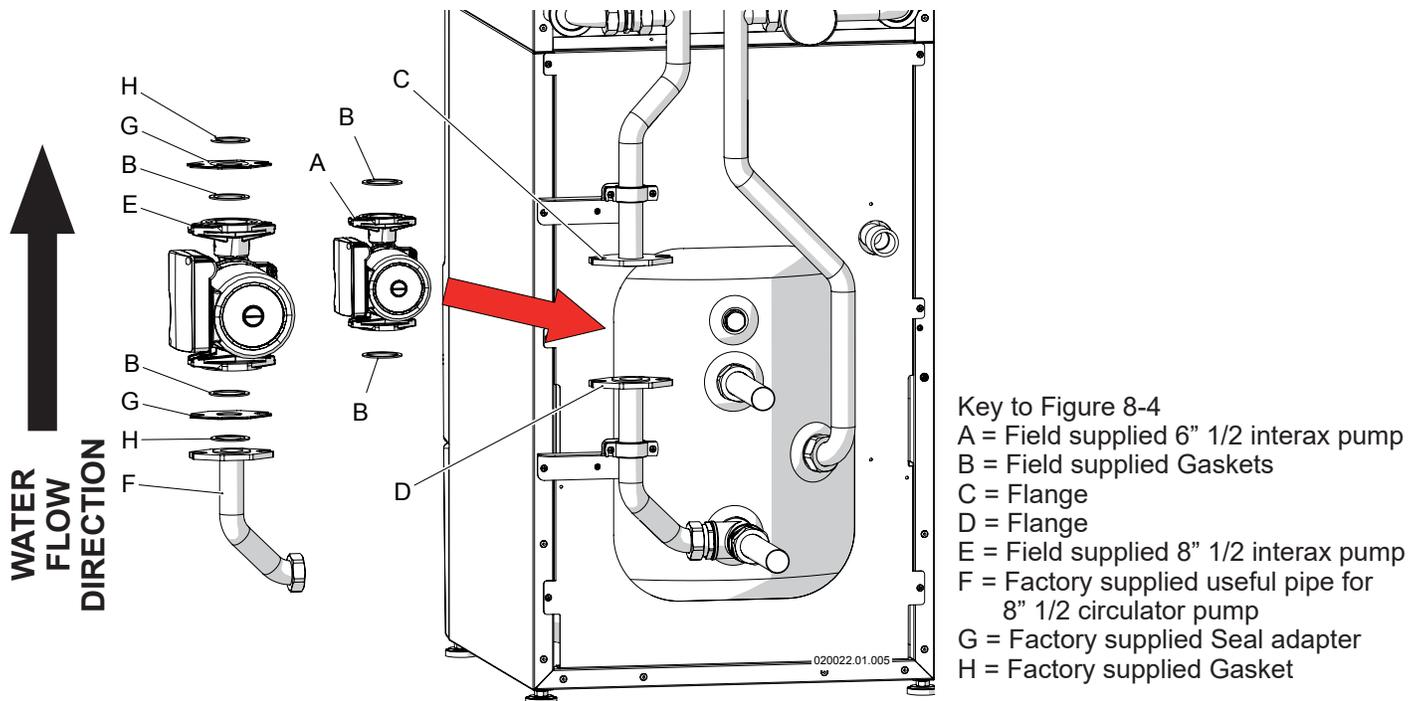
**Figure 8-4 Circulator pump installation**
