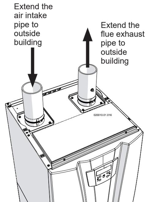
**Figure 12-13 Polypropylene air intake/vent connection correctly in place**
