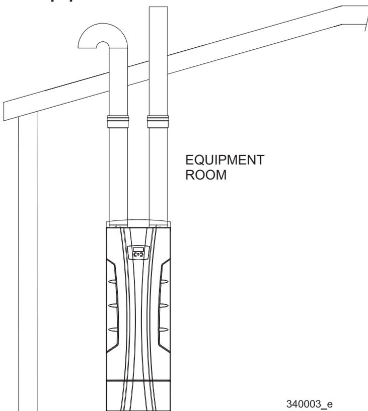
**Figure 13-3 Vertical direct vent installation with rooftop combustion air inlet**
