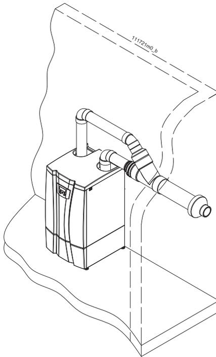
**Figure 12-4 Side wall concentric (Direct venting).**
