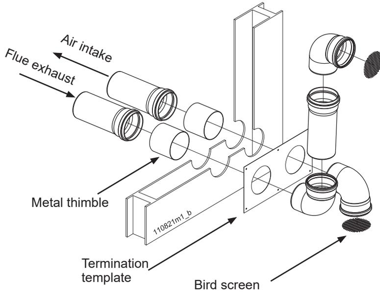
**Figure 12-16 Two pipes sidewall termination assembly**
