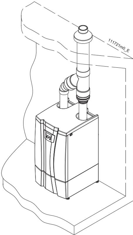
**Figure 12-3 Vertical concentric (Direct venting).**
