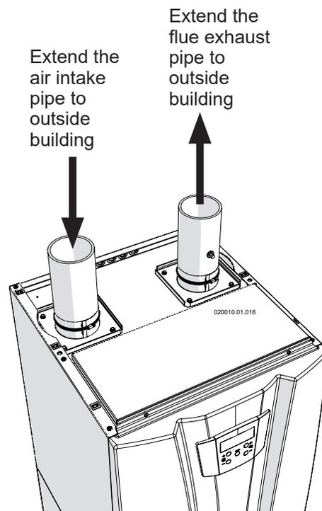
Figure 12-9 PVC/CPVC air intake/Vent connection correctly in place
