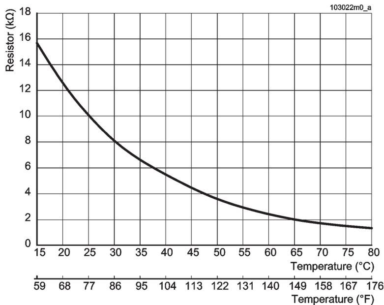
**Figure 17-14 Water and flue temperature sensors' curve**
