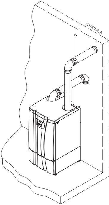
**Figure 12-1 Side wall two pipes (Direct venting).**
