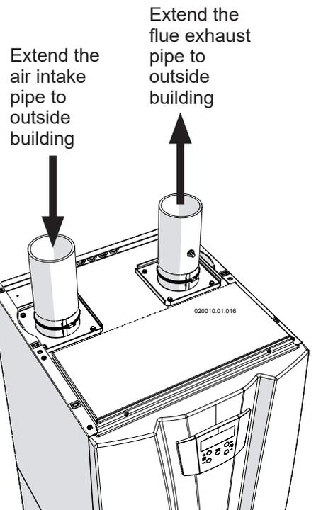
**Figure 12-11 Stainless steel air intake/vent connection correctly in place**
