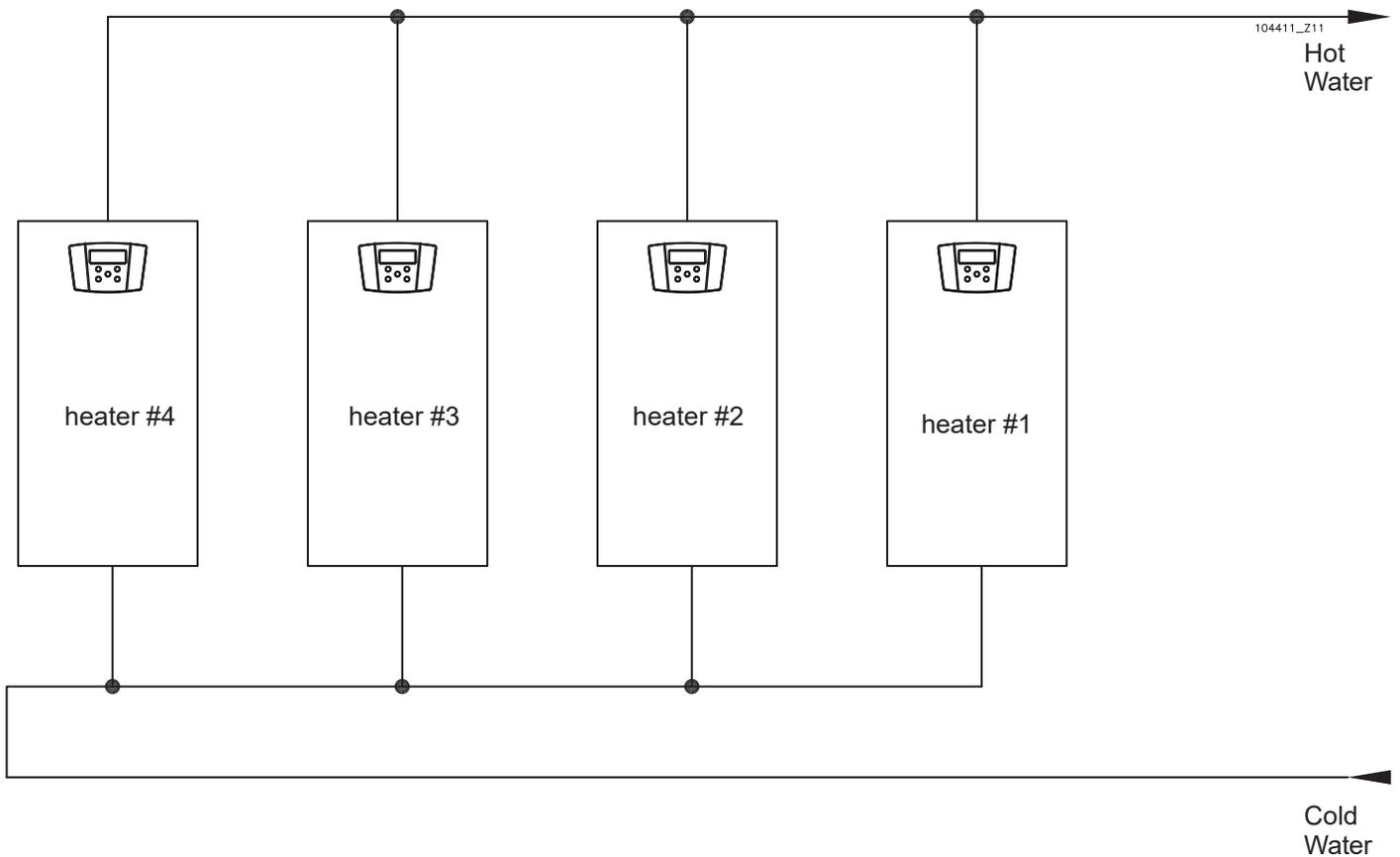
Figure 10-4 Multiple water heaters conceptual scheme
