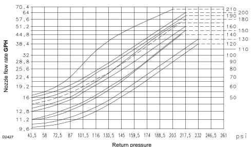
The values indicated in the right side of the diagram (Fig. 21), refer to the data printed on the nozzle.
