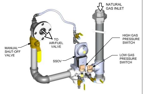
Figure 3-1b: BMK 1500 & 2000 SSOV Location (P/N 22188 shown)
