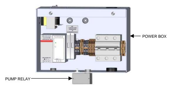
Figure 2-13b: BMK 1500/2000/2500-3000 Pump Relay Location (BMK 25000/3000 Shown)
