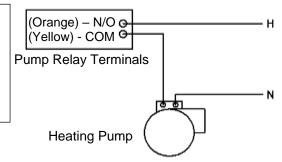
Figure 2-14: Schematic – System Pump Start using Boiler Pump Relay
