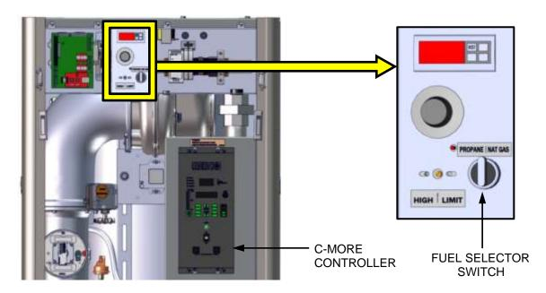
PARTIAL FRONT VIEW WITH FRONT COVER REMOVED
