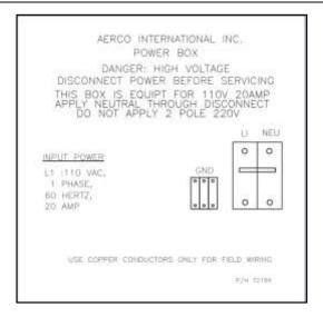
Figure 2-8a: Power Box Cover Label – BMK 750 – 2000
