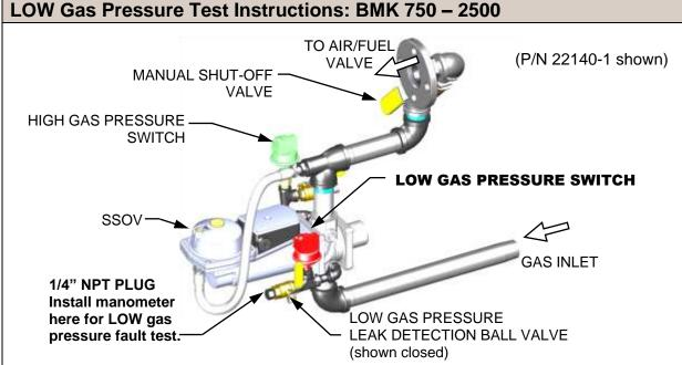
Figure 5-1a: <u>BMK 750/1000</u> LOW Gas Pressure Test Components
