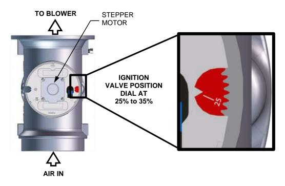
Figure 3-4: Air/Fuel Valve In Ignition Position
