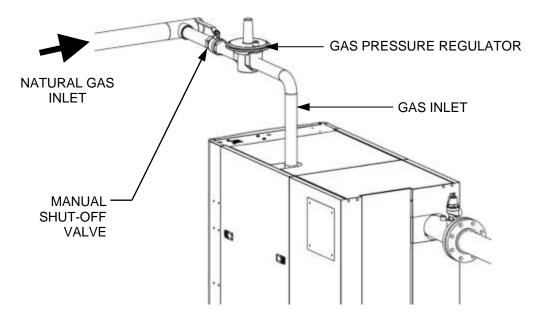
Figure 2-7b: BMK 1500-3000 Manual Gas Shut-Off Valve and Gas Regulator
