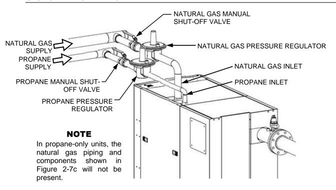
Figure 2-7c: BMK 1500-3000DF Dual Fuel Manual Gas Shut-Off Valve & Gas Regulator
