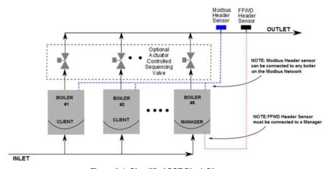
Figure 6-1: Simplified BST Block Diagram
