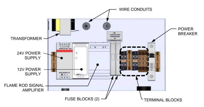
Figure 2-10b: BMK 1500/2000 Power Box Internal Components
