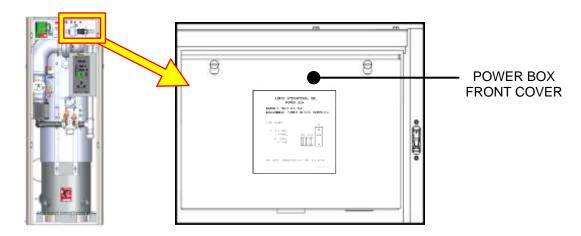
Figure 2-9b: BMK 1500/2000/2500/3000 Power Box with Closed Cover
