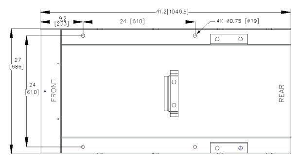
Figure 2-2b: BMK 1500/2000 Anchor Bolt Locations
