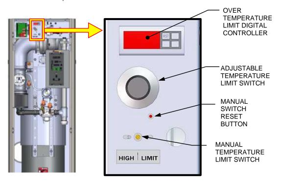
Figure 5-5a: Temperature Limit Switch Location – BMK 1500-3000
