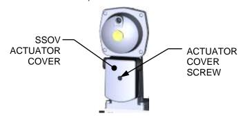
Figure 5-8: SSOV Actuator Cover Location
