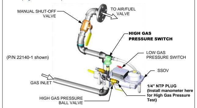
Figure 5–3a: BMK 750/1000 HIGH Gas Pressure Test Components
