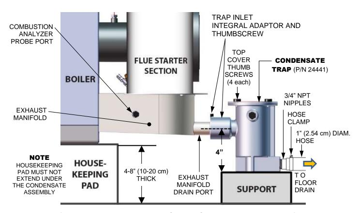
Figure 2-6b: BMK 1500 - 3000 Sample Condensate Trap Installation
