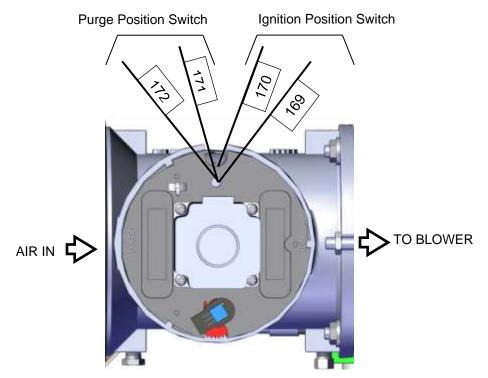
Figure 5-10b: Air/Fuel Purge and Ignition Locations— BMK 750/1000
