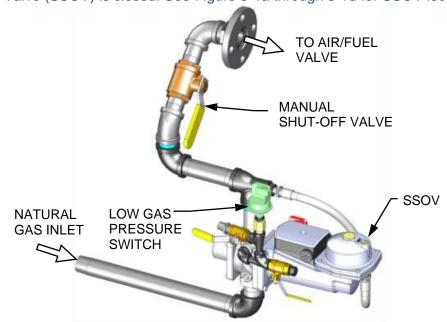
Figure 3-1a: BMK 750 & 1000 SSOV Location (P/N 22140-1 shown)
