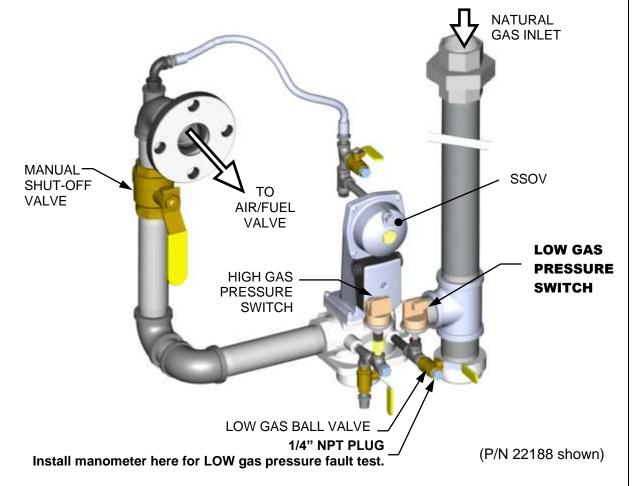
Figure 5-1b: <u>BMK 1500/2000</u> LOW Gas Pressure Test Components
