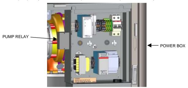
Figure 2-13a: BMK 750/1000 Pump Relay Location
