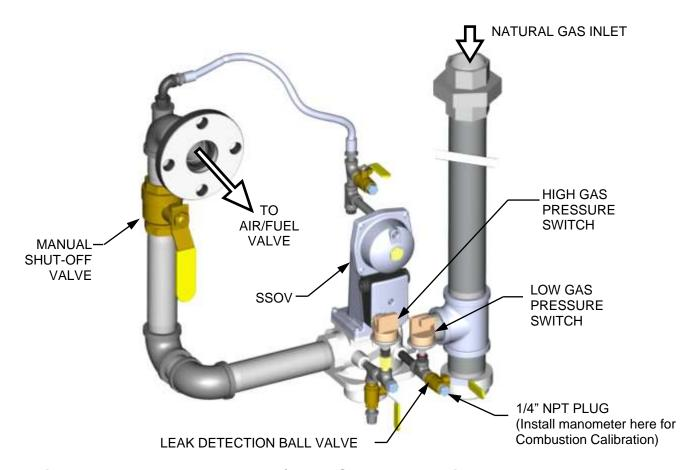
Figure 4-1b: BMK 1500 & 2000 1/4 Inch Gas Plug Location (P/N 22188 shown)
