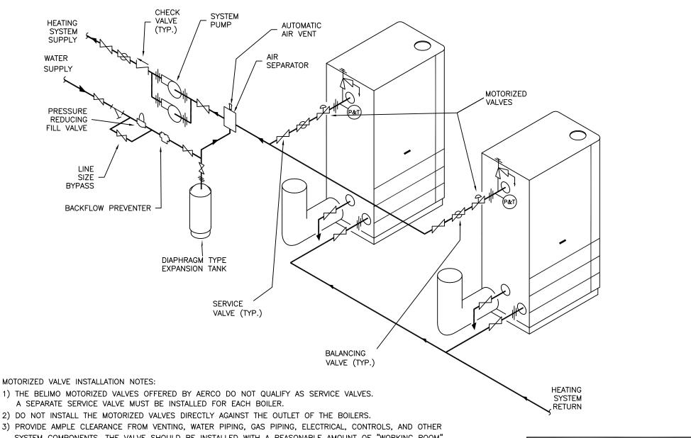
3) PROVIDE AMPLE CLEARANCE FROM VENTING, WATER PIPING, GAS PIPING, ELECTRICAL, CONTROLS, AND OTHER SYSTEM COMPONENTS. THE VALVE SHOULD BE INSTALLED WITH A REASONABLE AMOUNT OF "WORKING ROOM" AROUND IT TO ALLOW ROOM TO BE ABLE TO SERVICE THE VALVE AND USE THE MANUAL LEVER.
