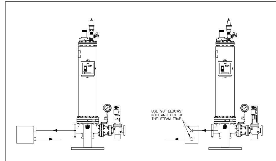
A PARALLEL PIPE STEAM TRAP CAN BE ORIENTED USING ONE OF THE ABOVE DIAGRAMS.
