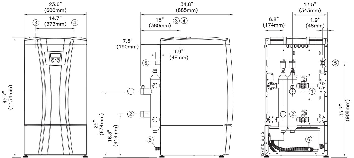
Figure 6-6 Dimensions for models 199, 250, 399 and 500.
