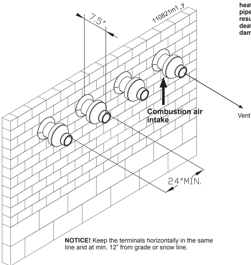
Figure 12-21 Concentric sidewall multiple heaters terminations
