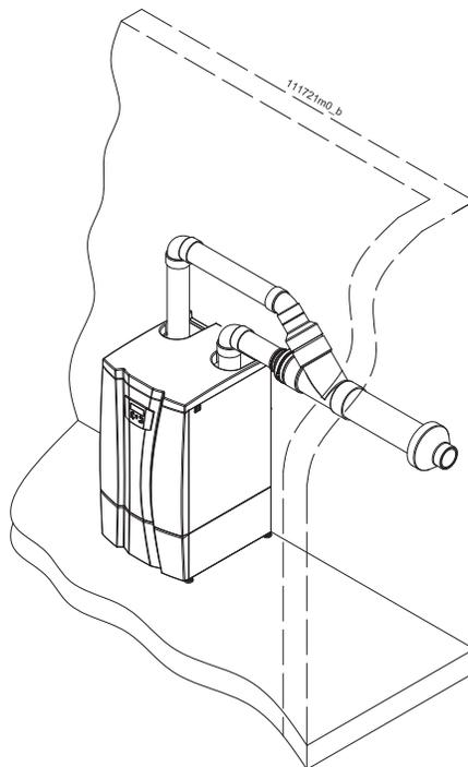
**Figure 12-5 Side wall concentric (Direct venting).**
