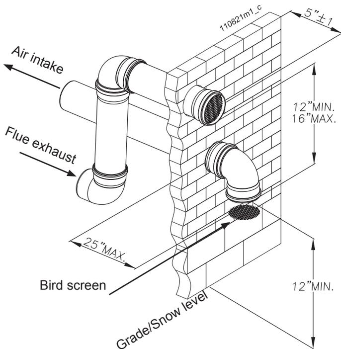
**Figure 12-16 Two pipes sidewall termination of air and vent (if space permits)**
