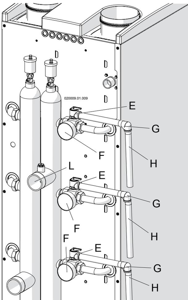
Figure 8-1 Piping of the P-T relief valve discharge
