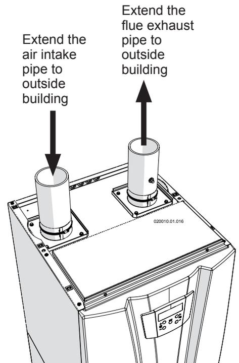
**Figure 12-11 Stainless steel air intake/vent connection**
