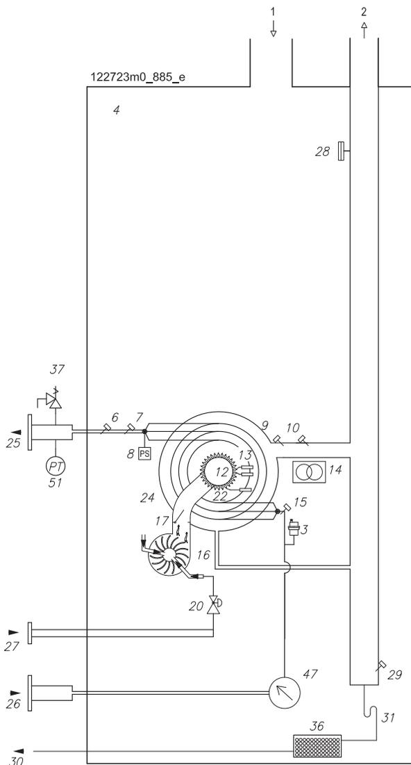
Figure 4-1 - Hydronic functional schematic for models 199 and 250
