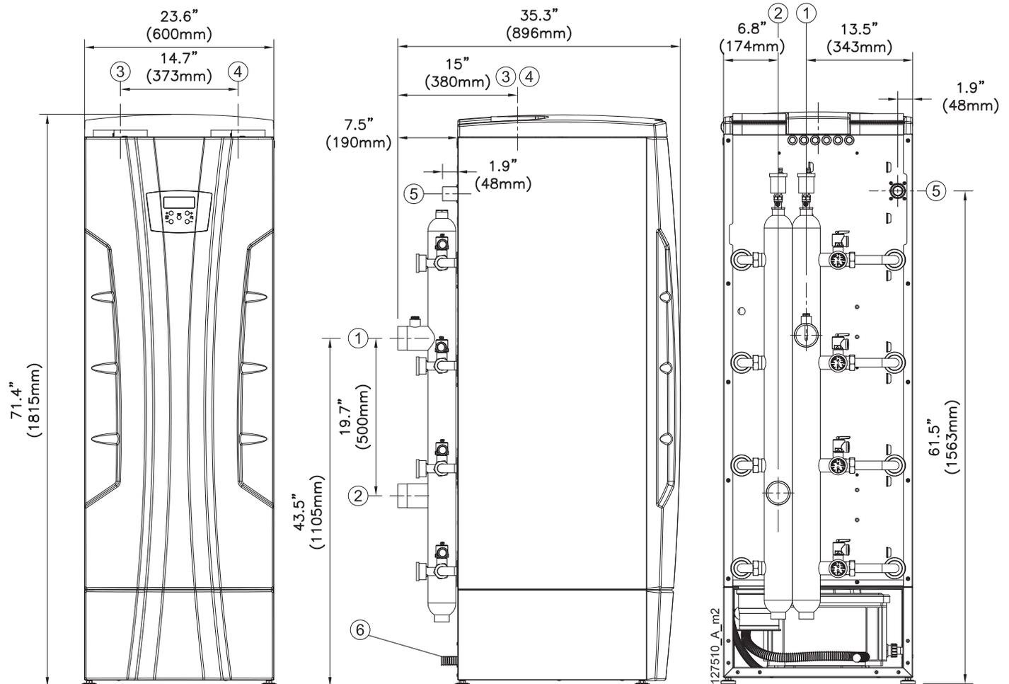
Figure 6-7 Dimensions for models 750 and 1000
