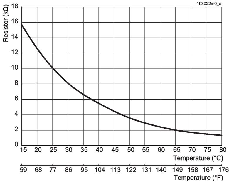
Figure 17-15 Water and flue temperature sensors' curve
