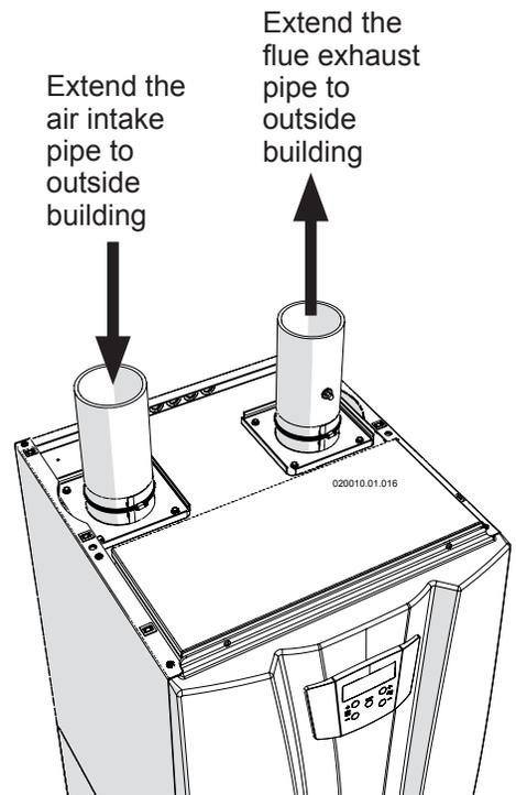
Figure 12-10 PVC/CPVC air intake/Vent connection correctly in place
